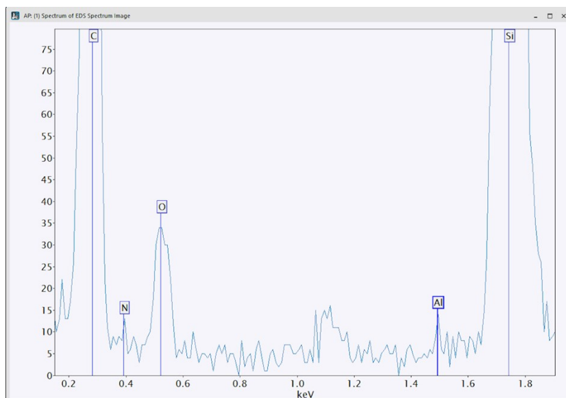
Figure S1. EDS spectrum acquired from the intercalated structure with sub-layers of Al atoms at the graphene/SiC interface at 60 KeV of beam energy and 0.01 KeV of energy dispersion. The main elements C, N, O, Al, and Si are here labeled.
