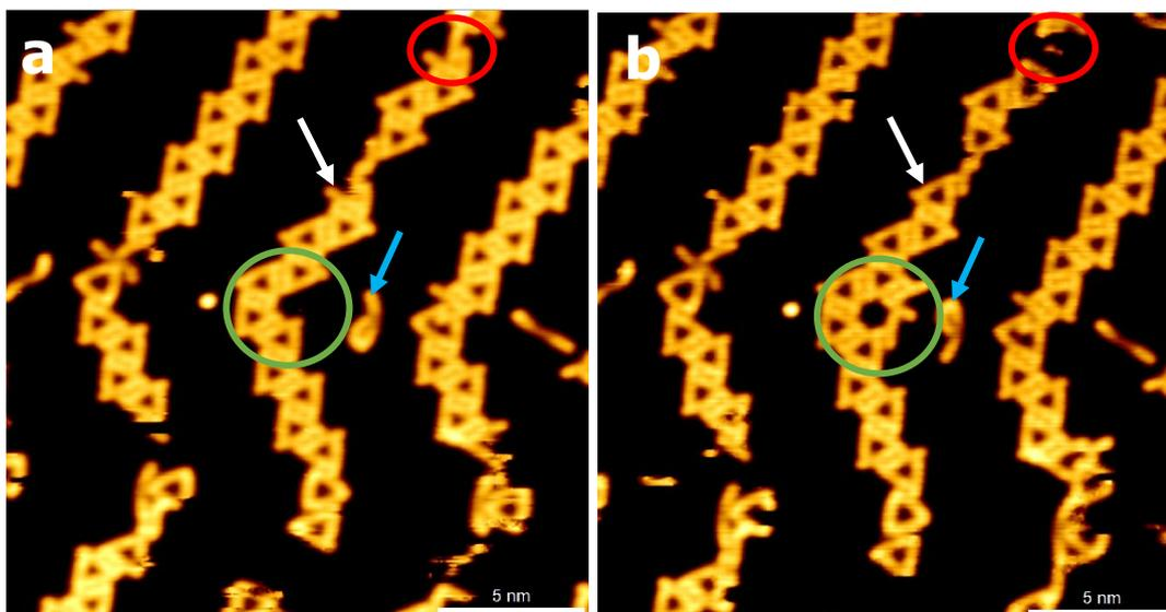
**Figure S1.** Two sequences of images for the triangle self-assembled pattern of DBTT showing the tip disturbance could move the triangles easily. (Scan area:  $100 \times 100 \text{ nm}^2$ ;  $V_s = -1000 \text{ mV}$ ,  $I = 100 \text{ pA}$ ).
