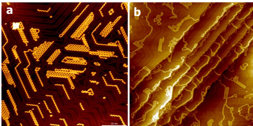
**Figure S9.** (a) Large-scale STM image of the organometallic intermediate of DBTT showing the single lines located on the Au(111) surface. ( $V_s = -600$  mV,  $I = 60$  pA). (b) Large-scale STM image of the complete polymer of DBTT showing the ordered and disorder polymer chains on the Au(111) surface. Scan area:  $100 \times 100$  nm<sup>2</sup>;  $V_s = 500$  mV,  $I = 200$  pA.
