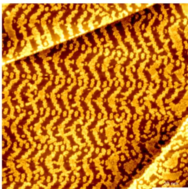
**Figure S7.** Large-scale STM image showing the molecular self-assembly after deposition of DBTT-CH<sub>3</sub> on the Au(111) surface at room temperature with ~0.6 monolayer. ( $V_s = 1000$  mV,  $I = 70$  pA).
