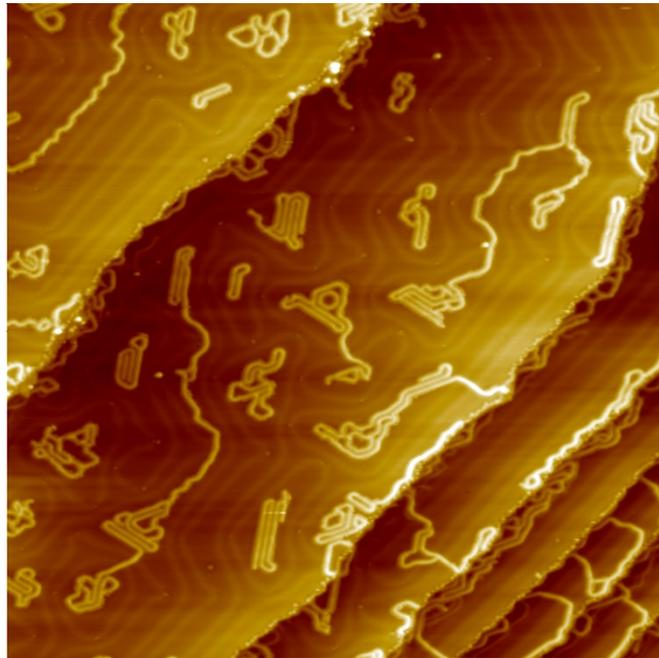
**Figure S3.** Large-scale STM image showing the formation of polythiophene. Almost no Br atoms adsorb on the Au(111) surface. The herringbone reconstruction of Au(111) is distorted at the place where the polythiophene coils are formed. Heating the sample for 40 min from the room temperature to 190°C. (Scan area: 66×66 nm<sup>2</sup>,  $V_s = -800$  mV,  $I = 80$  pA)
