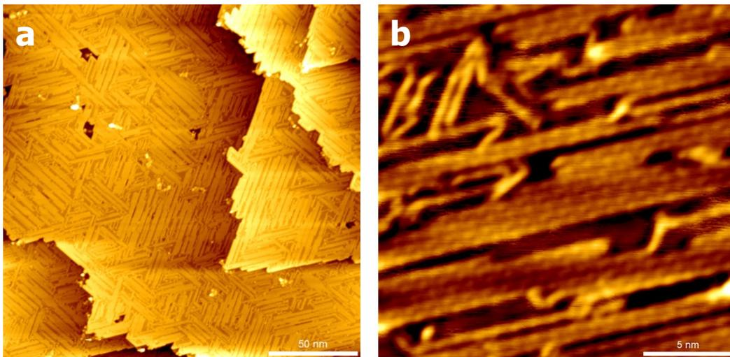
**Figure S5.** Large-scale (a) and high-resolution (b) STM images taken after deposition of 0.8 monolayer DBTT onto Cu(111) held at room temperature, showing the formation of the organometallic coordination. ( $V_s = -400 \text{ mV}$ ,  $I = 300 \text{ pA}$ ).
