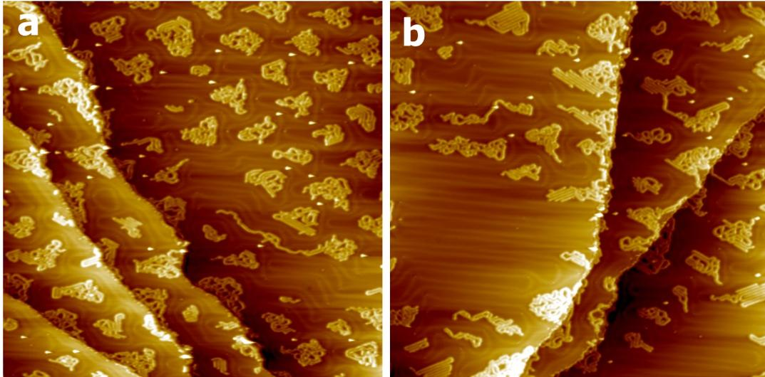
**Figure S4.** Large-scale STM images showing the morphology change of polythiophene coils from relative disordered (a) to less ordered coils (b) after annealing at 295°C for 5 min. (a) Scan area:  $100 \times 100 \text{ nm}^2$ ;  $V_s = 600 \text{ mV}$ ,  $I = 200 \text{ pA}$ . (b) Scan area:  $95 \times 95 \text{ nm}^2$ ;  $V_s = 700 \text{ mV}$ ,  $I = 50 \text{ pA}$ .
