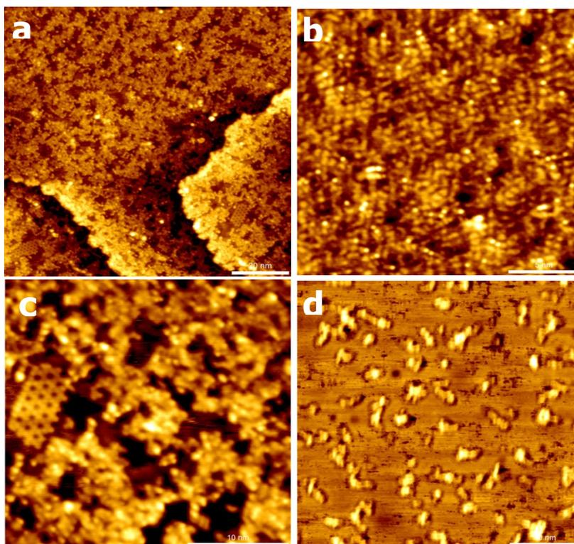
**Figure S6.** (a-c) STM images taken after annealing the coordinated intermediate of DBTT with 0.8 monolayer at 200 °C. ( $V_s = 600$  mV,  $I = 200$  pA). (d) STM image taken after annealing the coordinated intermediate of DBTT with 0.2 monolayer at 200 °C. ( $V_s = -500$  mV,  $I = 200$  pA).
