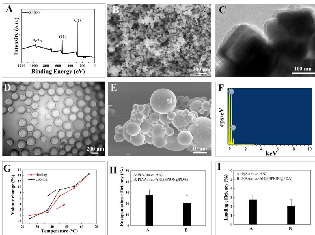
**Figure S1.** Characterization of microspheres. (A) XPS spectrum of SPION, (B) SEM and (C) TEM images of SPION@PDA. (D) Optical image, (E) SEM image, (F) SEM-EDS spectrum, and (G) volumetric alteration of P(AAm-co-AN) microspheres during heating/cooling procedure. (H) Drug encapsulation efficiency and (I) drug loading efficiency of microspheres.
