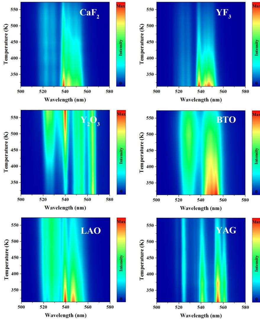
Fig. S4. The contour projections of thermal evolution spectra in 313–573 K range of  $\text{Er}^{3+}/\text{Yb}^{3+}$  co-doped  $\text{CaF}_2$ ,  $\text{YF}_3$ ,  $\text{Y}_2\text{O}_3$ , BTO, LAO and YAG samples.
