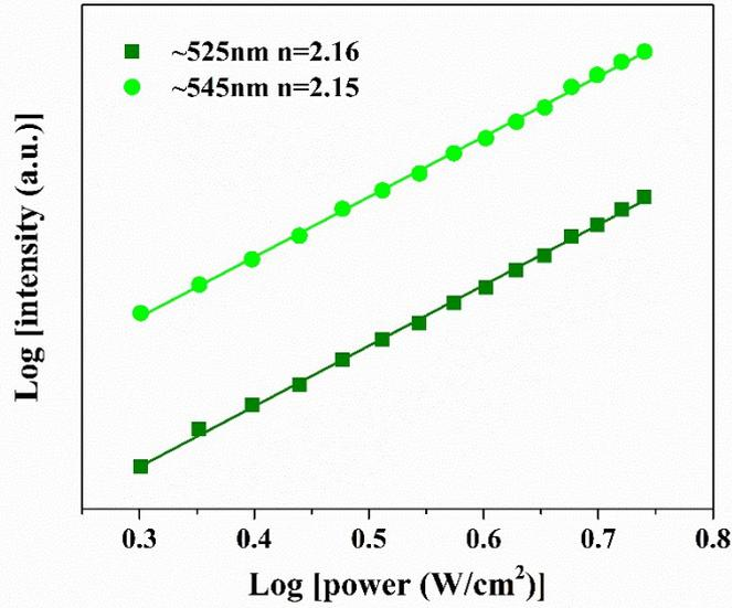
Fig. S2. The power-dependent slope factors ( $n$ ,  $I \sim P^n$ ) for the  $\sim 525$  nm and  $\sim 545$  nm emissions of  $\text{NaYF}_4: 2\% \text{Er}^{3+}, 18\% \text{Yb}^{3+}$  nanoparticles.  $n$  is the required pump photons of corresponding transition, that is, the slope value in Figure S2.  $I$  denotes the corresponding emission intensity, and  $P$  represents the excitation power.
