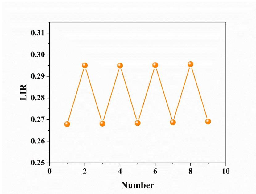
Fig. S10. The temperature-recycle measurements of *LIR* values of NaYF<sub>4</sub>: 2%Er<sup>3+</sup>, 18%Yb<sup>3+</sup>@NaYF<sub>4</sub>-PEI aqueous solution (500 μg/mL) under 980 nm excitation (2.0 W/cm<sup>2</sup>).
