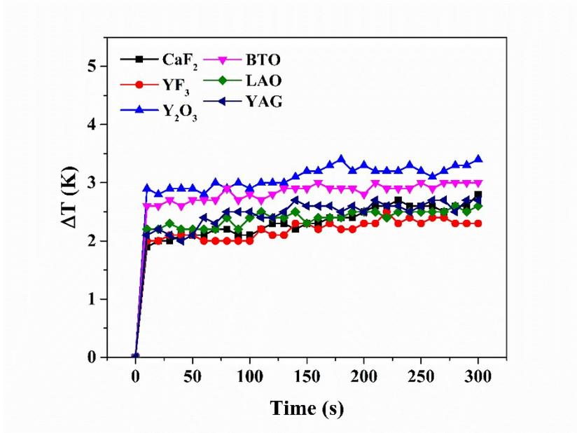
Fig. S7. The elevation of temperature of  $\text{Er}^{3+}/\text{Yb}^{3+}$  co-doped  $\text{CaF}_2$ ,  $\text{YF}_3$ ,  $\text{Y}_2\text{O}_3$ , BTO, LAO and YAG samples under 980 nm excitation with  $2.5 \text{ W/cm}^2$ .
