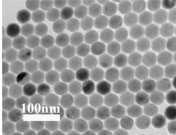
Fig. S8. The TEM image of  $\text{NaYF}_4: 2\%\text{Er}^{3+}, 18\%\text{Yb}^{3+}@ \text{NaYF}_4$  nanoparticles.
