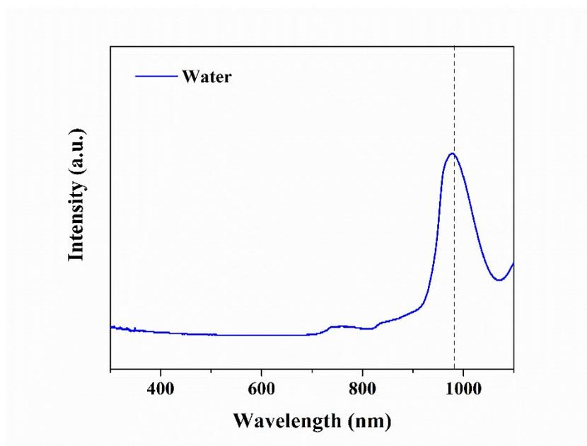
Fig. S11. Overlapping of the absorption spectrum of water and 980 nm excitation.
