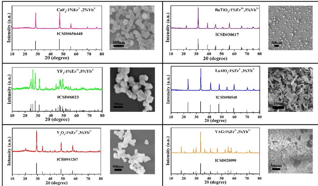
Fig. S3. The XRD patterns and SEM micrographs of  $\text{Er}^{3+}/\text{Yb}^{3+}$  co-doped  $\text{CaF}_2$ ,  $\text{YF}_3$ ,  $\text{Y}_2\text{O}_3$ , BTO, LAO and YAG samples.
