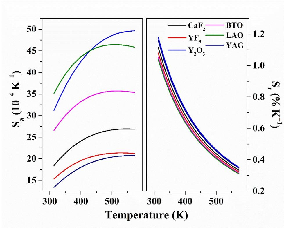
Fig. S6. The  $S_a$  and  $S_r$  of  $\text{Er}^{3+}/\text{Yb}^{3+}$  co-doped  $\text{CaF}_2$ ,  $\text{YF}_3$ ,  $\text{Y}_2\text{O}_3$ , BTO, LAO and YAG samples.
