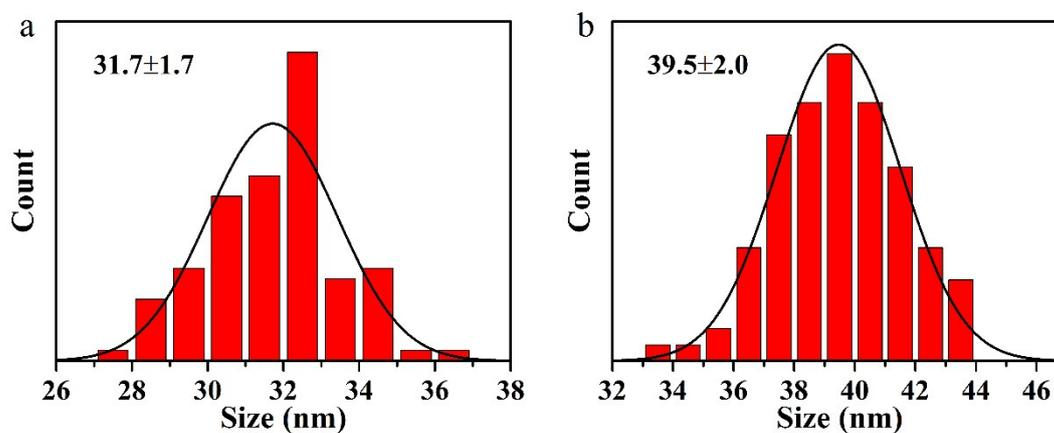
Fig. S1. The TEM-based size distribution histograms of (a) NaYF<sub>4</sub>: 2%Er<sup>3+</sup>, 18%Yb<sup>3+</sup> and (b) NaYF<sub>4</sub>: 2%Er<sup>3+</sup>, 18%Yb<sup>3+</sup>@NaYF<sub>4</sub> nanoparticles.
