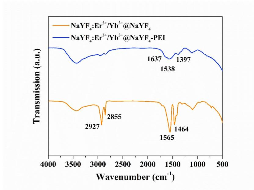
Fig. S9. The FT-IR spectra of OA-capped and PEI-capped  $\text{NaYF}_4: 2\%\text{Er}^{3+}, 18\%\text{Yb}^{3+}@ \text{NaYF}_4$  nanoparticles.
