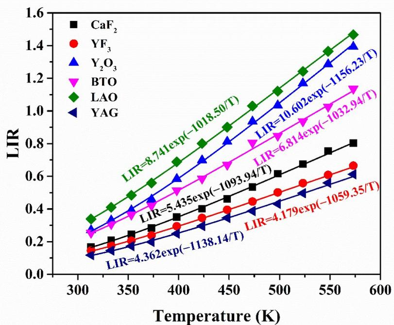
Fig. S5. The calculated calibration curves of Er<sup>3+</sup>/Yb<sup>3+</sup> co-doped CaF<sub>2</sub>, YF<sub>3</sub>, Y<sub>2</sub>O<sub>3</sub>, BTO, LAO and YAG samples.
