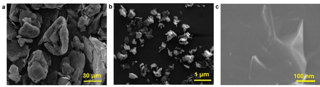
**Figure S5.** SEM images of natural ground mica (a) and mica nanosheets as-obtained (b, c), respectively. By comparing Fig. S1a to Fig.S1 b and c, the lateral size of MNSs are smaller than that of ground mica, revealing the ground has been successfully peeled through the proposed gas-assisted ball-milling strategy.
