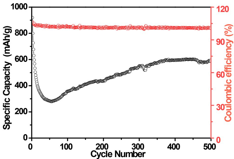
Figure S8 The cycling performances of MnO@C anode at 500 mA g<sup>-1</sup> current density.
