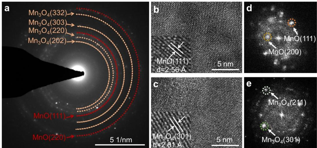
Figure S10 SAED patterns and HRTEM images of anodes after 200 cycles. (a) SAED patterns of MnO anode after 200 cycles. (b c), HRTEM images of anodes after 200 cycles. (d e) the corresponding FFT patterns of HRTEM images in b and c, respectively.
