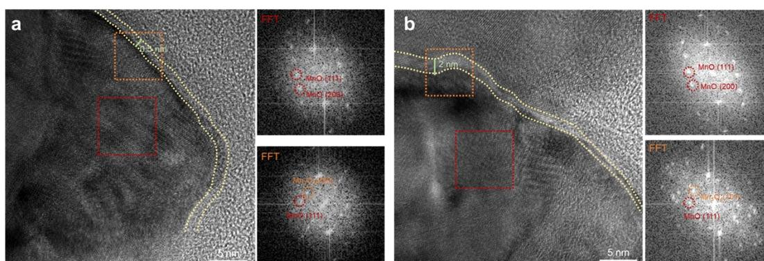
Figure S5 (a) HRTEM image of MnO anode discharged to 0.2 V and the corresponding FFT patterns of different regions. (b) HRTEM image of MnO anode discharged to 0.01 V and the corresponding FFT patterns of different regions.
