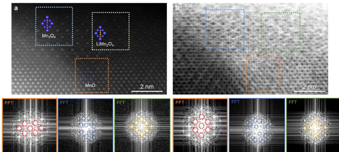
Figure S4 HAADF and ABF images of MnO anode discharged to 0.2 V. (a) HAADF image and the corresponding FFT patterns. (b) ABF image and the corresponding FFT patterns.
