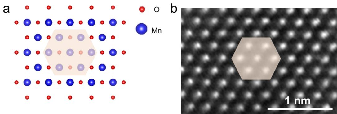
Figure S2 MnO@C anodes crystal structure and HAADF images along the [101] crystallographic. (a) Atomic structural model of MnO@C sample. (b) HAADF image of the MnO@C sample. The blue spheres represent Mn atoms, red spheres represent O atoms.
