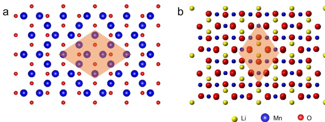
Figure S3 (a) Atomic structural model of the surface Mn<sub>3</sub>O<sub>4</sub> along the [100] crystallographic. (b) Atomic structural model of the surface LiMn<sub>2</sub>O<sub>4</sub> along the [110] crystallographic. The blue spheres represent Mn atoms, red spheres represent O atoms, and yellow spheres represent Li atoms, respectively.
