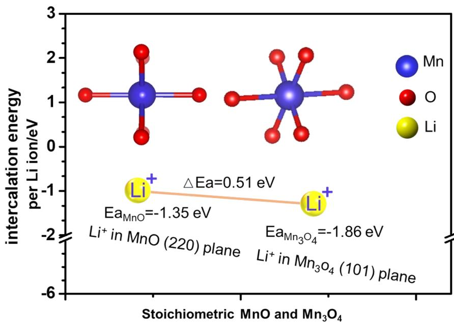
Figure S7 Schematic diagram of Li-ion adsorption energy in MnO<sub>(220)</sub> plane and in Mn<sub>3</sub>O<sub>4(101)</sub> plane.
