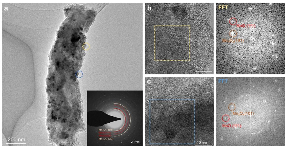
Figure S12 (a) Low magnification morphology image and SAED pattern of MnO anode after 500 cycles, (b) HRTEM image obtained from the area of the yellow box and the corresponding to FFT pattern, (c) HRTEM image obtained from the area of the blue box and the corresponding to FFT pattern.
