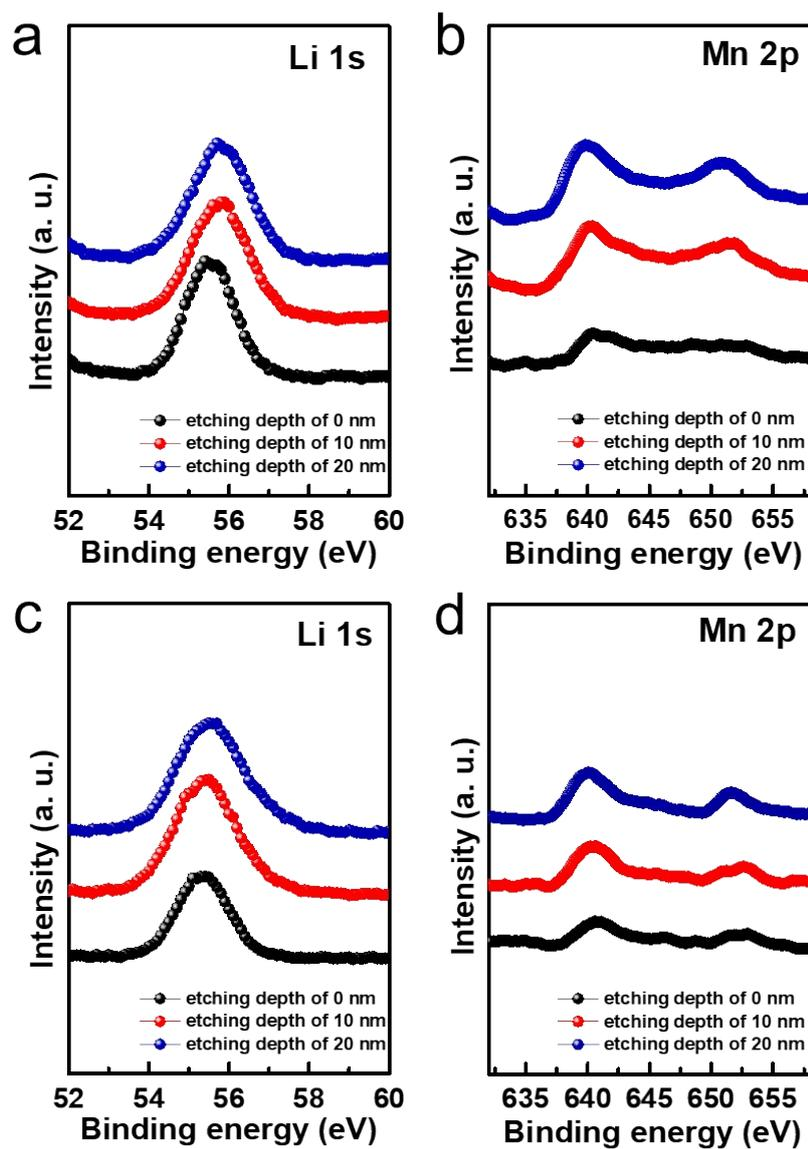
Figure S6 XPS spectra for etching different depth of Li 1s and Mn 2p. (a, b) show Li 1s and Mn 2p of etching depth of 0 nm, 10 nm and 20 nm for MnO anode discharged to 0.2 V. (c, d) show Li 1s and Mn 2p of etching depth of 0 nm, 10 nm and 20 nm for MnO anode discharged to 0.01 V.
