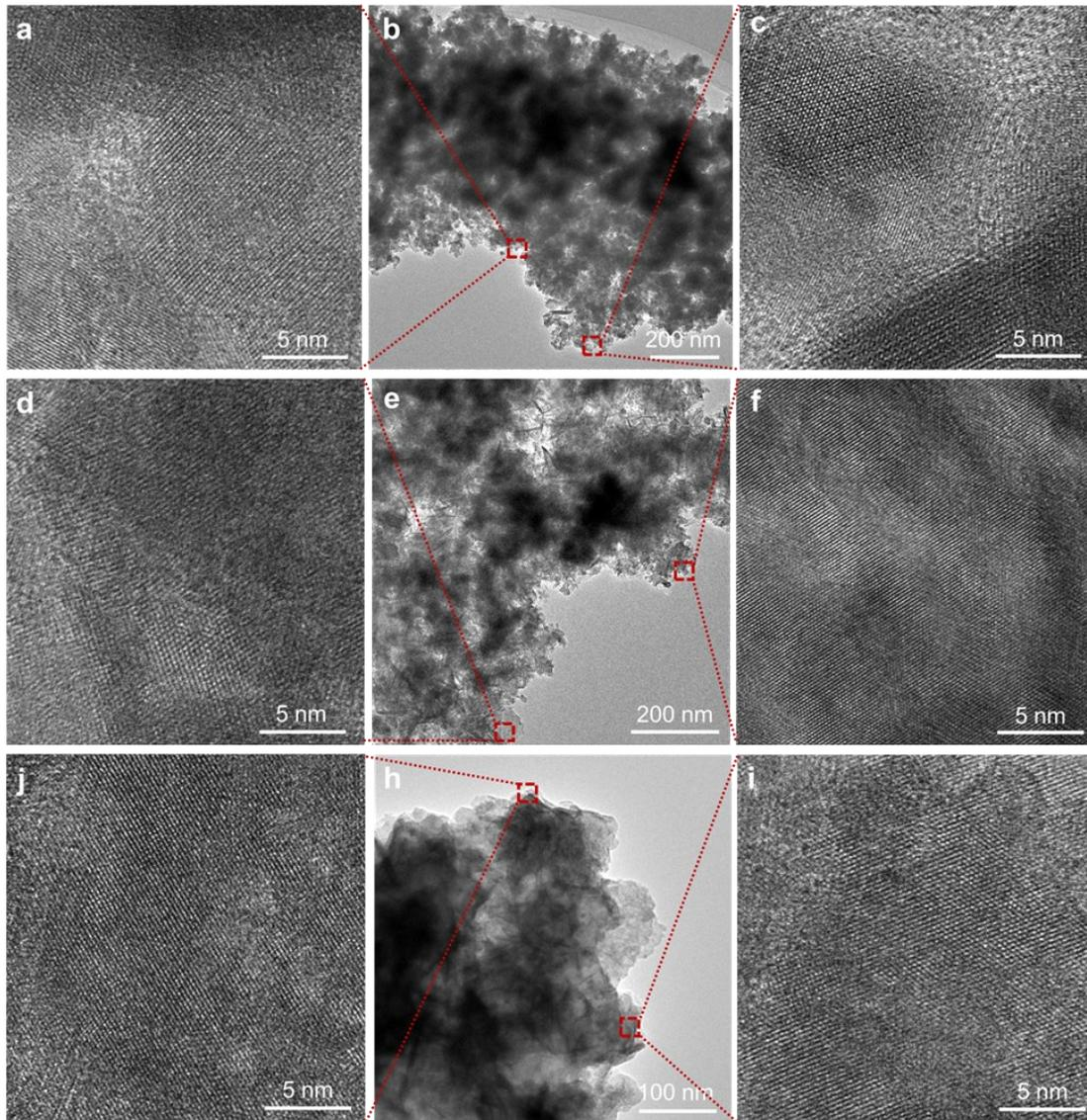
Figure S11 b, e and h, Low magnification images and HRTEM images of anodes after 50, 100 and 200 cycles. (a d j), HRTEM images of MnO. (c) HRTEM image of MnO<sub>2</sub>. (f i) HRTEM images of Mn<sub>3</sub>O<sub>4</sub>.
