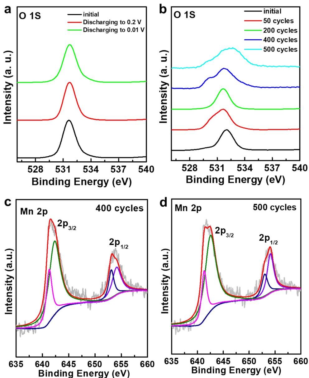
Fig.S9 (a) XPS spectra for initial MnO anode, discharged to 0.2 V and discharged to 0.01 V during the first cycle of O 1s, (b) XPS spectra for initial MnO anode, after 50 cycles, after 200 cycles, after 400 cycles and 500 cycles of O 1s, (c) XPS spectra of Mn 2p after 400 cycles. (d) XPS spectra of Mn 2p after 500 cycles.
