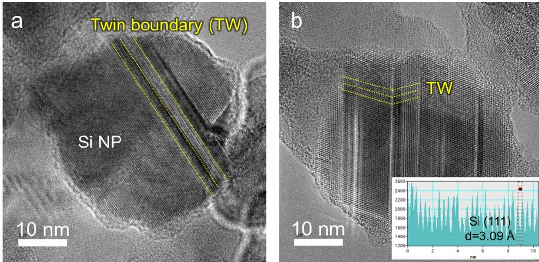
**Figure S3.** a, b) High-magnification transmission electron microscopy (TEM) images of bare Si nanoparticles (NPs). Lattice fringe pattern of Si NP in (b) shows a d-spacing value of 3.09 Å corresponding to the (111) plane of silicon.
