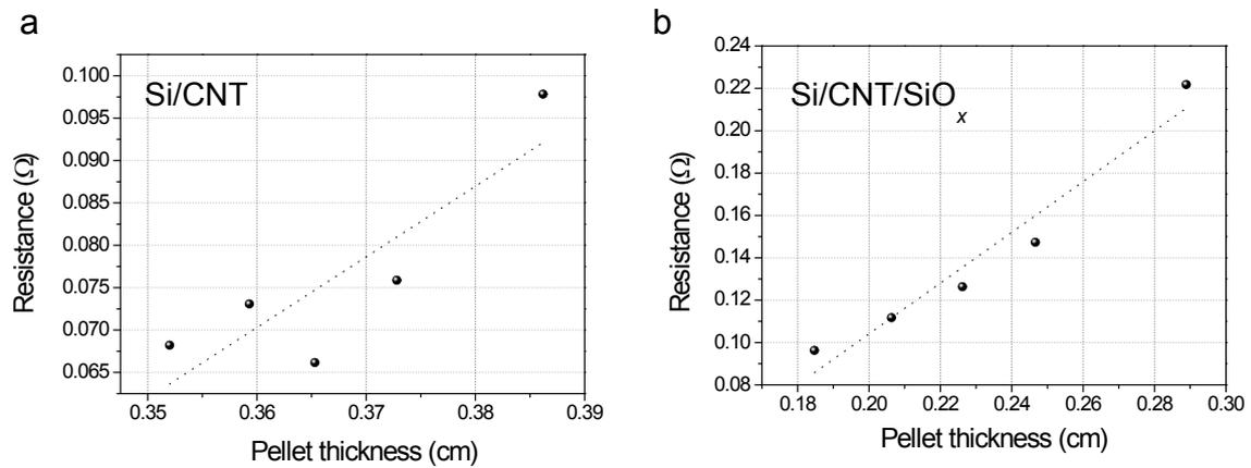
**Figure S4.** Resistance vs. pellet thickness for (a) Si/CNT and (b) Si/CNT/SiO<sub>x</sub> composites.
