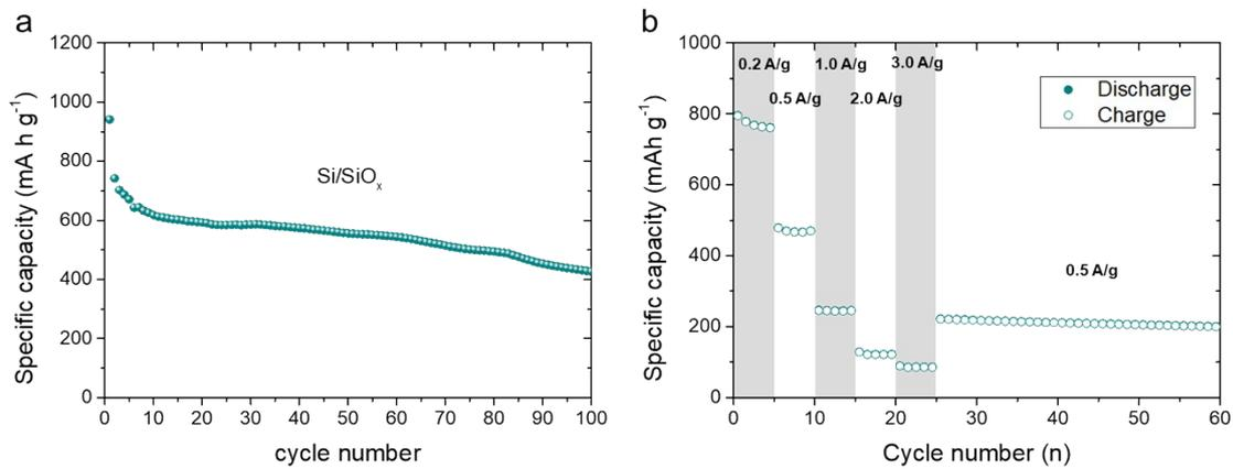
**Figure S5.** (a) Cycling performances of the Si /SiO<sub>x</sub> at a current density of 0.5 A g<sup>-1</sup>. (b) Rate performance of Si /SiO<sub>x</sub> with increasing current density. All the cycling and rate performance tests were conducted at the same charge–discharge rate.
