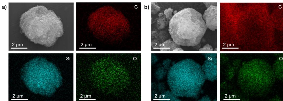
**Figure S1.** EDS maps of (a) the Si/CNT and (b) Si/CNT/SiO<sub>x</sub> microsphere composites. (red: C; blue: Si; and green: O)
