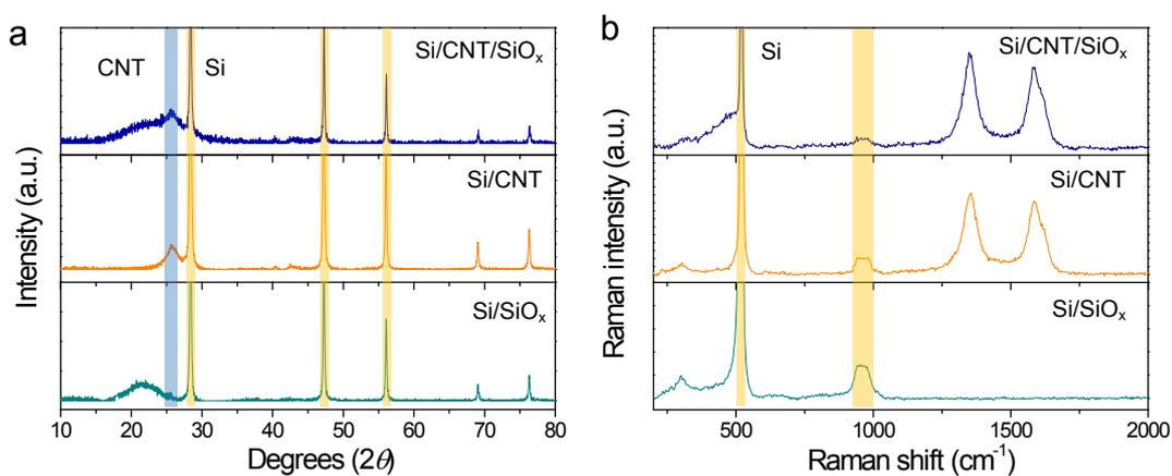
**Figure S2.** (a) X-ray diffraction (XRD) patterns and (b) Raman spectra of Si/CNT/SiO<sub>x</sub>, Si/CNT, and Si/SiO<sub>x</sub> composites.
