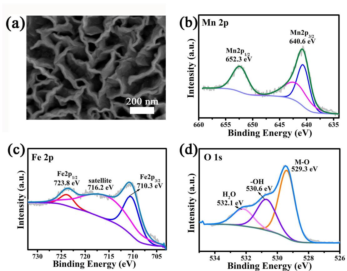
**Fig. S8.** (a) SEM image of MnFeO-NF-0.4 after stability test. (b–d) High resolution XPS spectra of Mn 2p, Fe 2p, and O 1s after stability test.
