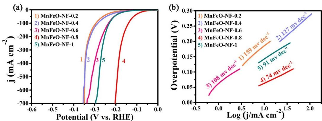
**Fig. S9.** (a) Polarization curves and (b) Tafel plots of MnFeO-NF-0.2, MnFeO-NF-0.4, MnFeO-NF-0.6, MnFeO-NF-0.8, and MnFeO-NF-1 in 1.0 M KOH.
