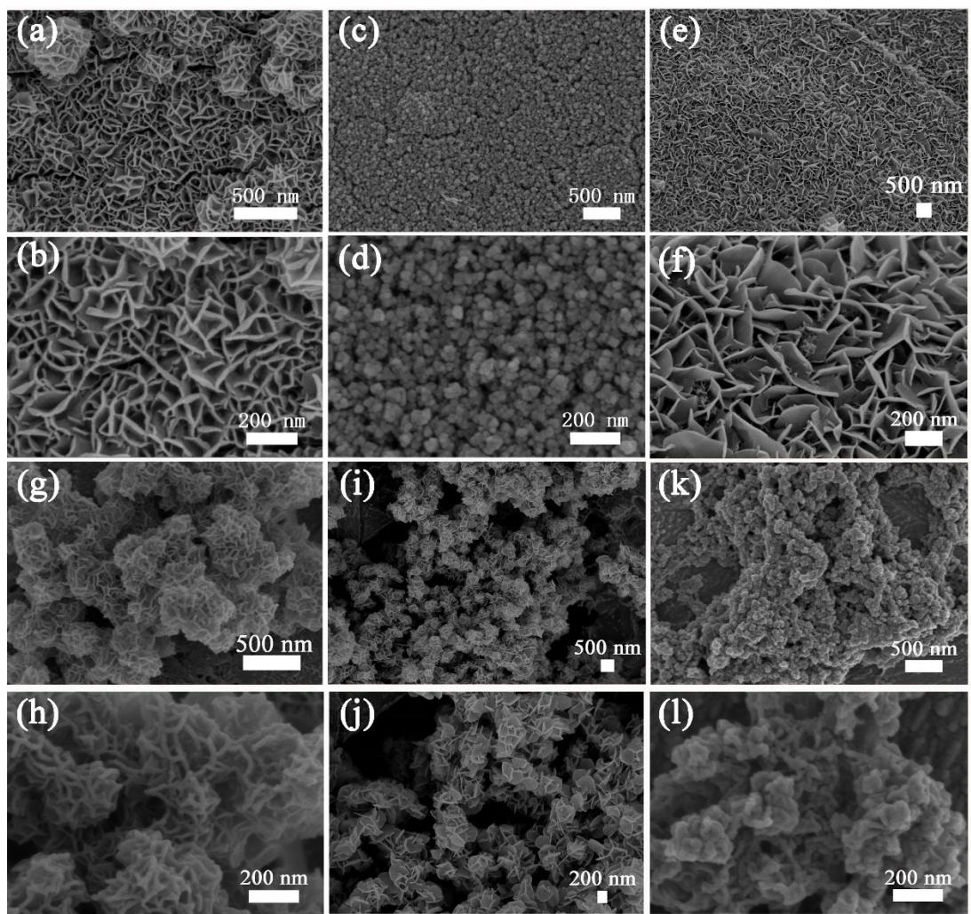
**Fig. S2.** SEM and magnified SEM images of MnO<sub>2</sub>-NF (a, b), MnFeO-NF-0.2 (c, d), MnFeO-NF-0.4 (e, f), MnFeO-NF-0.6 (g, h), MnFeO-NF-0.8 (i, j), and MnFeO-NF-1 (k, l), respectively.
