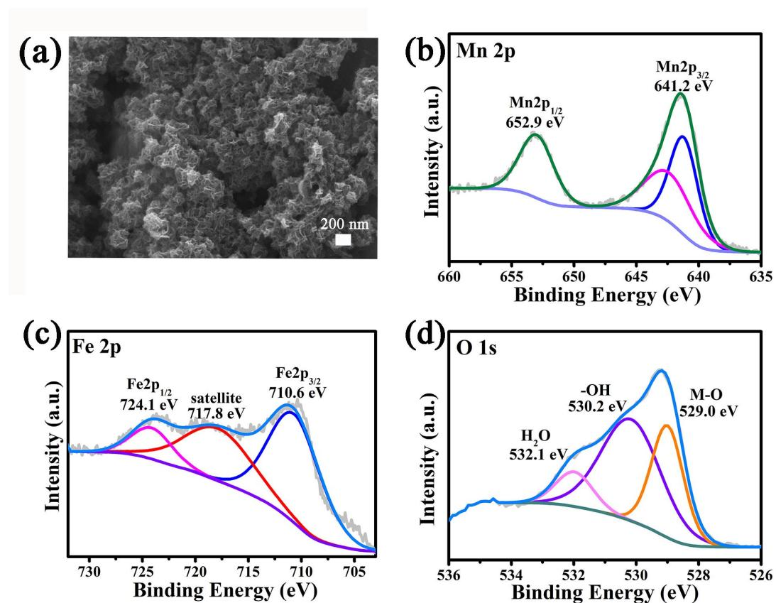
**Fig. S12.** (a) SEM image of MnFeO-NF-0.8 after stability test. (c-d) High resolution XPS spectra of Mn 2p, Fe 2p, and O 1s after stability test for MnFeO-NF-0.8.
