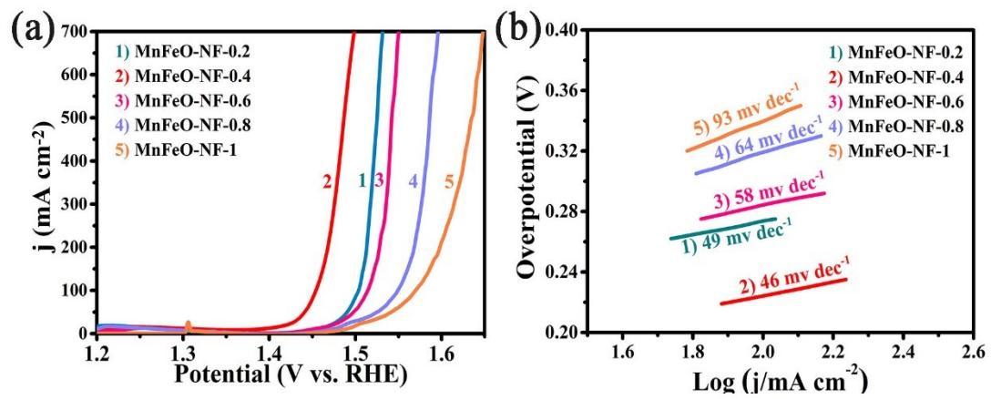
**Fig. S5.** (a) Polarization curves and (b) Tafel plots of MnFeO-NF-0.2, MnFeO-NF-0.4, MnFeO-NF-0.6, MnFeO-NF-0.8, and MnFeO-NF-1 in 1.0 M KOH.
