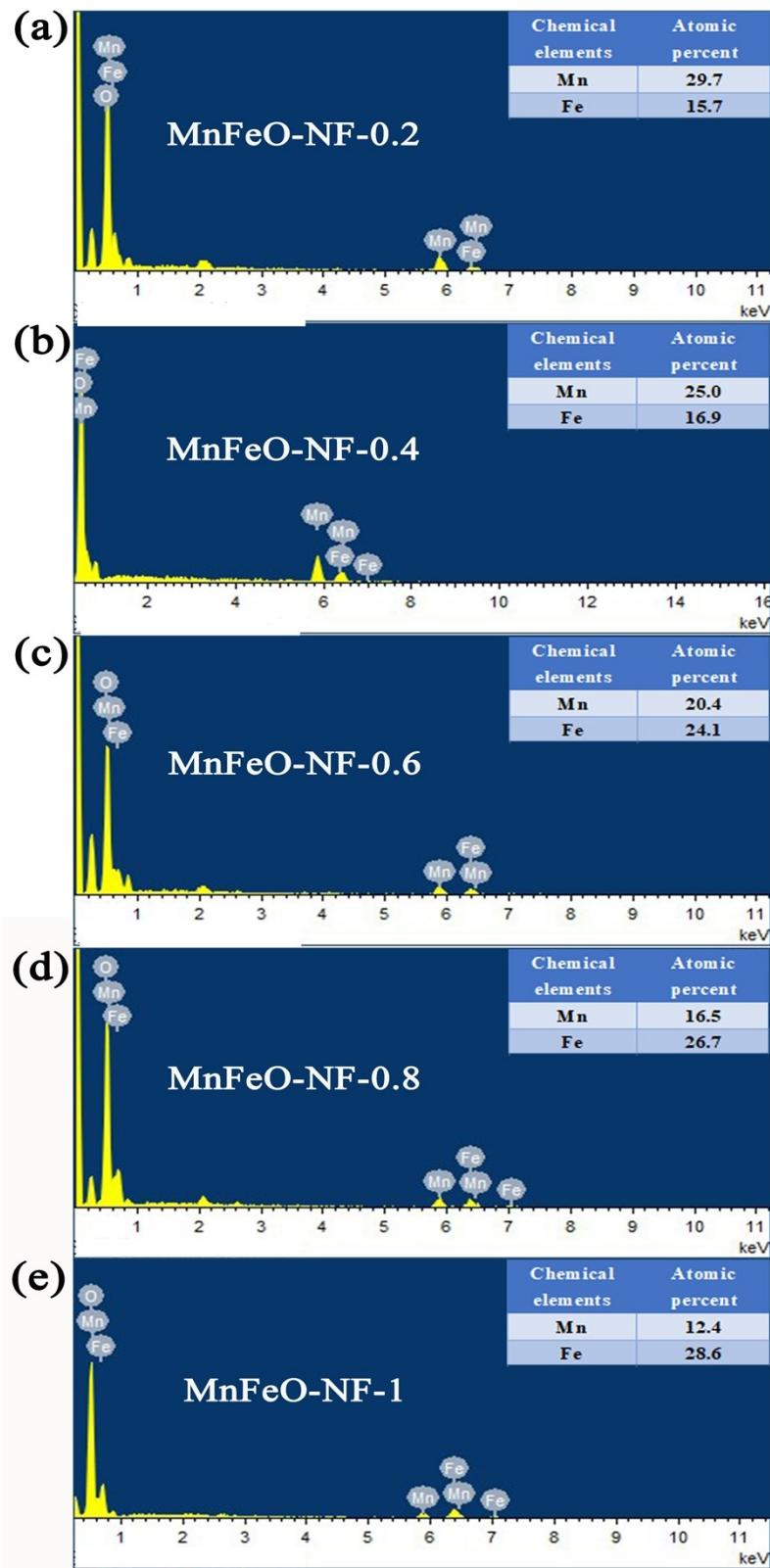
**Fig. S3.** EDS data of (a) MnFeO-NF-0.2, (b) MnFeO-NF-0.4, (c) MnFeO-NF-0.6, (d) MnFeO-NF-0.8, and (e) MnFeO-NF-1. Inset image is a table of atomic percent of Mn and Fe.
