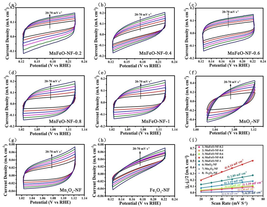
**Fig. S11.** CV curves at different scan rates for catalysts: (a) MnFeO-NF-0.2, (b) MnFeO-NF-0.4, (c) MnFeO-NF-0.6, (d) MnFeO-NF-0.8, (e) MnFeO-NF-1, (f) MnO<sub>2</sub>-NF, (g) Mn<sub>3</sub>O<sub>4</sub>-NF, and (h) Fe<sub>2</sub>O<sub>3</sub>-NF. (i) Plots of capacitive currents with different scan rates for various catalysts to determine  $C_{dl}$ .
