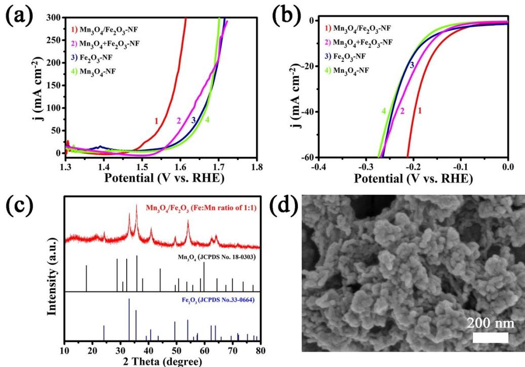
**Fig. S1.** (a) OER polarization curves and (b) HER polarization curves of  $\text{Mn}_3\text{O}_4/\text{Fe}_2\text{O}_3\text{-NF}$  complex,  $\text{Mn}_3\text{O}_4+\text{Fe}_2\text{O}_3\text{-NF}$  complex,  $\text{Fe}_2\text{O}_3\text{-NF}$ , and  $\text{Mn}_3\text{O}_4\text{-NF}$  in 1.0 M KOH. (c) XRD pattern and (d) SEM image of  $\text{Mn}_3\text{O}_4/\text{Fe}_2\text{O}_3$  (Fe:Mn ratio of 1:1).
