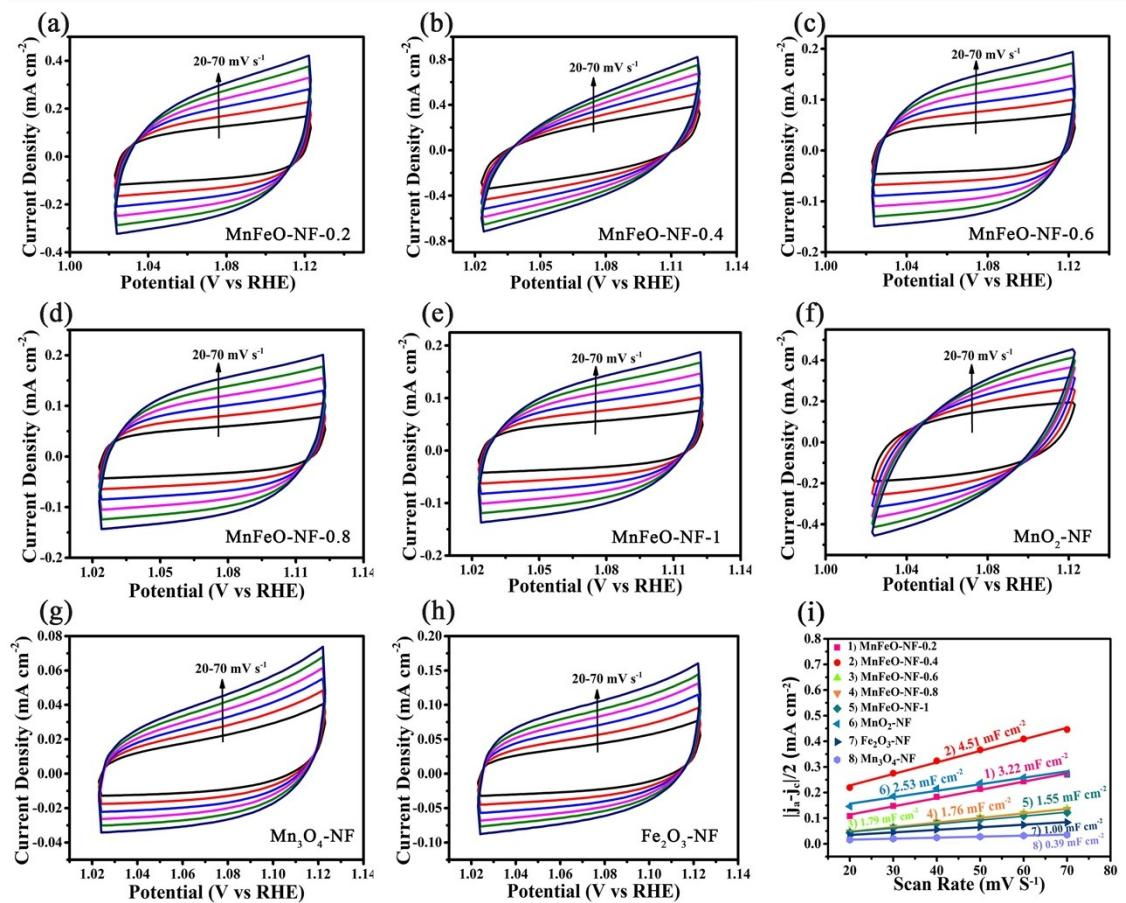
**Fig. S7.** CV curves at different scan rates for catalysts: (a) MnFeO-NF-0.2, (b) MnFeO-NF-0.4, (c) MnFeO-NF-0.6, (d) MnFeO-NF-0.8, (e) MnFeO-NF-1, (f) MnO<sub>2</sub>-NF, (g) Mn<sub>3</sub>O<sub>4</sub>-NF, and (h) Fe<sub>2</sub>O<sub>3</sub>-NF, (i) Plots of capacitive currents with different scan rates for various catalysts to determine C<sub>dl</sub>.
