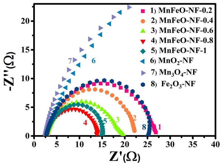
**Fig. S10.** EIS of MnFeO-NF-0.2, MnFeO-NF-0.4, MnFeO-NF-0.6, MnFeO-NF-0.8, MnFeO-NF-1, MnO<sub>2</sub>-NF, Mn<sub>3</sub>O<sub>4</sub>-NF, and Fe<sub>2</sub>O<sub>3</sub>-NF at -0.177 V vs. RHE.
