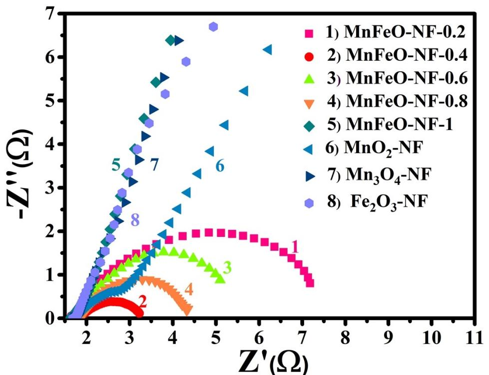
**Fig. S6.** EIS of MnFeO-NF-0.2, MnFeO-NF-0.4, MnFeO-NF-0.6, MnFeO-NF-0.8, MnFeO-NF-1, MnO<sub>2</sub>-NF, Mn<sub>3</sub>O<sub>4</sub>-NF, and Fe<sub>2</sub>O<sub>3</sub>-NF at 1.533 V *vs.* RHE.
