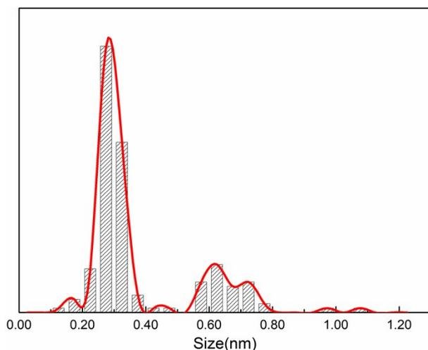
**Fig. S3. Histogram of cluster height distribution.** This plot is based on measurement from a sample that has been annealed to 425 K. The height distribution has two peaks: one at  $\sim 0.28$  nm due to  $C_{60}$  molecules sitting on a single layer of Au atoms; and the other at  $\sim 0.63$  nm which is due to  $C_{60}$  molecule sitting on two layers of Au.
