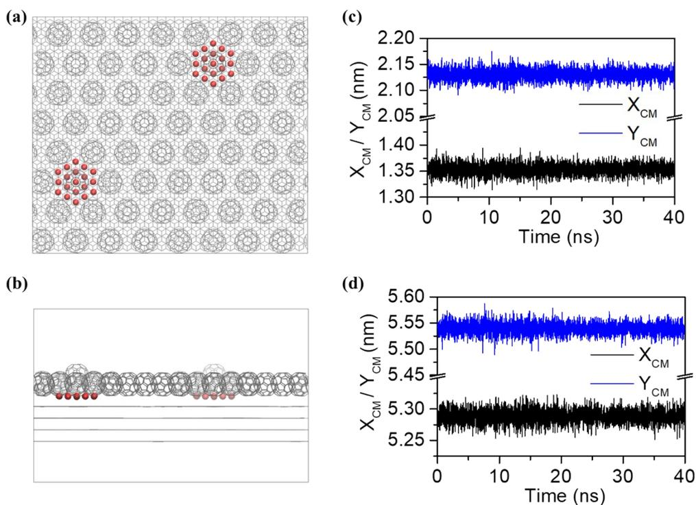
Figure S4. Molecular-dynamics simulation results at 300 K. (a) Top view and (b) side view of the atomic model in the MD calculations. (c, d) The evolution of the center-of-mass position as a function of the simulation time for the lower left and the upper right Au<sub>19</sub> clusters in (a), respectively.  $X_{CM}$  and  $Y_{CM}$  are the (x,y) coordinates of the center of mass of the cluster.
