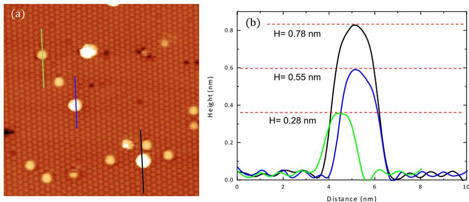
**Fig. S2 (a)** STM image obtained with +1.7 V sample bias and 50 pA tunnel current. **(b)** Height profiles along the green, blue, and black lines in (a), respectively. Height profile along the green line in (a) shows that the corresponding bright  $C_{60}$  is  $\sim 0.28$  nm tall. The height profiles along the blue line and the black line are for two floating Au clusters.
