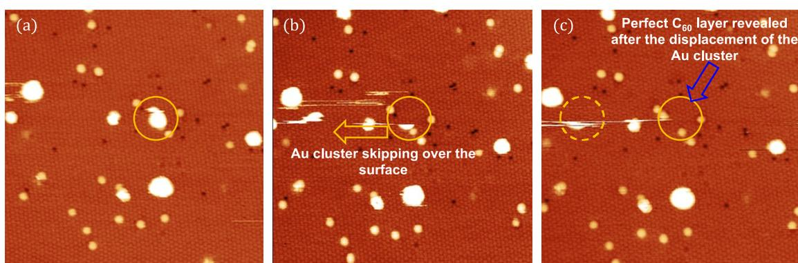
Fig. S1 Successive STM images showing the movement of a floating Au cluster. Image size: 55 nm x 55 nm. Image parameters: +1.7 V; 50 pA.
