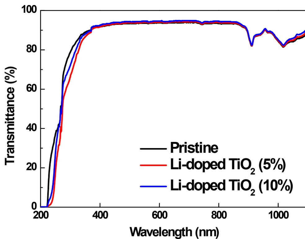
**Fig. S3** Optical transmittance from pristine, 5% and 10% Li-doped TiO<sub>2</sub> NPs.
