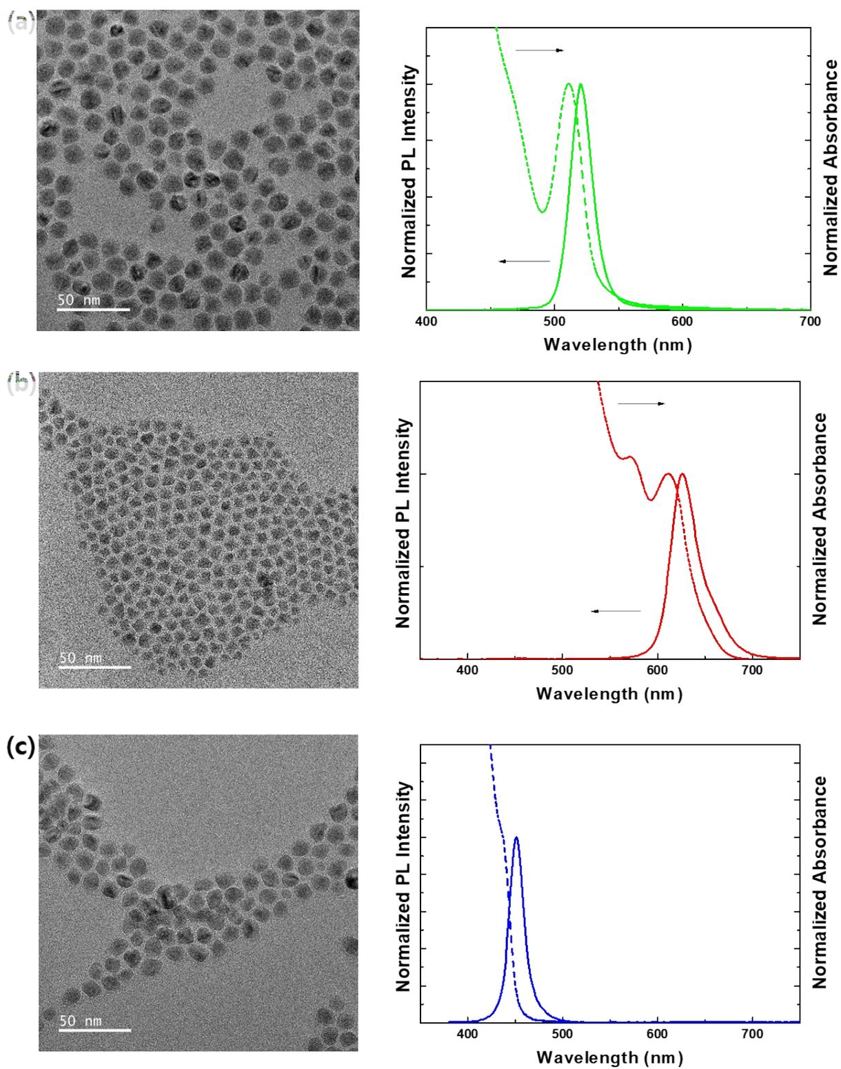
**Fig. S6** TEM images and absorption/PL spectra of (a) green, (b) red, and (c) blue QDs.
