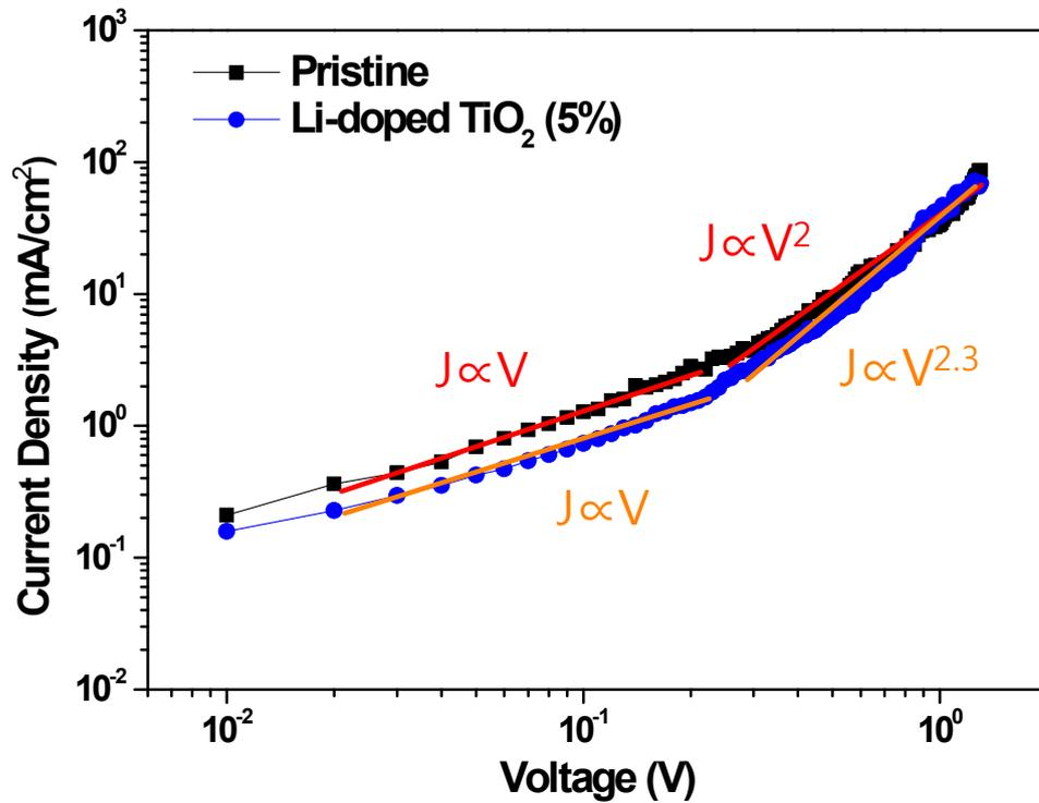
**Fig. S10** Current density-voltage curves of two comparative EODs based on pristine and 5% Li-doped TiO<sub>2</sub> NPs. EOD structure consists of ITO/Al/200 nm-thick pristine or 5% Li-doped TiO<sub>2</sub> NPs/Al. Electron mobilities were calculated by Child's law (inset) to be  $3.3 \times 10^{-6}$  and  $2.8 \times 10^{-6}$  cm<sup>2</sup>/Vs for pristine or 5% Li-doped TiO<sub>2</sub> NPs, respectively. Relative permittivity of TiO<sub>2</sub> was taken as 85 for this calculation.
