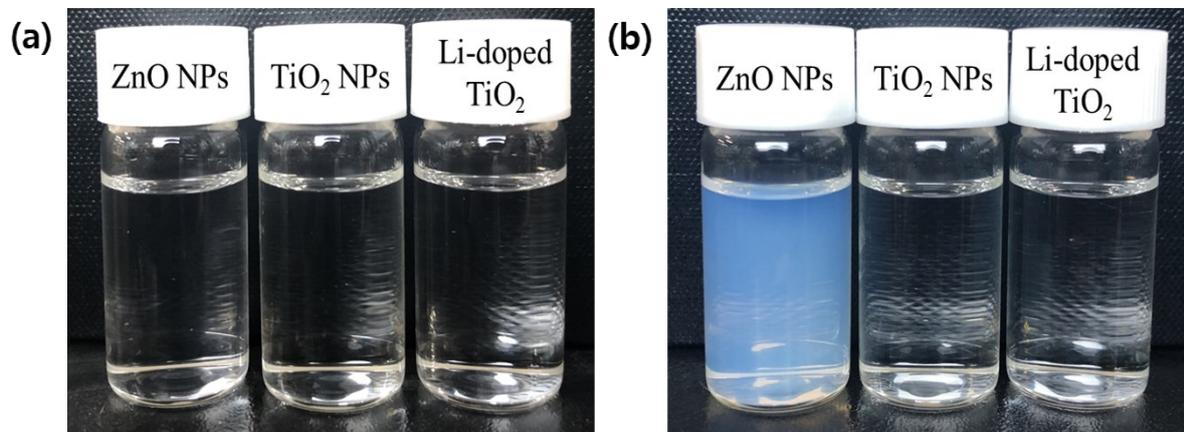
**Fig. S5** Observation of the aggregate formation from ZnO, TiO<sub>2</sub> and 5% Li-doped TiO<sub>2</sub> NPs in ethanol at room temperature: (a) As-re-dispersed and (b) after 2 days.
