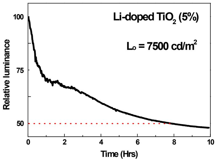
**Fig. S8** Lifetime measurement of QLEDs with 5% Li-doped  $\text{TiO}_2$  NPs as the ETL.
