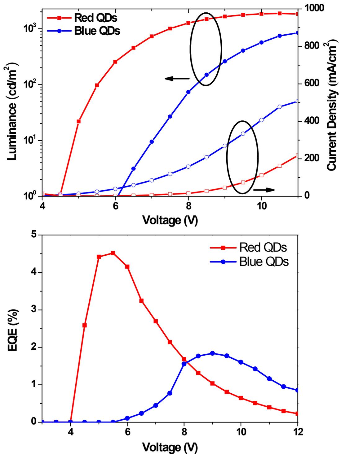
**Fig. S11** (a) Luminance-voltage-current density curves and (b) EQE-voltage curves of red and blue QLEDs with 5% Li-doped TiO<sub>2</sub> NPs.
