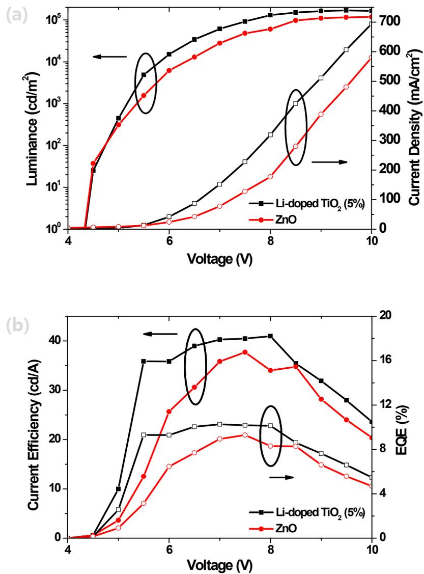
**Fig. S9** Voltage-dependent variations of (a) current density and luminance and (b) current efficiency and EQE of QLEDs with 5% Li-doped TiO<sub>2</sub> NPs or ZnO NPs as the ETL.
