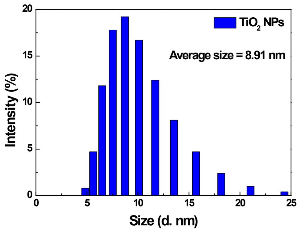
**Fig. S1** Particle size distribution of TiO<sub>2</sub> nanoparticles by dynamic light scattering method.
