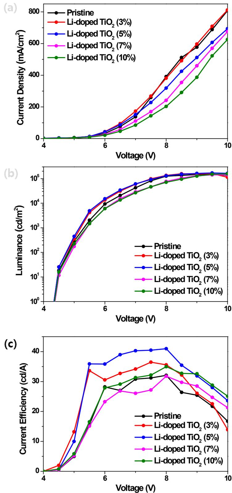
**Fig. S7** Voltage-dependent variations of (a) current density, (b) luminance, and (c) current efficiency of QLEDs with pristine or Li-doped TiO<sub>2</sub> NPs as the ETL.
