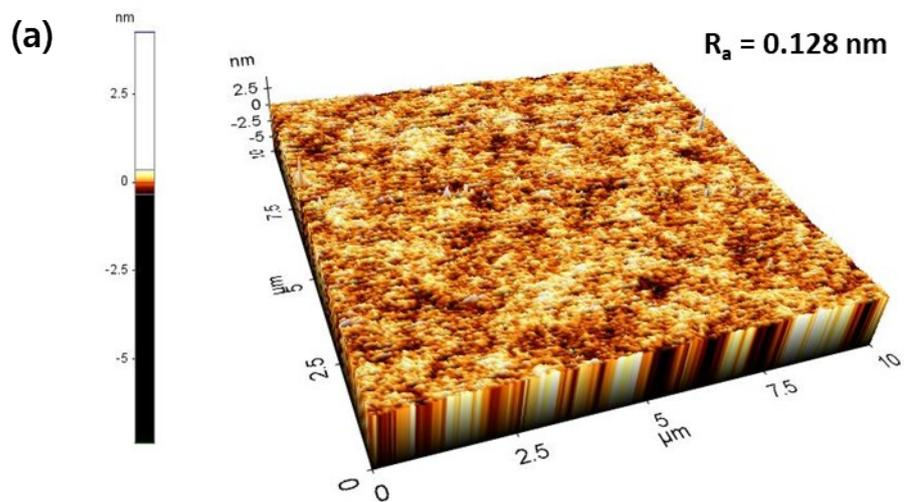
**Fig. S4** AFM images of (a) pristine and (b) 5% Li-doped  $\text{TiO}_2$  NPs on ITO glass.
