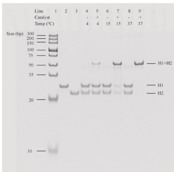
Figure S1. Native PAGE analysis of CHA at different temperatures. Line 1: ladder; Line 2: 500 nM H1 alone; Line 3: 500 nM H2 alone; Line 4, 6, 8: 500 nM H1 and 500 nM H2 at the respective temperatures for 30 min; Line 5, 7, 9: 500 nM H1, 500 nM H2 and 50 nM catalyst at the respective temperatures for 30 min.
