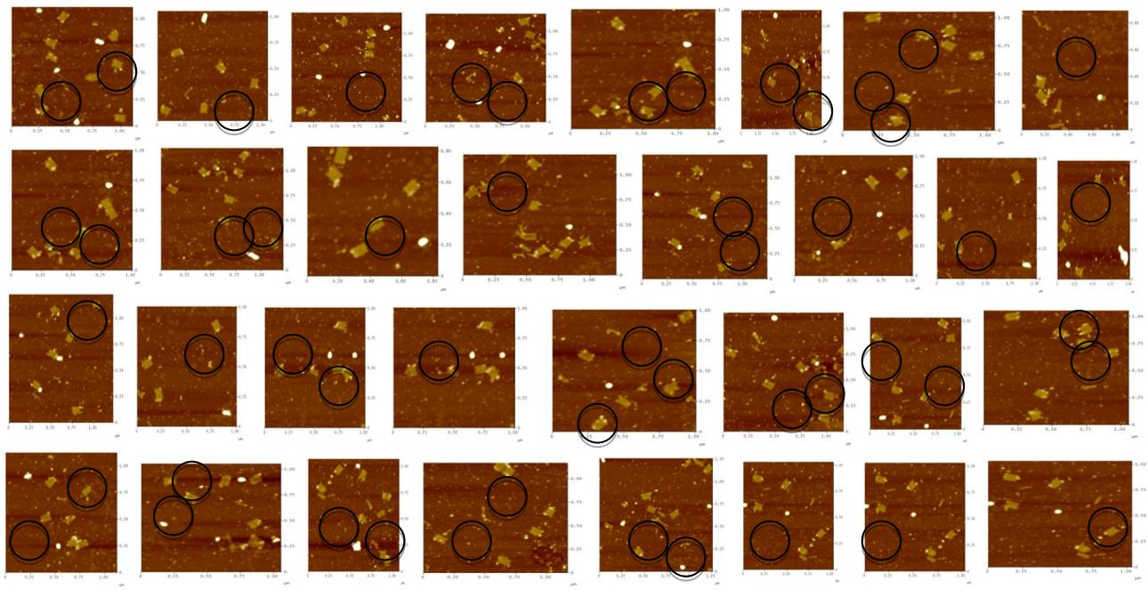
**Figure S5.** Representative AFM images for calculating the efficiency of modification as described in Table 1. Twin spots of 5 nm each or 10 nm high spots are marked with black circle.
