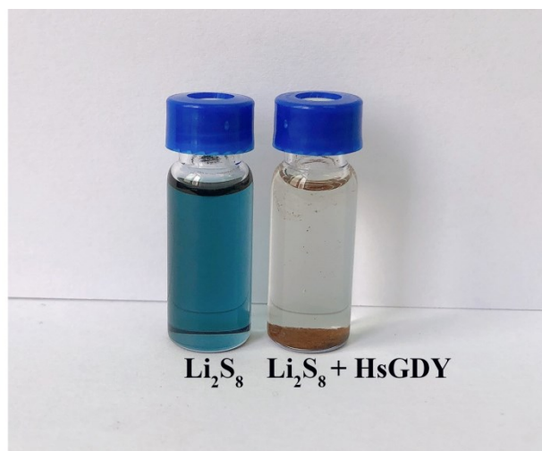
Fig. S14 LiPSs adsorption tests of HsGDY. 0.5 mM \text{Li}_2\text{S}_8 solution was prepared by mixing \text{Li}_2\text{S} and \text{S}_8 powder in DMSO. Afterwards, HsGDY (3 mg) were added into 1 mL \text{Li}_2\text{S}_8 (0.5 mM) solution and kept standing for 48 hours.
