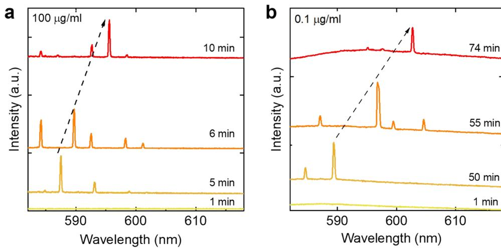
**Figure S9.** Lasing spectra of Bodipy microdroplet with various enzyme-substrate reaction time based on the identical droplet. **(a)** 100 µg/ml. **(b)** 0.1 µg/ml.
