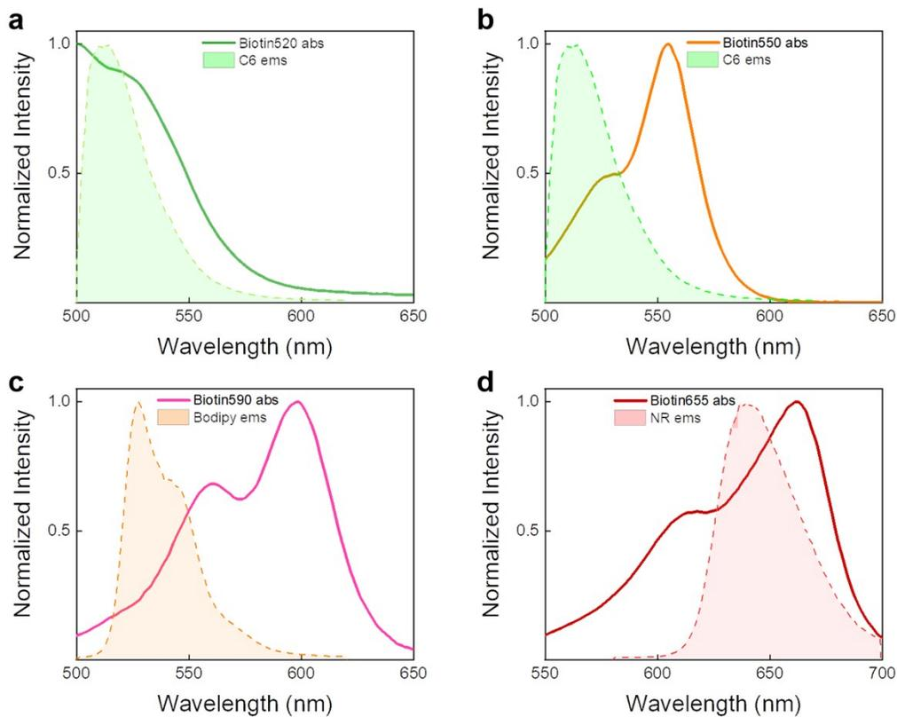
**Figure S10.** Normalized emission spectra of the respective donor in liquid crystal and absorption spectra of corresponding acceptor molecules in water. **(a)** Coumarin 6 (C6) droplet with Biotin 520 molecule; **(b)** C6 droplet with Biotin 550 molecule; **(c)** Bodipy droplet with Biotin 590 molecule; **(d)** Nile Red (NR) droplet with Biotin 655 molecule.
