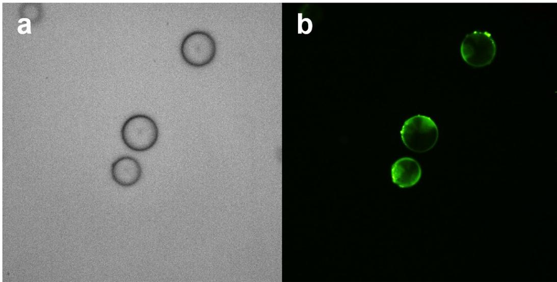
**Figure S6. (a)** Bright-field image of plain LC microdroplets. **(b)** Fluorescence image showing binding of SA-AF514 on the plain LC microdroplets surface.
