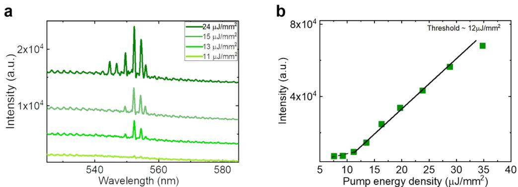
**Figure S5. (a)** Lasing spectra of 120- $\mu\text{M}$  Biotin520 binding to 20-mM C6 microdroplet ( $A/D$  ratio = 0.006) with relatively low pump energy densities; the curves have been vertically shifted for clarity. **(b)** Spectrally integrated Biotin520 laser output as a function of pump energy density extracted from the spectra shown in **(a)**, where the wavelength range is 545-560 nm, and the solid line denotes a linear fit; the lasing approximately 12  $\mu\text{J}/\text{mm}^2$ .
