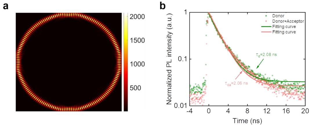
**Figure S1.** (a) Simulation of 10  $\mu\text{m}$  diameter WGM resonators displaying the electric field distribution. (b) Time-resolved fluorescence lifetime measurement of donor microdroplet before and after adding acceptor solution (A/D ratio = 0.01). The FRET efficiency is around 1.5% ( $E_f = 1 - \tau_{da} / \tau_d$ ). The solid curves were fitted by the scattered dots according to the exponential decay functions.
