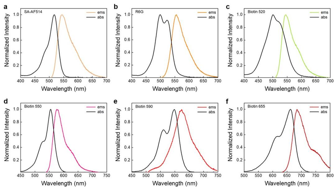
**Figure S11.** Normalized absorption and emission spectra of **(a)** SA-AF514; **(b)** R6G; **(c)** Biotin 520; **(d)** Biotin 550; **(e)** Biotin 590; **(f)** Biotin 655.
