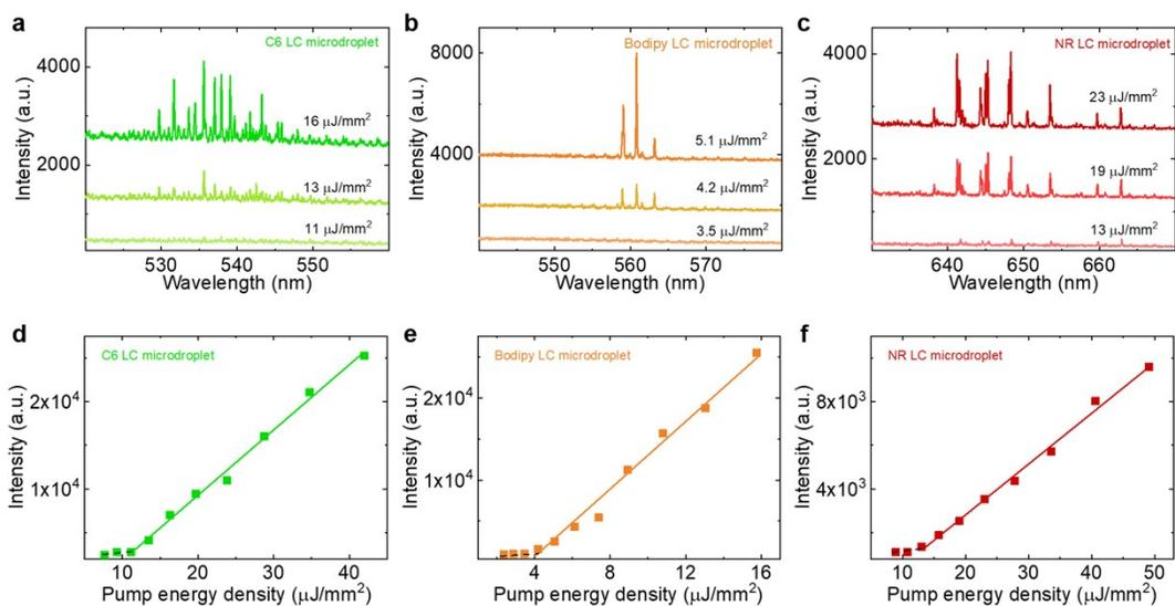
**Figure S12.** (a-c) Lasing spectra of C6, Bodipy and NR LC microdroplet, with relatively low pump energy densities (excitation wavelength: 450 nm, 488 nm and 532 nm). (d-f) Spectrally integrated R6G laser output as a function of pump energy density extracted from the spectra shown in (a-c).
