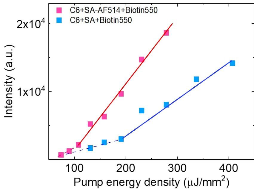
**Figure S7.** Spectrally integrated FRET laser output as a function of pump energy density. Pink line: 450 nm excitation for SA-AF514 coated microdroplet binding with Biotin 550. Blue line: 450 nm excitation for pure SA coated microdroplet binding with Biotin 550. The solid lines show linear fits.
