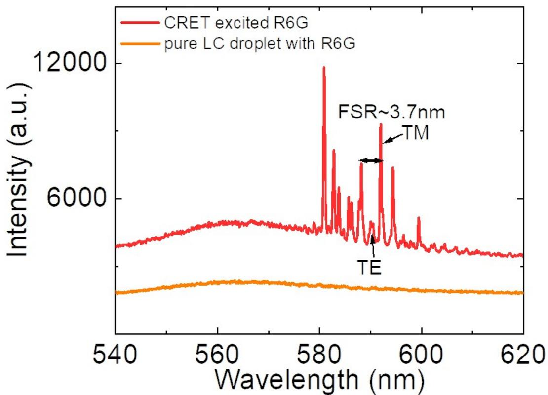
**Figure S2.** Laser and fluorescence emission spectra of a pure microdroplet (i.e., no dyes inside) and C6-doped microdroplet immersed in 0.1 mM R6G solution under the condition of the same pump energy and same excitation wavelength. (excitation wavelength: 450 nm). TE and TM modes are clearly labeled within the spectrum. Free spectral range (FSR) is around 3.7nm. Diameter of droplet= 24  $\mu$ m.
