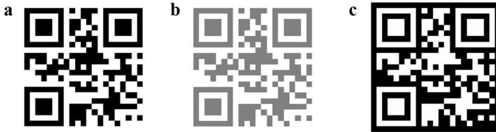
**Figure S9.** The simulation results of the images under bright daylight condition. (a) The original QR code image. (b) The image is overexposed under bright daylight condition. (c) The pre-processing result by OPU array proves the contrast enhancement effect.
