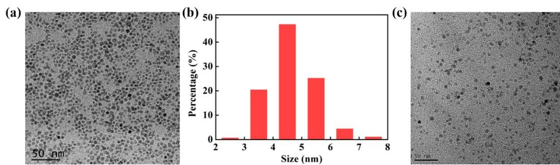
**Fig. S1** (a) TEM image and (b) size distribution of IONP-OA. (c) TEM image of IONP-P.
