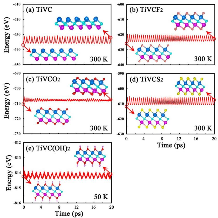
**Figure S3.** The pristine and functionalized TiVC MXenes after *ab initio* molecular dynamics simulations of 20 ps.
