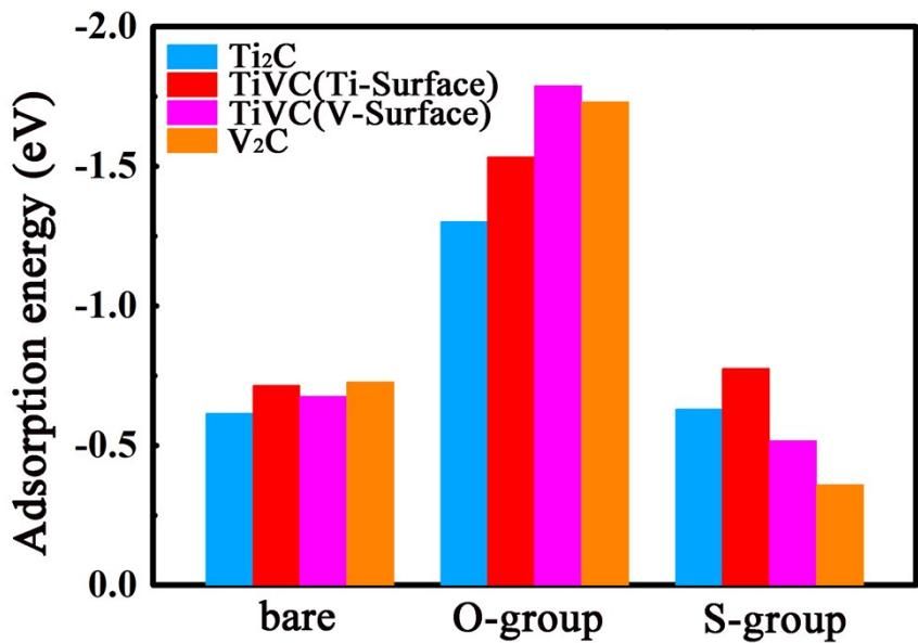
**Figure S6.** The average adsorption energy of multi-Li ions on favorable adsorption sites of  $\text{TiVC}$ ,  $\text{TiVCO}_2$  and  $\text{TiVCS}_2$  monolayers.
