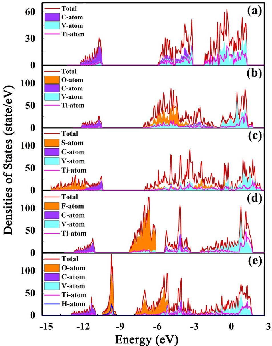
**Figure S4.** The density of states (DOS) for (a) TiVC, (b) TiVCO<sub>2</sub>, (c) TiVCS<sub>2</sub>, (d) TiVCF<sub>2</sub>, and (e) TiVC(OH)<sub>2</sub> monolayers. Note that the Fermi levels are set to zero.
