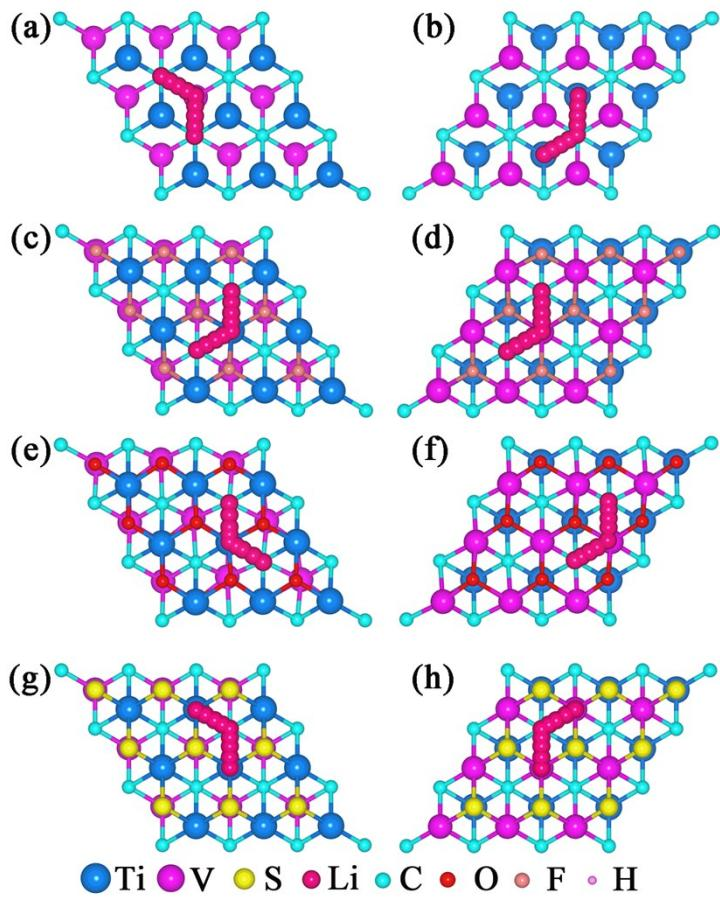
**Figure S5.** The diffusion pathway of Li ion on (a) Ti and (b) V surfaces of pristine TiVC monolayer, (c) Ti and (d) V surfaces of TiVCF<sub>2</sub> monolayer, (e) Ti and (f) V surfaces of TiVCO<sub>2</sub> monolayer, and (g) Ti and (h) V surfaces of TiVCS<sub>2</sub> monolayer (Referring to Figure 1 for interpretation of atomic color).
