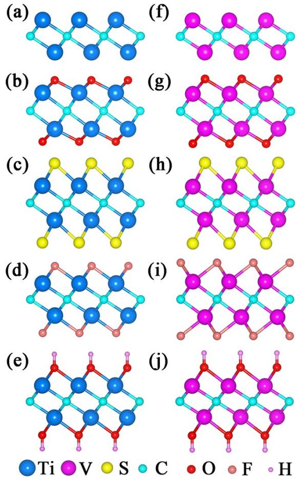
**Figure S1.** Side views for the most stable configurations of (a)  $\text{Ti}_2\text{C}$ , (b)  $\text{Ti}_2\text{CO}_2$ , (c)  $\text{Ti}_2\text{CS}_2$ , (d)  $\text{Ti}_2\text{CF}_2$ , (e)  $\text{Ti}_2\text{C}(\text{OH})_2$ , and (f)  $\text{V}_2\text{C}$ , (g)  $\text{V}_2\text{CO}_2$ , (h)  $\text{V}_2\text{CS}_2$ , (i)  $\text{V}_2\text{CF}_2$  and (j)  $\text{V}_2\text{C}(\text{OH})_2$  monolayers after relaxation, respectively (Referring to Figure 1 for interpretation of atomic color).
