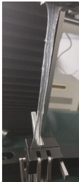
Figure S5. Optical image of the stretched PAAK/CMC-24M in the universal tensile testing machine.
