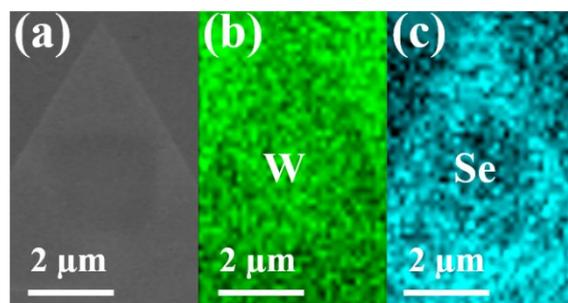
**Fig. S2.** (a) Field emission scanning electron microscope (FE-SEM) image of the prepared WSe<sub>2</sub> nanosheet. Energy dispersive X-ray spectroscopy (EDX) elemental mapping images of W (b) and Se (c).
