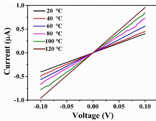
**Fig. S6.** The temperature dependent conductive behaviors of the WSe<sub>2</sub> based memristor at the low resistance state. As the temperature is increased, the current (resistance) increases (decreases), suggesting the semiconducting behaviors rather than the metallic conductance.
