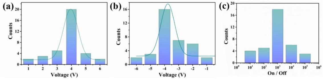
**Fig. S5.** Statistical analysis of the memristive parameters of the fabricated 36 WSe<sub>2</sub>-based memristors. (a) Statistical analysis of the set voltages. (b) Statistical analysis of the reset voltages. (c) Statistical analysis of the ON/OFF ratio.
