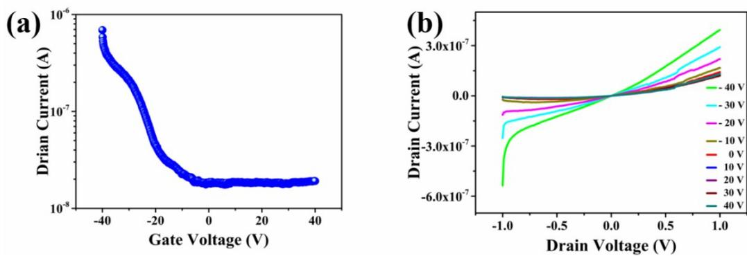
**Fig. S6.** (a) The transport property and (b) the output characteristics of WSe<sub>2</sub>-based field effect transistor with SiO<sub>2</sub> as gate dielectric and Ag as source and drain electrodes.
