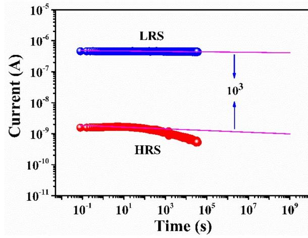
Fig. S8. Retention performance of the 2D WSe<sub>2</sub> based memristor with power law extrapolation to 10 years.
