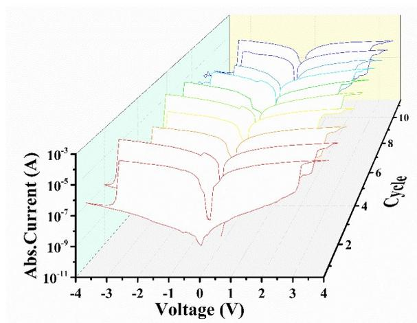
**Fig. S4.** 10 experimental switching loops of the fabricated memristor based on WSe<sub>2</sub> nanosheet.
