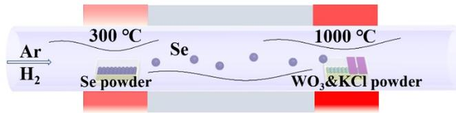
**Fig. S1.** Schematic of growth process of WSe<sub>2</sub> by chemical vapor deposition method.
