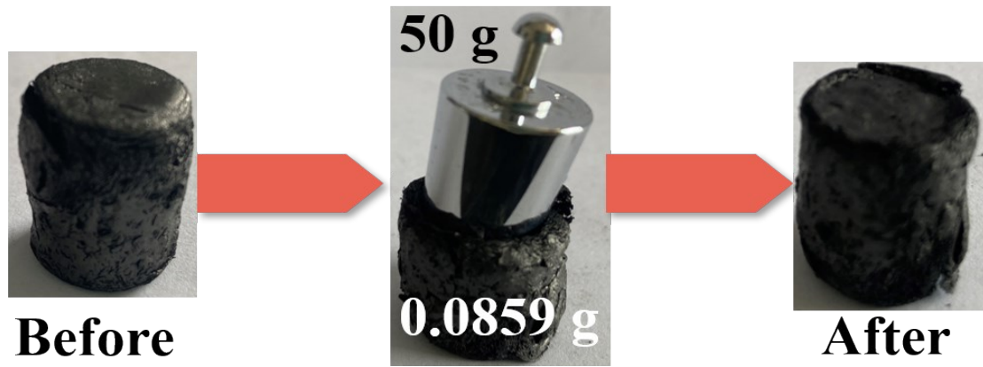
Fig. S2 Typical digital images of S3 before, during and after the compression test.
