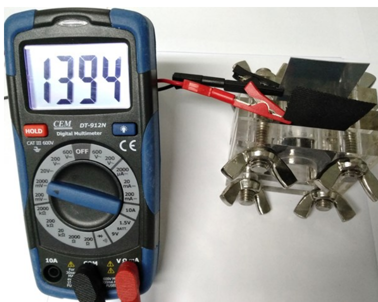
Fig. S15 Photograph of the Zn-air battery employing the commercial cathode, giving an open-circuit potential of 1.394 V.
