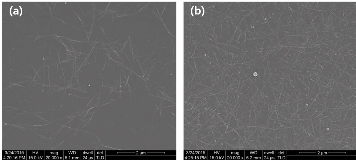
**Fig. S2** SEM images of the SWCNT networks on a SiO<sub>2</sub>/Si substrate **(a)** w/o and **(b)** with APTES SAM treatment.
