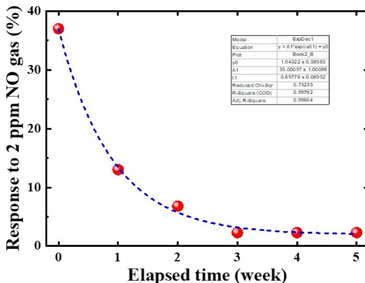
**Fig. S4** Long-term stability test; variation of response values with the elapsed time.
