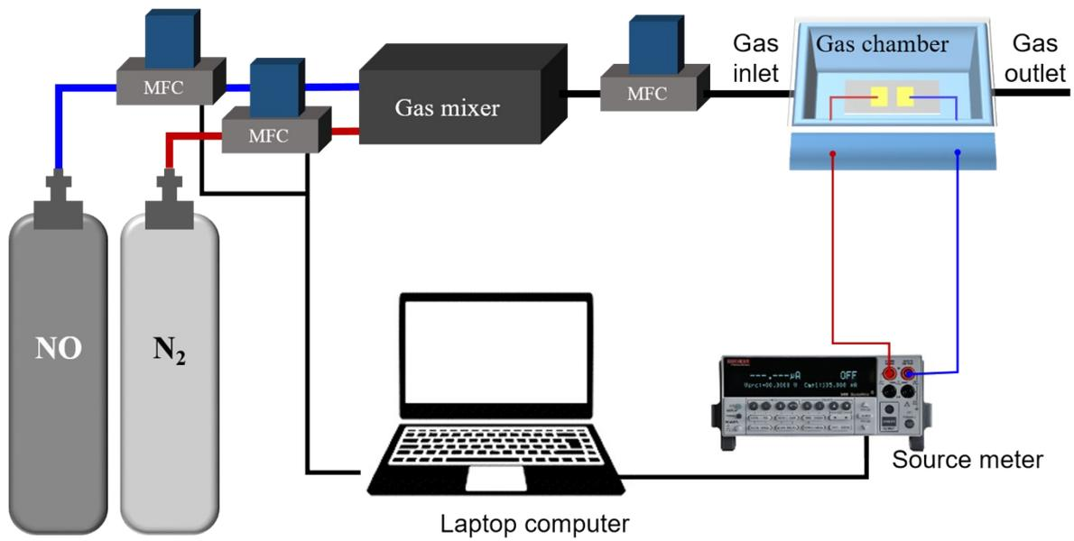
**Fig. S1** Schematic of the measurement system for chemiresistive-type gas sensing device.
