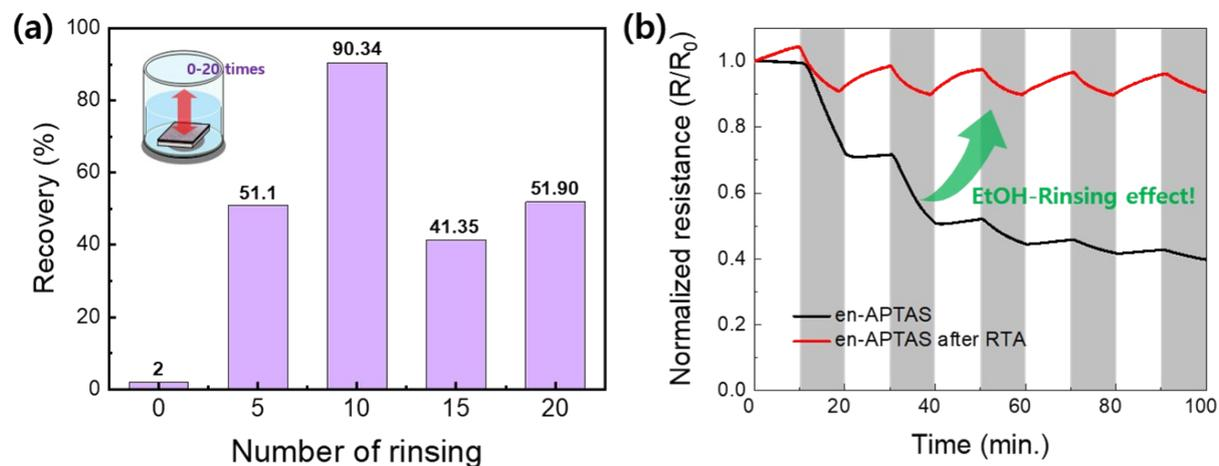
**Fig. S3** Recovery variation depending on the number of ethanol rinsing. **(a)** Plot of the recovery (%) versus the number of rinsing. **(b)** Variation in normalized resistance ( $R/R_0$ ) on time.
