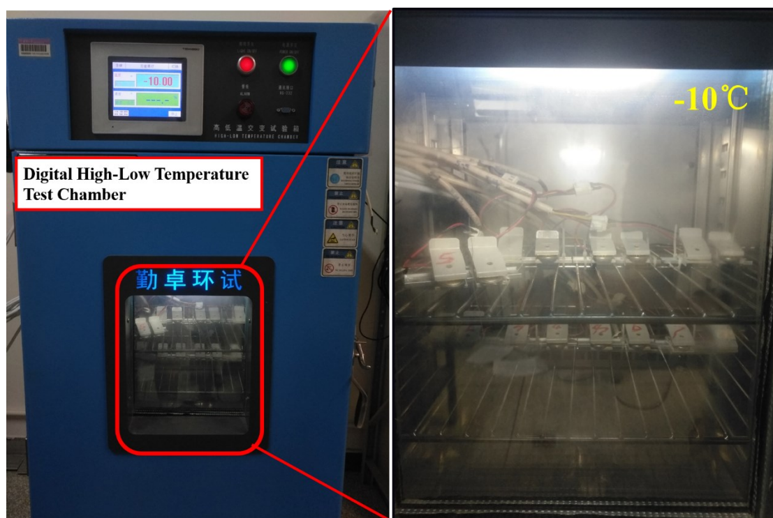
Figure S8. Photograph of 2032 cells being tested in digital high-low temperature test chamber.
