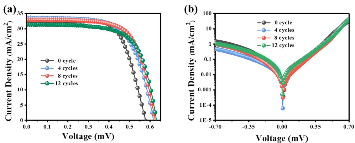
**Fig. S4.** (a) Photocurrent  $J-V$  curves, and (b) dark  $J-V$  curves of PEDOT:PSS/Si solar cells based on the CdS nanowire layer by spin-coating different cycles.
