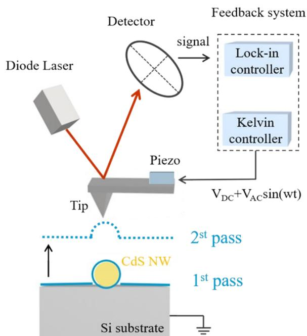
**Fig. S5.** The sample structure and configuration of dual-pass AM mode KPFM measurement. During the second-pass scan, a DC and AC mixed voltage is applied to the tip, and the Kelvin feedback system minimizes the tip oscillation and outputs  $V_{DC}$  as KPFM signal.
