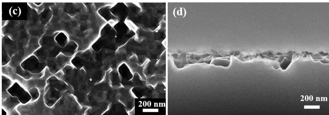
**Fig. S3.** SEM image of nanostructured Si obtained by TMAH modified Si nanowires
