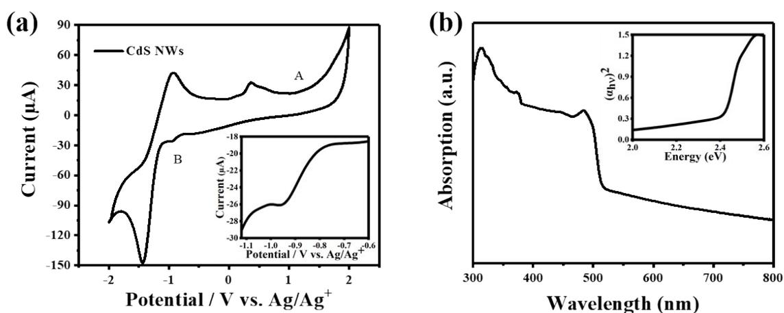
**Fig. S6.** (a) cyclic voltammetry of CdS nanowires in acetonitrile solution (The inset is a partial enlarged view of area B). (b) UV/Vis absorption spectrum of CdS NWs (The inset is the fitted optical band gap diagram).
