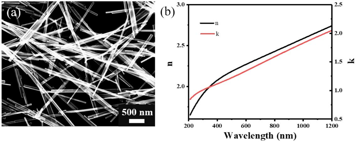
**Fig. S1.** (a) SEM image of CdS nanowires spin-coated on the back of silicon wafer, (b) Refractive index ( $n$ ) and absorption coefficient ( $k$ ) curves of the TiN film.
