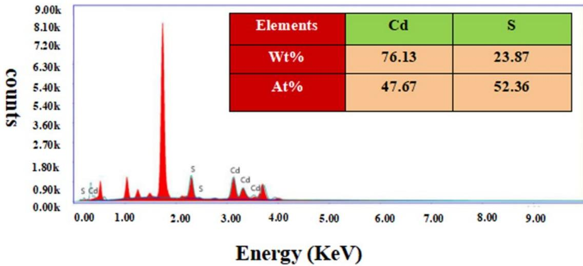
**Fig. S2.** Energy dispersive spectra taken from the CdS nanowires.
