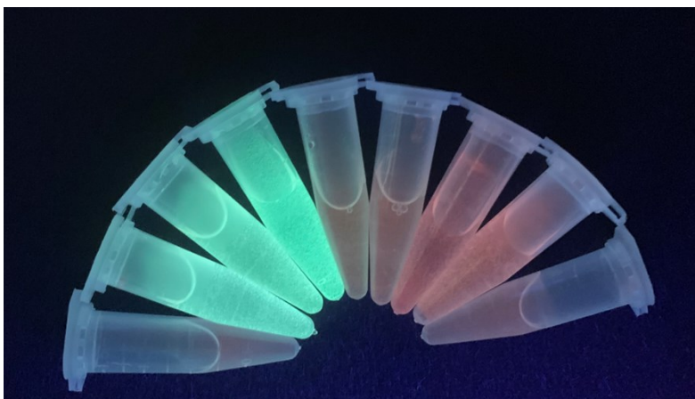
Figure S3. Photographs of the MPA-AuNCs under 365 nm UV light with addition of 2M-IM ( c_{2\text{M-IM}} = 6 \text{ mM} ) and different concentrations of \text{Zn}^{2+} (left to right: c_{\text{Zn}^{2+}} = 3, 2.5, 2.25, 2, 1.75, 1.5, 1.25, 1, 0.5 \text{ mM} ).
