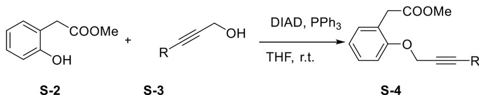
Synthesis of **S-4**: To a 50-mL oven-dried flask containing a magnetic stirring bar, **S-2** (1.7 g, 10.0 mmol), propargyl alcohol **S-3** (11.0 mmol, 1.1 equiv.),  $\text{PPh}_3$  (3.9 g, 1.5 equiv.) in dry THF (30.0 mL), was added DIAD (3.0 g, 1.5 equiv.) slowly at  $0^\circ\text{C}$ ,
