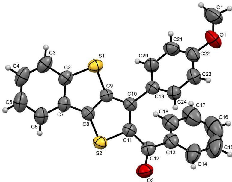
Compound **9d** in according XRD data. Thermal ellipsoids are shown at 50% probability level.
