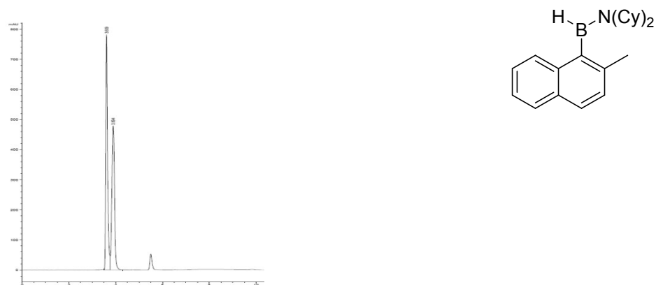
Figure 9 : Sample 10h chromatogram at 0°C using Hexane:isopropanol 99:1 as the mobile phase
