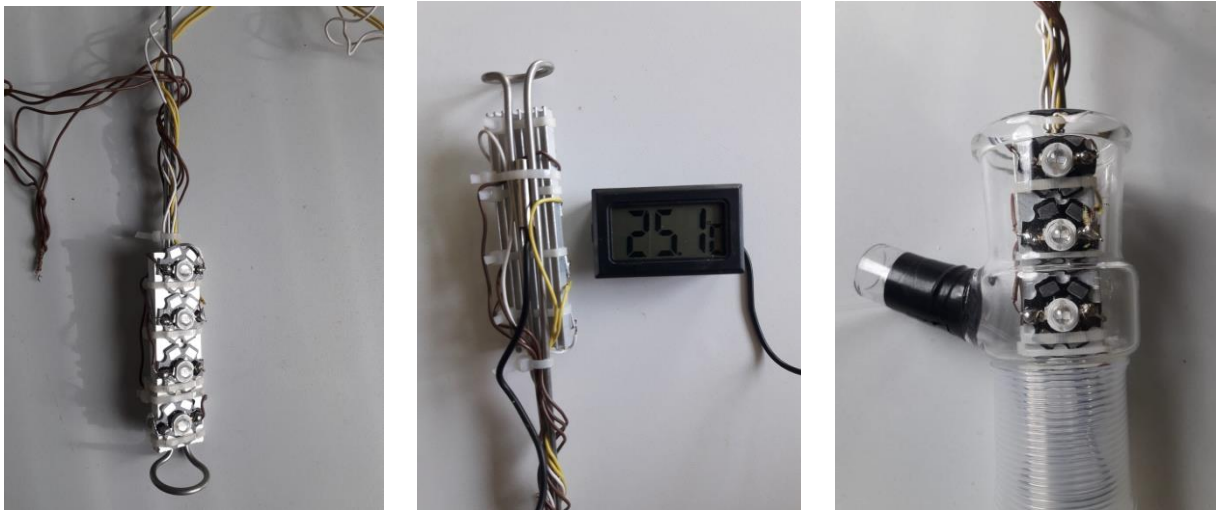
Figure S4 4X10W LED rack (the thermometer probe is placed on the aluminium heat exchanger)
