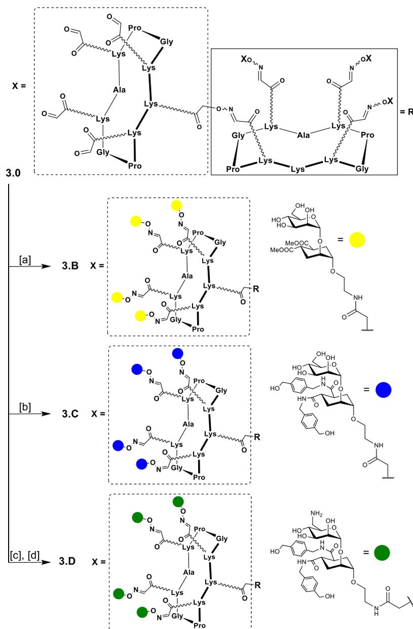
**Scheme S2.** Synthesis of mannose mimics-containing hexadecavalent glycodendrimers **3.B**, **3.C** and **3.D**. Conditions: [a] **S2**, 0.1% TFA in H<sub>2</sub>O, 37 °C; [b] **S4**, 0.1% TFA in H<sub>2</sub>O, 37 °C; [c] TFA/CH<sub>2</sub>Cl<sub>2</sub> (1:1, v/v); [d] **S6**, 0.1% TFA in H<sub>2</sub>O, 37 °C.
