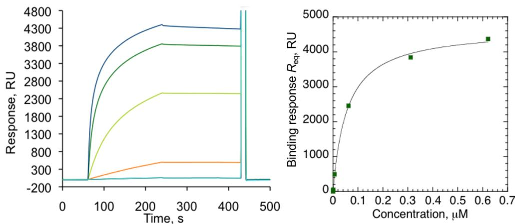
**Figure S22.** DC-SIGN S-ECD titration over a *StrepTactin* amine-coupled surface. Left panel shows the sensorgram of DC-SIGN S-ECD (concentrations from 0.62 nM to 622 nM) over immobilized *StrepTactin* (2700 RU). The surface was regenerated with 1M NaOH/ 50 mM NaCl. The right panel represents the corresponding binding responses as a function of DC-SIGN S-ECD concentration. The  $K_D$  extracted from *steady state affinity* model is equal to 57 nM.
