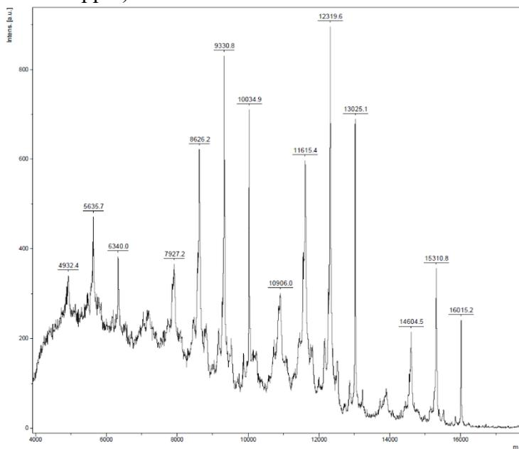
**Figure S14.** MALDI-TOF of **4.C**.  $m/z$  calcd for  $C_{747}H_{1050}N_{123}O_{266}$   $[M+H]^+$ : 16009.0, found: 16015.2 (+6.2, error = 387 ppm).
