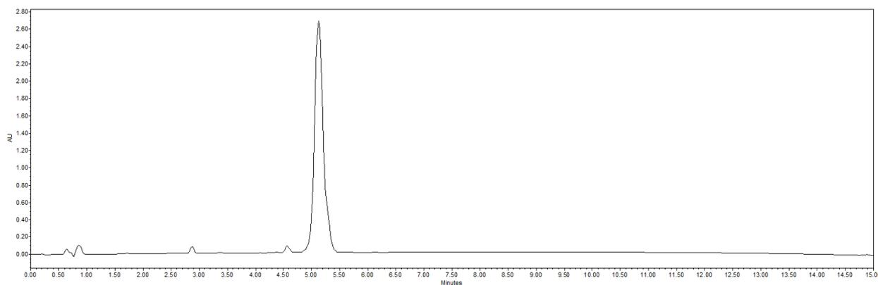
**Figure S18.** Analytical RP-HPLC of **3.C**.  $t_R = 5.13$  min (C18,  $\lambda = 214$  nm 5-100% B in 15 min).
