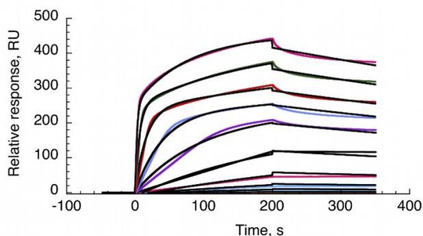
**Figure S23:** Kinetic analysis of BSA-Man titration over a DC-SIGN S-ECD surface. The fit (black curves) derives from the *heterogeneous ligand* model. The extracted values from the fit are:  $K_{D1}=6.48$  nM and  $K_{D2}= 0.27$  nM. The respective  $R_{max}$  are 209.9 RU and 233.8 RU.
