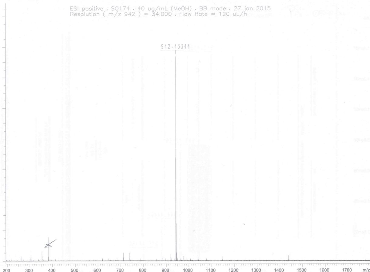
**Figure S9.** HRMS (ESI-TOF) of **S6**.  $m/z$  calcd. for  $[C_{44}H_{65}N_5O_{16}Na]^+$ : 942.43240; found: 942.43344 (error = +1.1 ppm).
