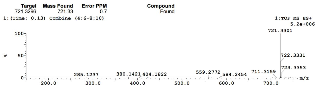
**Figure S8.** HRMS (ESI-TOF) of **S4**.  $m/z$  calcd for  $C_{34}H_{49}N_4O_{13} [M+H]^+$ : 721.3296, found: 721.3301 (error = +0.7 ppm).
