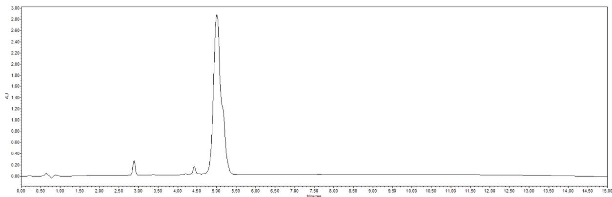
**Figure S21.** Analytical RP-HPLC of **4.C**.  $t_R = 5.01$  min (C18,  $\lambda = 214$  nm 5-100% B in 15 min).
