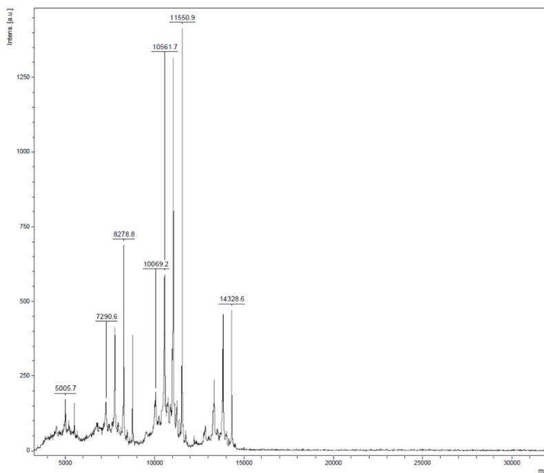
**Figure S10.** MALDI-TOF of **3.B**.  $m/z$  calcd for  $C_{603}H_{942}N_{111}O_{286} [M+H]^+$ : 14322.5, found: 14328.6 (+6.1, error = 426 ppm).
