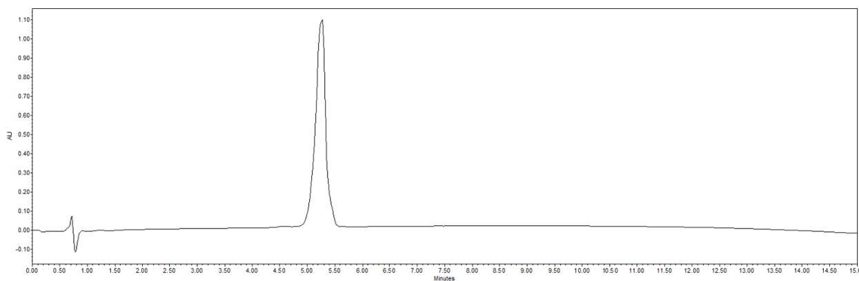
**Figure S20.** Analytical RP-HPLC of **4.B**.  $t_R = 5.26$  min (C18,  $\lambda = 214$  nm 5-100% B in 15 min).
