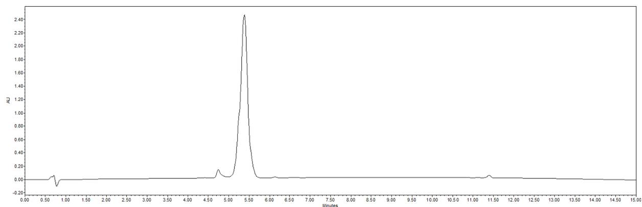
**Figure S17.** Analytical RP-HPLC of **3.B**.  $t_R = 5.38$  min (C18,  $\lambda = 214$  nm 5-100% B in 15 min).
