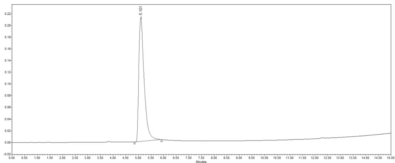
**Figure S19.** Analytical RP-HPLC of **3.D**.  $t_R = 5.10$  min (C18,  $\lambda = 214$  nm 5-100% B in 15 min.).
