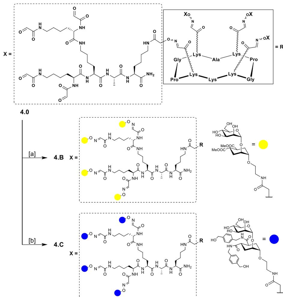
**Scheme S3.** Synthesis of mannoside-containing hexadecavalent glycodendrimers **4.B** and **4.C**. Conditions: [a] **S2**, 0.1% TFA in  $H_2O$ , 37 °C; [b] **S4**, 0.1% TFA in  $H_2O$ , 37 °C.
