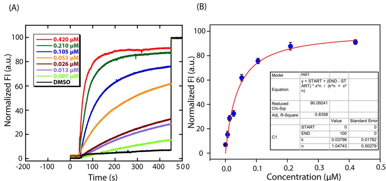
**Fig. S8.** Concentration-dependent transmembrane transport of  $\text{Cl}^-$  ion in the presence of compound **1c** across the EYPC/CHOL-LUV $\supset$ HPTS. The ion transport activity was measured by HPTS fluorescence assay using a pH gradient ( $\text{pH}_{\text{in}} = 7.2$ ,  $\text{pH}_{\text{out}} = 7.8$ ; A). The  $\text{EC}_{50}$  value was calculated using the modified Hill equation (B).
