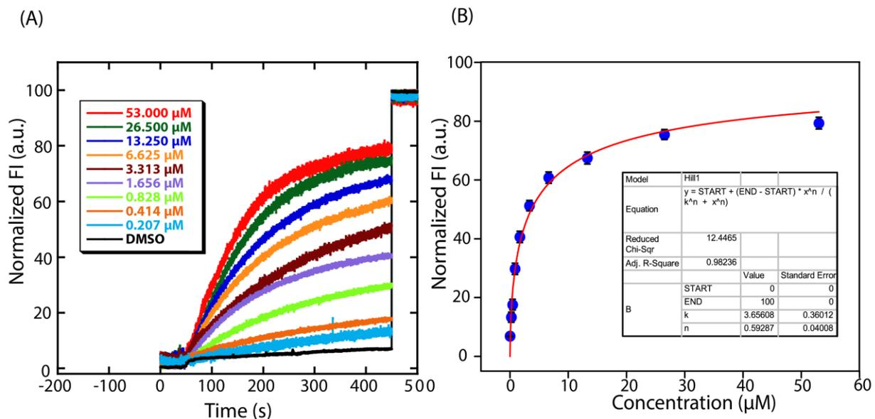
**Fig. S6.** Concentration-dependent transmembrane transport of  $\text{Cl}^-$  ion in the presence of compound **1a** across the EYPC/CHOL-LUV $\supset$ HPTS. The ion transport activity was measured by HPTS fluorescence assay using a pH gradient ( $\text{pH}_{\text{in}} = 7.2$ ,  $\text{pH}_{\text{out}} = 7.8$ ; A). The  $\text{EC}_{50}$  value was calculated using the modified Hill equation (B).
