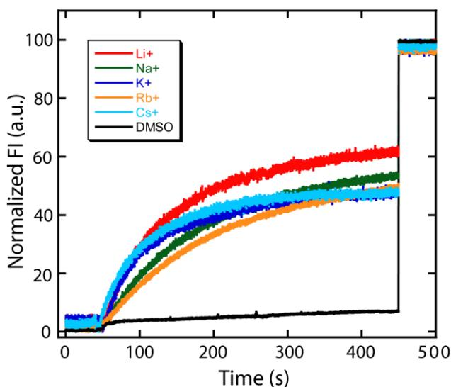
**Fig. S10.** Cation selectivity of compound **1c** (0.038  $\mu$ M), as measured by HPTS assay in the presence of pH gradient.
