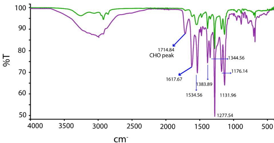
**Fig. S14.** FT-IR spectrum of sulfonium salt **2** in the absence of 365 nm UV light (green line) and after 10 min (violet line) irradiated with 365 nm light.
