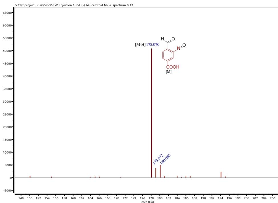
**Fig. S15.** Mass spectra of intermediate **5** upon photoirradiation of compound **2**.
