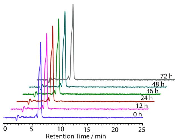
**Fig. S11.** HPLC traces of proanionophore **2** at different time intervals in the absence of Fenton's reagent. A similar spectral pattern was observed in the absence of GSH.
