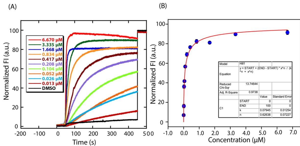
**Fig. S7.** Concentration-dependent transmembrane transport of  $\text{Cl}^-$  ion in the presence of compound **1b** across the EYPC/CHOL-LUV $\Delta$ HPTS. The ion transport activity was measured by HPTS fluorescence assay using a pH gradient ( $\text{pH}_{\text{in}} = 7.2$ ,  $\text{pH}_{\text{out}} = 7.8$ ; A). The  $\text{EC}_{50}$  value was calculated using the modified Hill equation (B).
