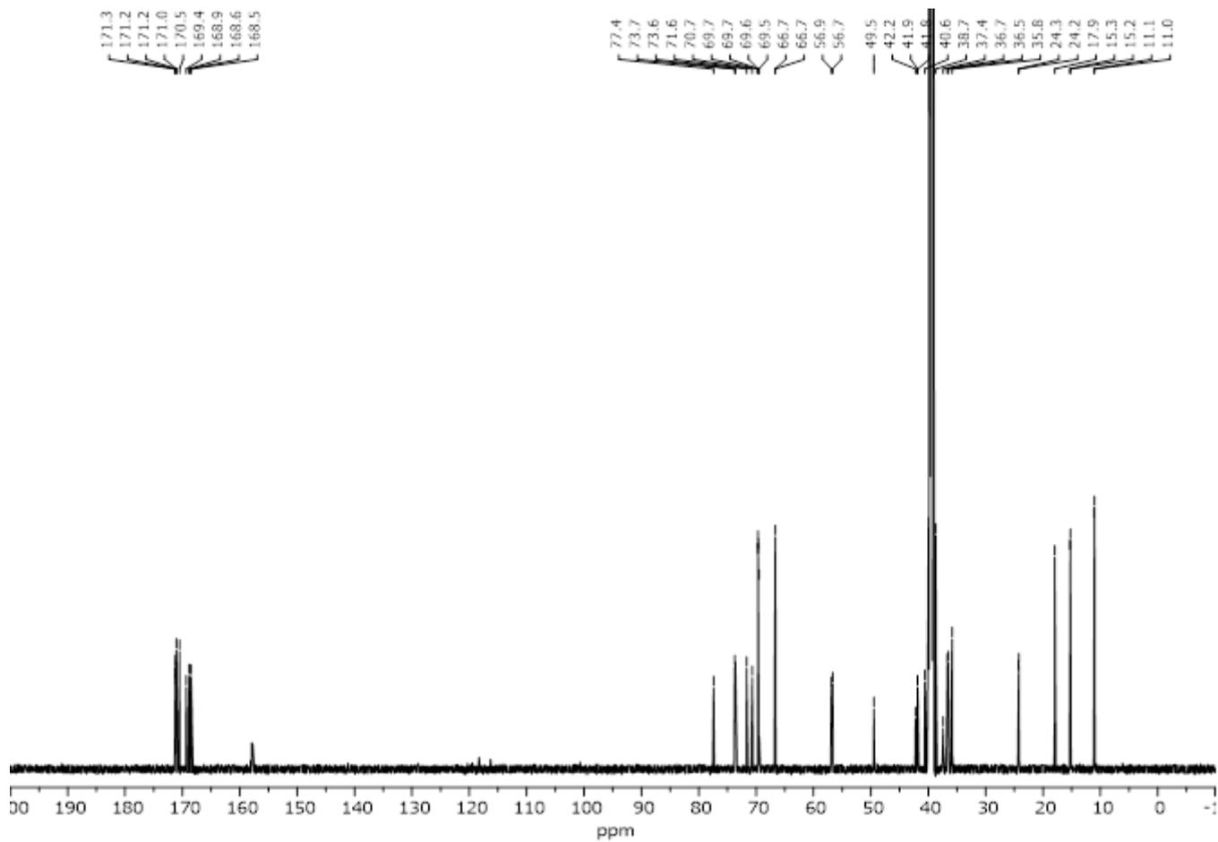
$^{13}\text{C}$ -NMR Spectrum of Asn $^{\beta}$ -Rha-Peptide with TEG-Spacer **S16** (150 MHz, [d $_6$ ]-DMSO)
