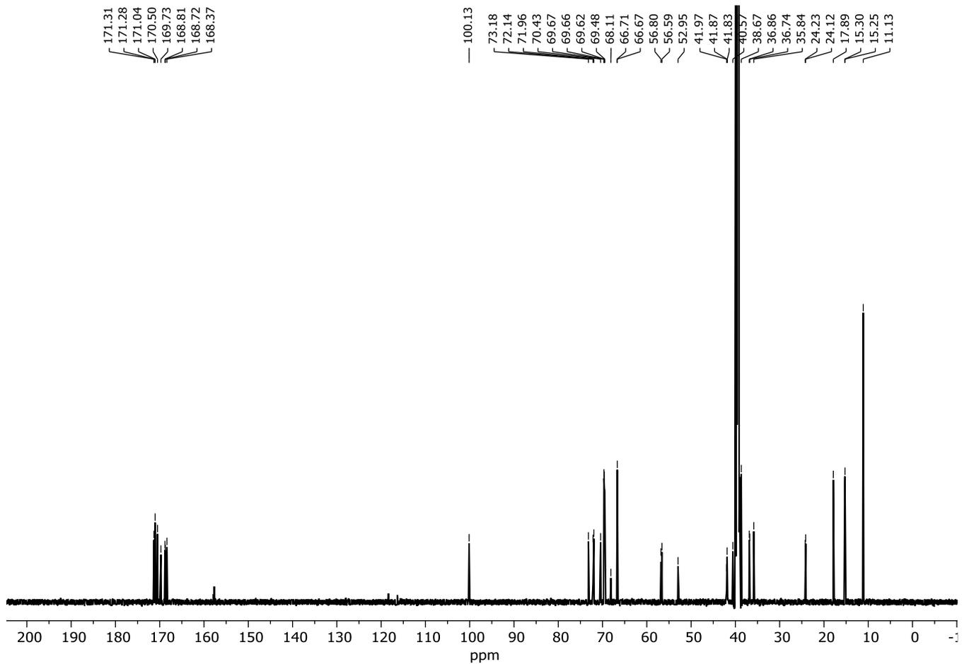
$^{13}\text{C}$ -NMR Spectrum Ser $^{\beta}$ -Rha-Peptide with TEG-Spacer **S12** (150 MHz, [d<sub>6</sub>]-DMSO)
