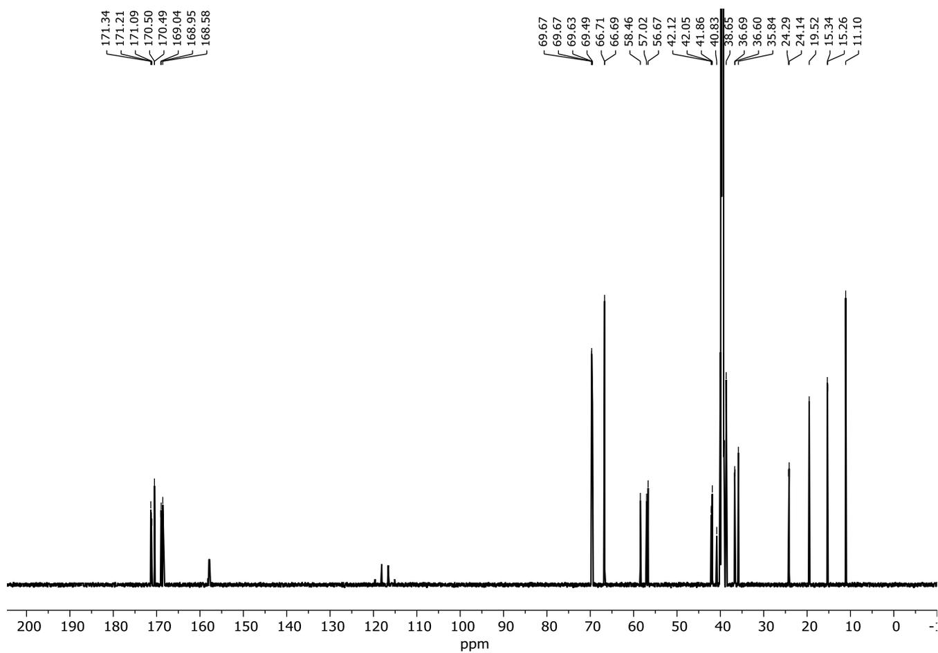
$^{13}\text{C}$ -NMR Spectrum of naked Thr-Peptide with TEG-Spacer **S18** (200 MHz,  $[\text{d}_6]$ -DMSO)
