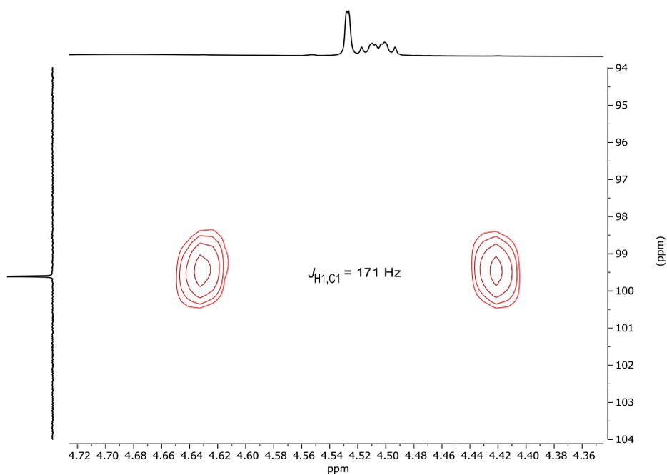
$^1\text{H}$ - $^{13}\text{C}$ -coupled HSQC-Spectrum of Glycopeptide **S11**: H-1, C-1 coupling constant  $J_{\text{H}_1, \text{C}_1}$
