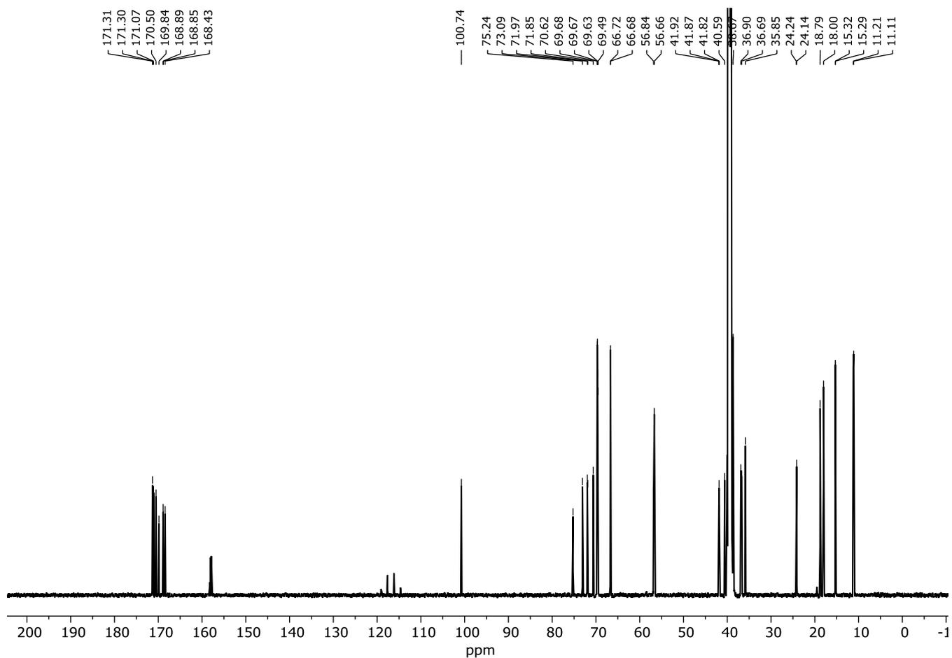
$^{13}\text{C}$ -NMR Spectrum of Thr $^{\beta}$ -Rha-Peptide with TEG-Spacer **S14** (200 MHz, [d6]-DMSO)
