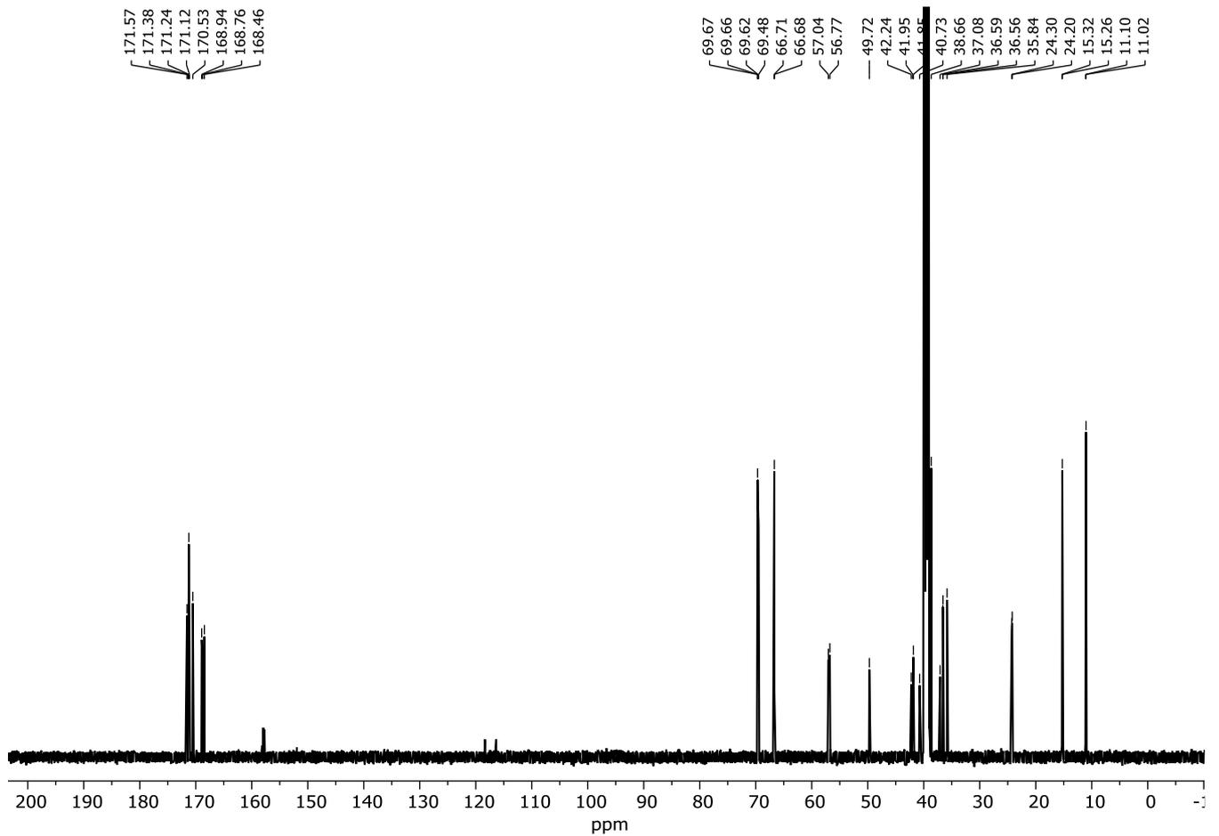
$^{13}\text{C}$ -NMR Spectrum of Naked Asn-Peptide with TEG-Spacer **S19** (150 MHz, [d6]-DMSO)
