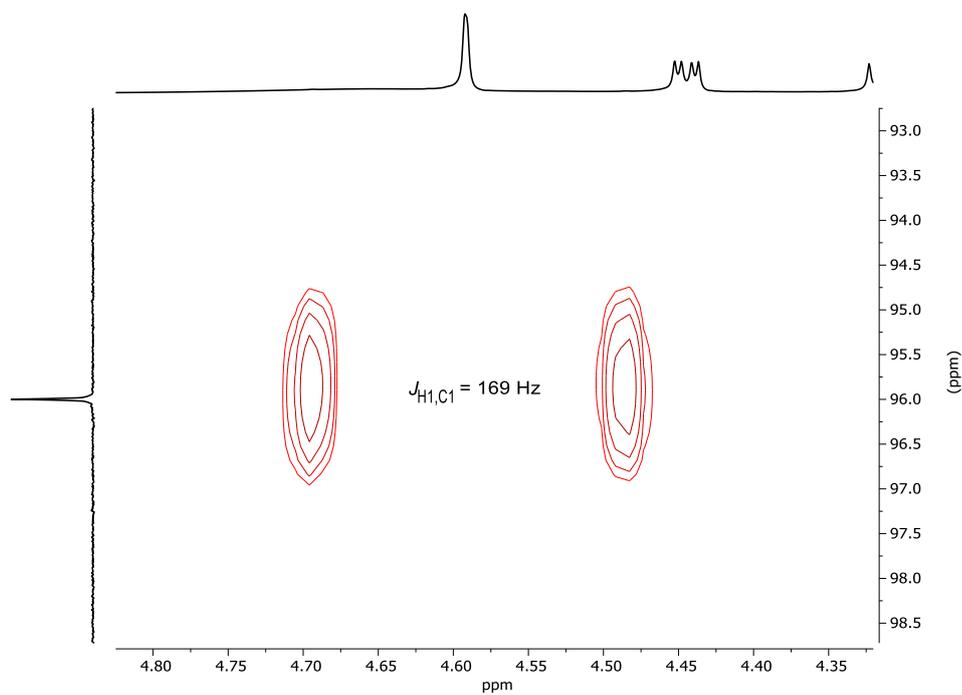
$^1\text{H}$ - $^{13}\text{C}$ -coupled HSQC-Spectrum of Glycopeptide **13**: H-1,C-1 coupling constant  $J_{\text{H}_1,\text{C}_1}$
