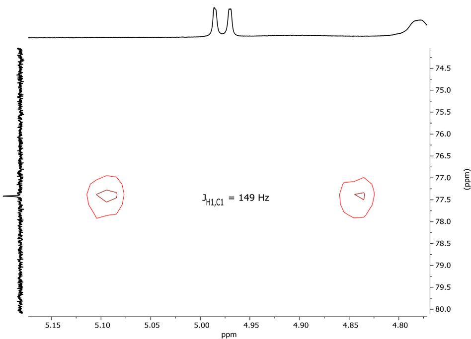
$^1\text{H}$ - $^{13}\text{C}$ -coupled HSQC-Spectrum of Glycopeptide **16**: H-1-C-1 coupling constant  $J_{\text{H}_1, \text{C}_1}$
