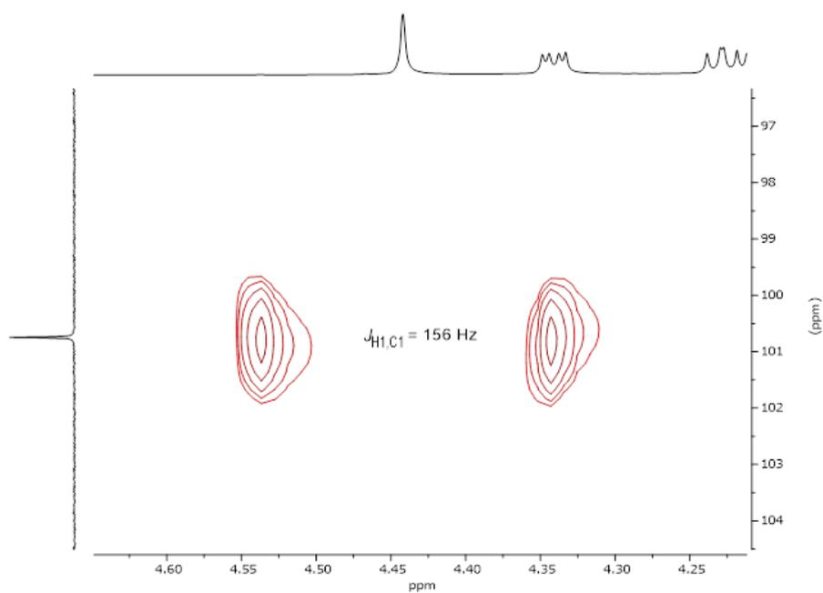
$^1\text{H}$ - $^{13}\text{C}$ -coupled HSQC-Spectrum of Glycopeptide **S14**: H-1,C-1 coupling constant  $J_{\text{H1,C1}}$
