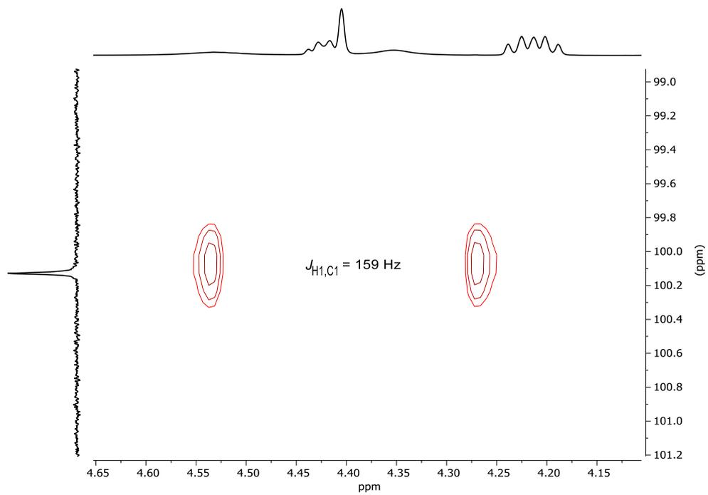
$^1\text{H}$ - $^{13}\text{C}$ -coupled HSQC-Spectrum of Glycopeptide **S12**: H-1,C-1 coupling constant  $J_{\text{H1,C1}}$
