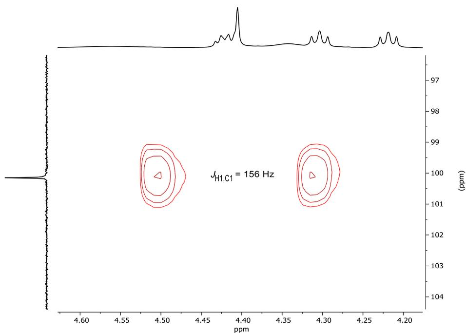
$^1\text{H}$ - $^{13}\text{C}$ -coupled HSQC-Spectrum of Glycopeptide **12**: H-1,C-1 coupling constant  $J_{\text{H}_1, \text{C}_1}$
