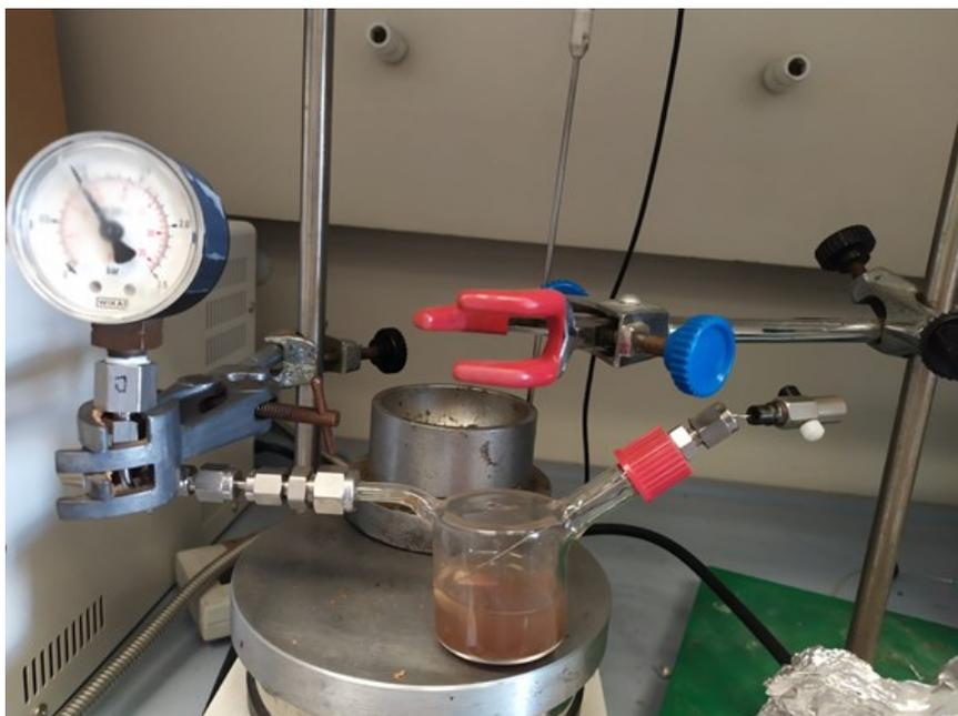
Figure S1. Photograph of the catalytic device employed for the tandem reaction.
