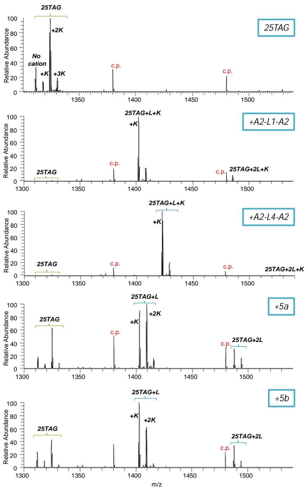
**Fig. S4** ESI-MS spectra of 25TAG (5  $\mu$ M) in the absence (top) and in the presence of equimolar concentrations of ligands (L) **A2-L1-A2**, **A2-L4-A2**, **5a**, and **5b**, in 100 mM TMAA + 1 mM KCl buffer. **c.p.** = calibration peak ( $dT_6$ ).
