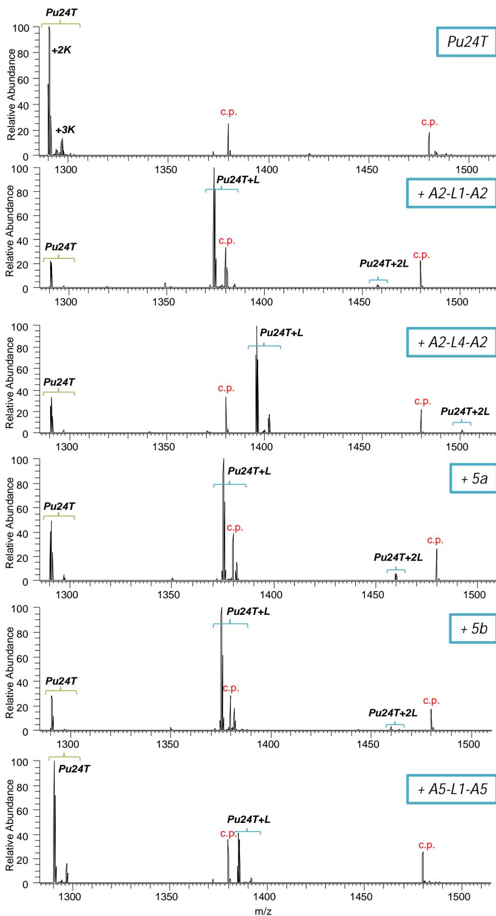
**Fig. S5** ESI-MS spectra of *Pu24T* (5  $\mu\text{M}$ ) in the absence (top) and in the presence of equimolar concentrations of ligands (L) **A2-L1-A2**, **A2-L4-A2**, **5a**, **5b**, and **A5-L1-A5**, in 100 mM TMAA + 1 mM KCl buffer. **c.p.** = calibration peak ( $dT_6$ ).
