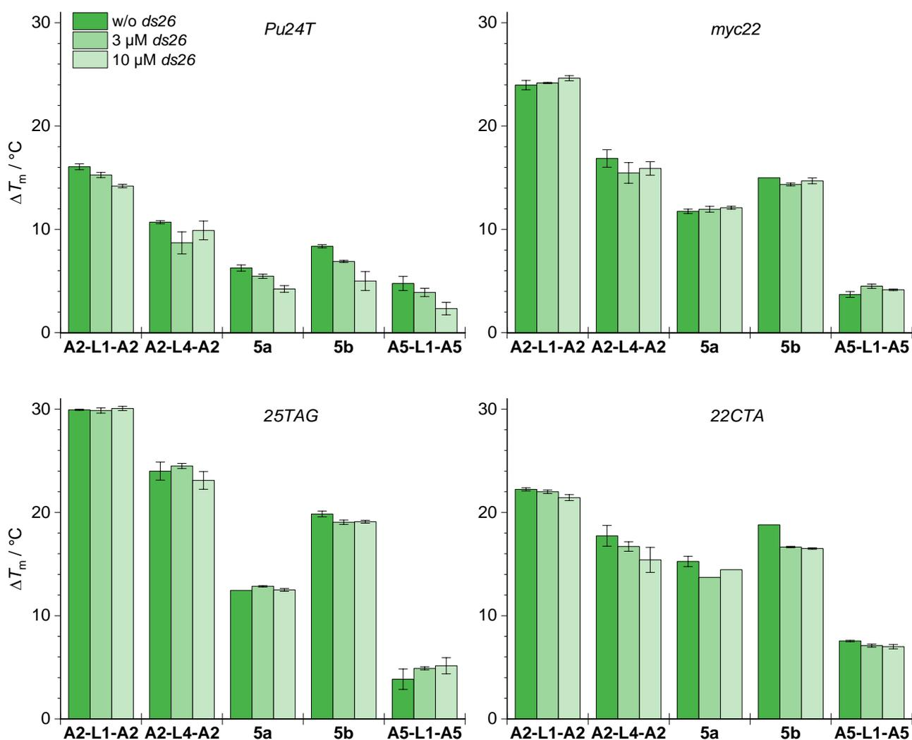
**Fig. S6** Effect of unlabelled double-stranded competitor (*ds26*) on the ligand-induced stabilization ( $\Delta T_m$ , °C) of G4-DNA (*Pu24T*, *myc22*, *25TAG*, *22CTA*) observed in fluorescence-melting experiments. Data are mean  $\pm$  s.d. from three measurements.
