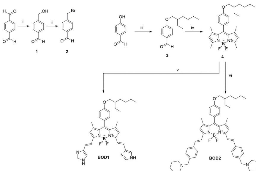
**Scheme S1.** Synthesis of **BOD1** and **BOD2**. Reaction conditions: i)  $\text{NaBH}_4$ , THF, EtOH; ii) NBS,  $\text{PPh}_3$ , DCM; iii)  $\text{K}_2\text{CO}_3$ , 2-ethylhexyl bromide, DMF; iv) a. 2,4-dimethyl pyrrole,  $\text{N}_2$ , TFA, DCM; b) p-chloranil; c)  $\text{Et}_3\text{N}$ ,  $\text{BF}_3 \cdot \text{OEt}_2$ ; v) 4-imidazole carboxaldehyde, piperidine, acetic acid, benzene; vi) compound 2, piperidine, acetic acid, benzene.
