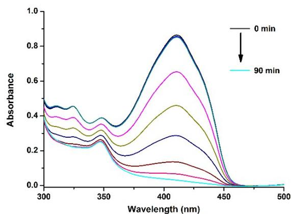
Figure S3. Decrease in the absorbance of DPBF (50  $\mu\text{M}$ ) in the presence of **BOD2** (2  $\mu\text{M}$ ) in 1%  $\text{H}_2\text{O}$  in acetonitrile. Sample is kept in dark in the first 30 minutes, then irradiated with 637 nm LED light.
