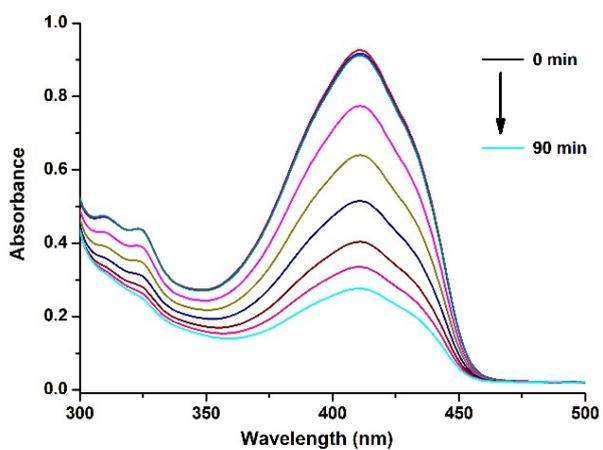
Figure S2. Decrease in the absorbance of DPBF (50 μM) in the presence of **BOD1** (2 μM) in 10% H<sub>2</sub>O in acetonitrile. Sample is kept in dark in the first 30 minutes, then irradiated with 637 nm LED light.
