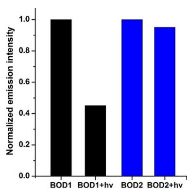
Figure S5. Normalized peak emission intensity of **BOD1** and **BOD2** at the presence and absence of 637 nm light. Light is introduced by an LED source for 120 min from a distance of 5 cm.
