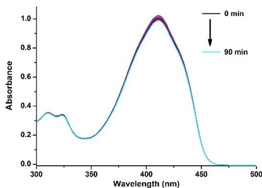
Figure S4. Decrease in the absorbance of DPBF alone (50  $\mu\text{M}$ ) in 1%  $\text{H}_2\text{O}$  in acetonitrile. Sample is kept in dark in the first 30 minutes, then irradiated with 637 nm LED light.
