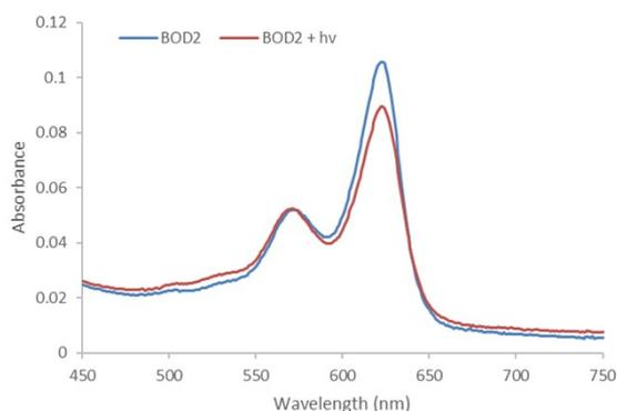
**Figure S11.** Change in UV-Vis Absorbance spectrum of **BOD2** after 2h irradiation with 637 nm light. Small decrease in absorption is contributed to formyl-**BOD2** formation.
