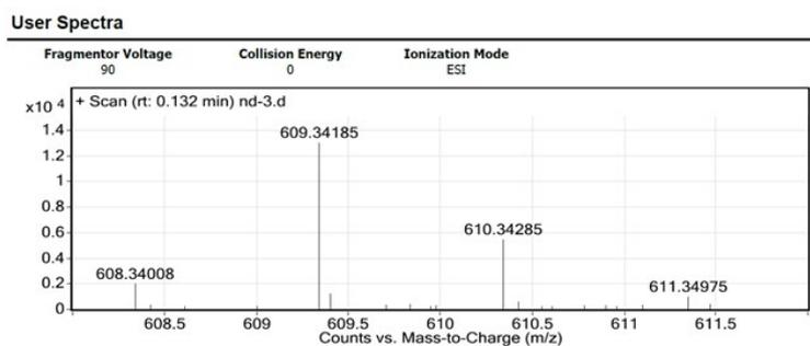
**Figure S9.** High Resolution ESI-MS Spectra of **BOD1** after 3h irradiation with 505 nm LED light from a distance of 5 cm. Values are 609.3325 for theoretical  $m/z$  of  $(M+H)^+$  and 609.34185 for experimental ( $\Delta$ : 13.13 ppm).
