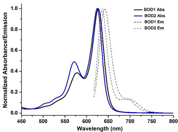
Figure S1. Normalized absorbance (solid) and fluorescence (dashed) spectra of BOD1 (black) and BOD2 (blue) in H<sub>2</sub>O/acetonitrile (1:99; v/v).
