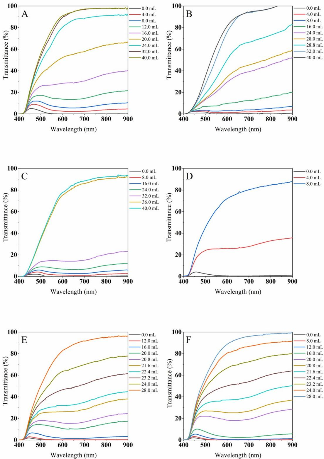
**Figure S5.** Transmittance spectra in the 400-900 nm part of the spectra during recovery with air injection for  $\text{TiO}_2$  NPs in different solvents. A) Ethanol; B) *n*-Propanol; C) *i*-Propanol; D) *n*-Butanol; E) *n*-Pentanol; F) *n*-Hexanol.
