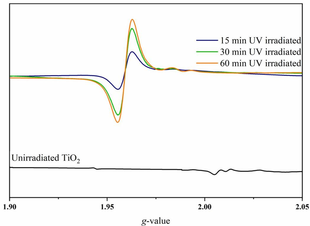
**Figure S1.** EPR spectra of unirradiated TiO<sub>2</sub> colloid and UV irradiated TiO<sub>2</sub> colloid for 15, 30 and 60 min. The peaks at  $g=2.0036$ ,  $2.0096$  and  $2.026$  correspond to Ti<sup>4+</sup>-O<sup>2-</sup> species, but peak at  $g=1.957$  corresponds to Ti<sup>3+</sup>
