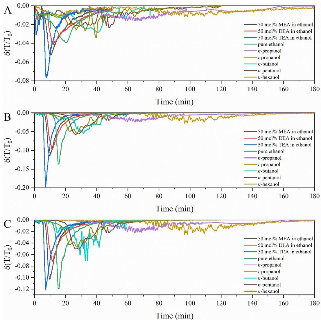
**Figure S4.**  $\delta(T/T_0)$  plots as a function of time during UV irradiation for NPs in different solvents and with different additional hole scavengers measured at A) 450 nm; B) 600 nm; C) 900 nm.
