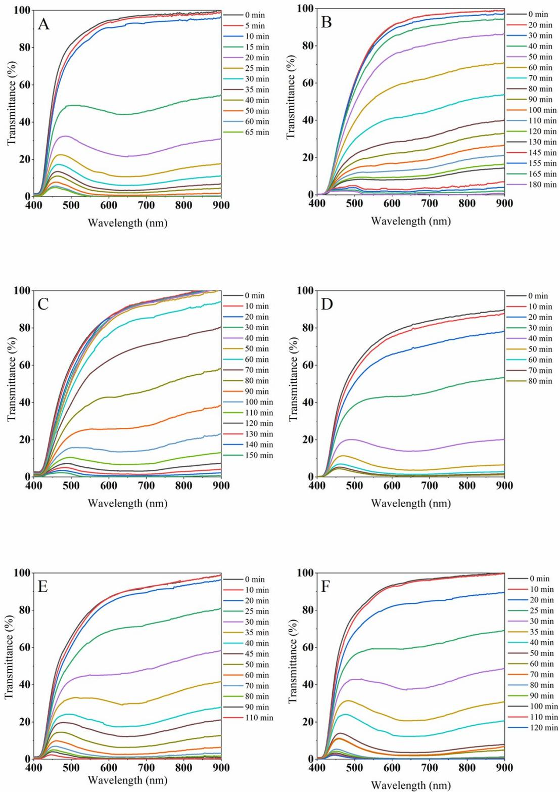
**Figure S2.** Transmittance spectra in the 400-900 nm part of the spectra during UV irradiation for TiO<sub>2</sub> NPs in different solvents. A) Ethanol; B) *n*-Propanol; C) *i*-Propanol; D) *n*-Butanol; E) *n*-Pentanol; F) *n*-Hexanol.
