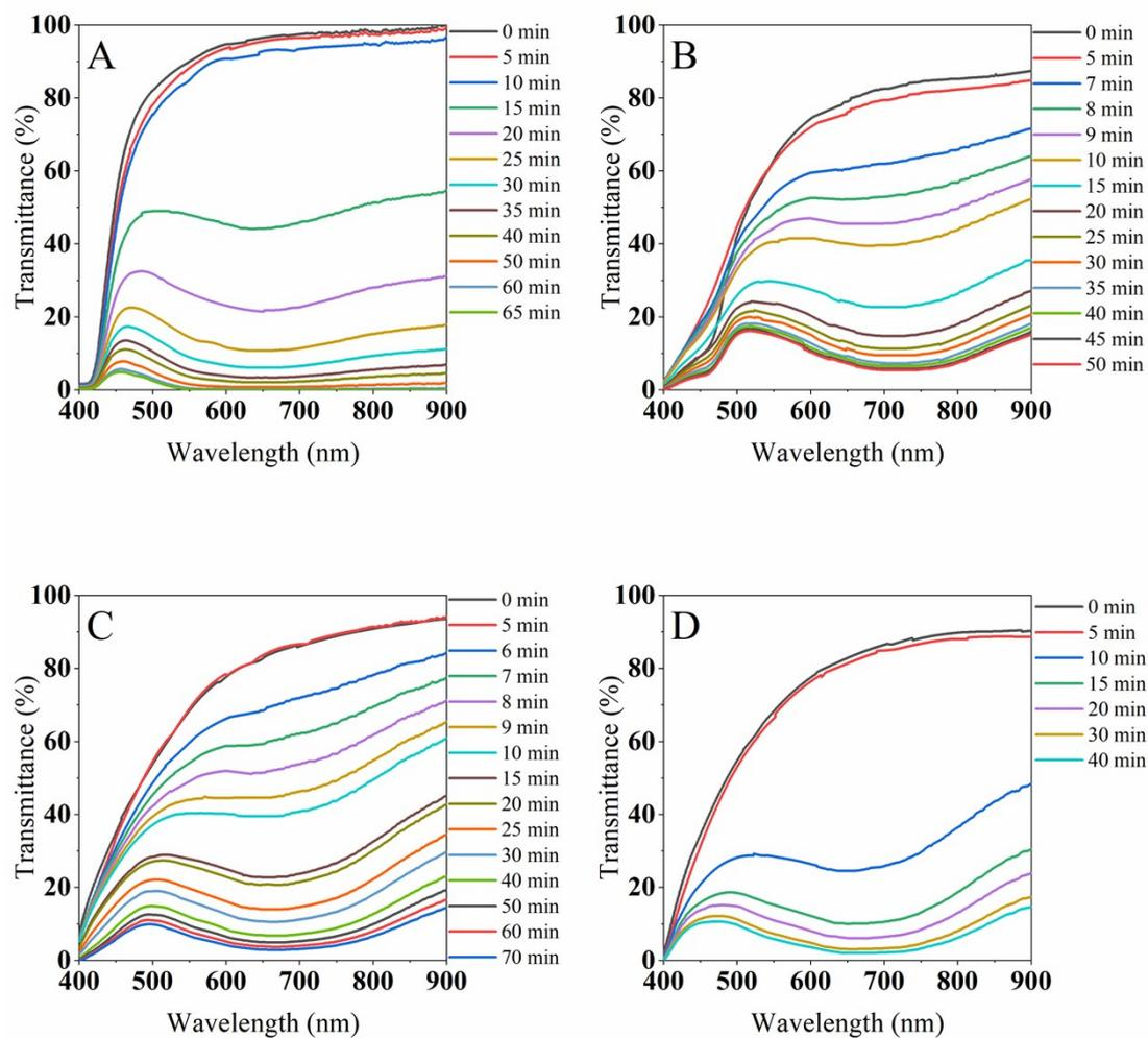
**Figure S3.** Transmittance spectra in the 400-900 nm part of the spectra during UV irradiation for  $\text{TiO}_2$  NPs in ethanol and with different hole scavenger additions. A) Pure ethanol; B) 50 mol% of MEA; C) 50 mol% DEA; D) 50 mol% TEA.
