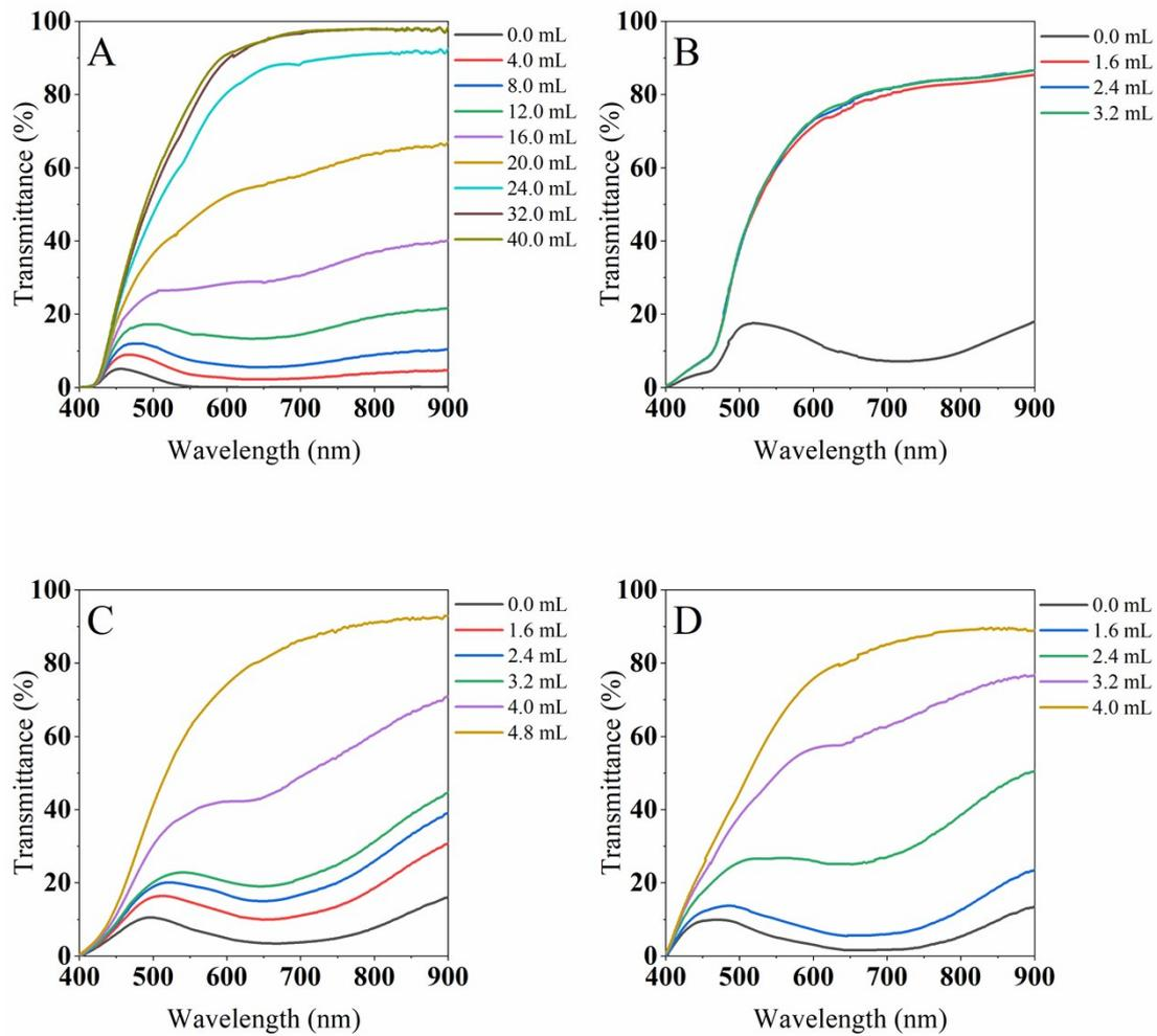
**Figure S6.** Transmittance spectra in the 400-900 nm part of the spectra during recovery with air injection for TiO<sub>2</sub> NPs in ethanol and with different hole scavenger additions. A) Pure ethanol; B) 50 mol% of MEA; C) 50 mol% DEA; D) 50 mol% TEA.
