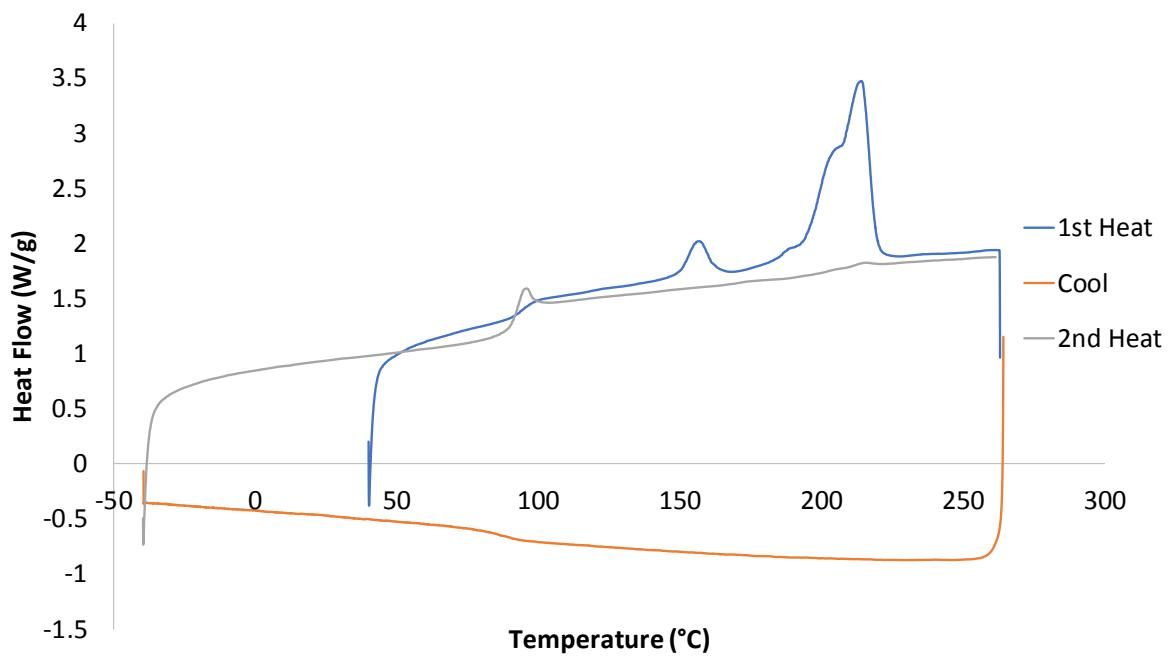
**Fig. S8** DSC thermogram of heat-cool-heat cycle of 4,4'-BCD homopolymer after oven annealing of melt compressed film at 145 °C for 1h. Film Sample. Heating and cooling cycles conducted at a ramp rate of 10 °C min<sup>-1</sup>.
