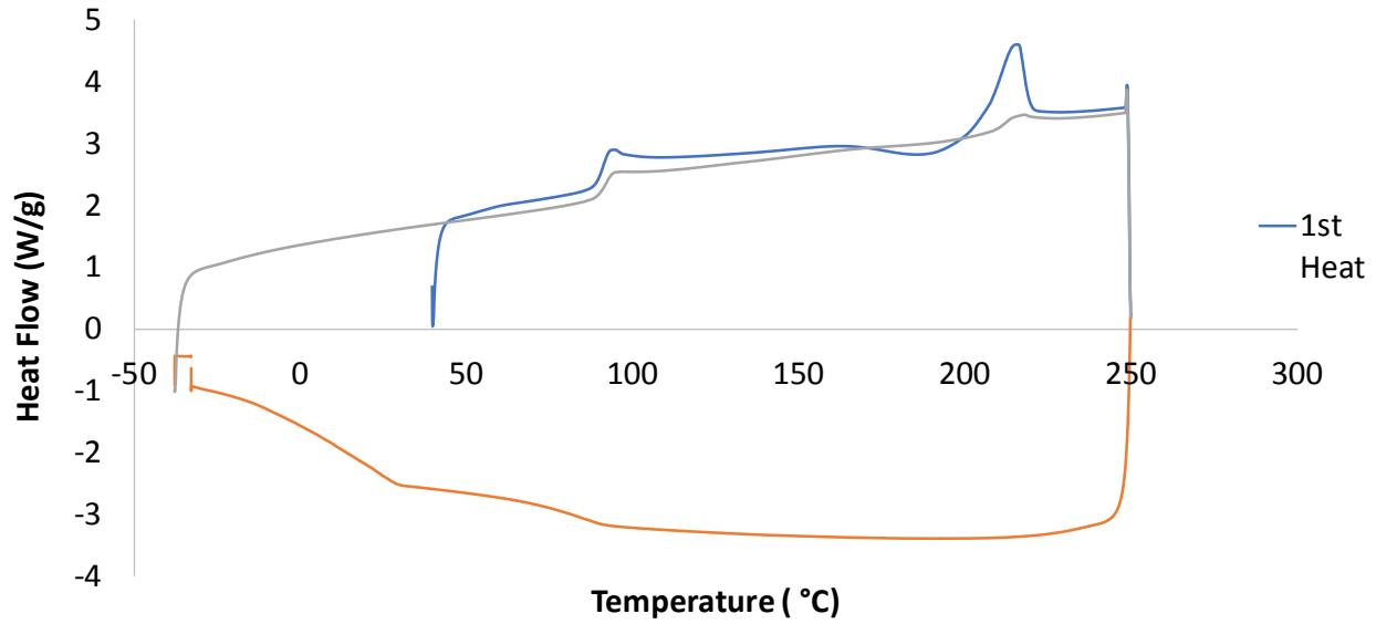
**Fig. S7** DSC thermogram of heat-cool-heat cycle of 4,4'-BCD homopolymer after compression into a film. Film Sample. Heating and cooling cycles conducted at a ramp rate of  $10\text{ }^{\circ}\text{C min}^{-1}$ .
