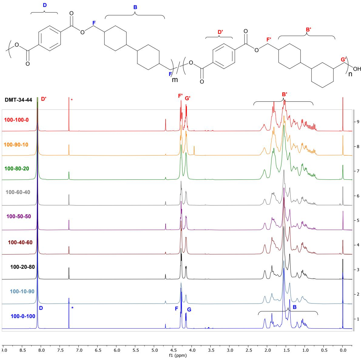
**Fig. S1**  $^1\text{H}$  NMR spectra of poly(bicyclohexyldimethylene terephthalate) polyester series. \* -  $\text{CDCl}_3$
