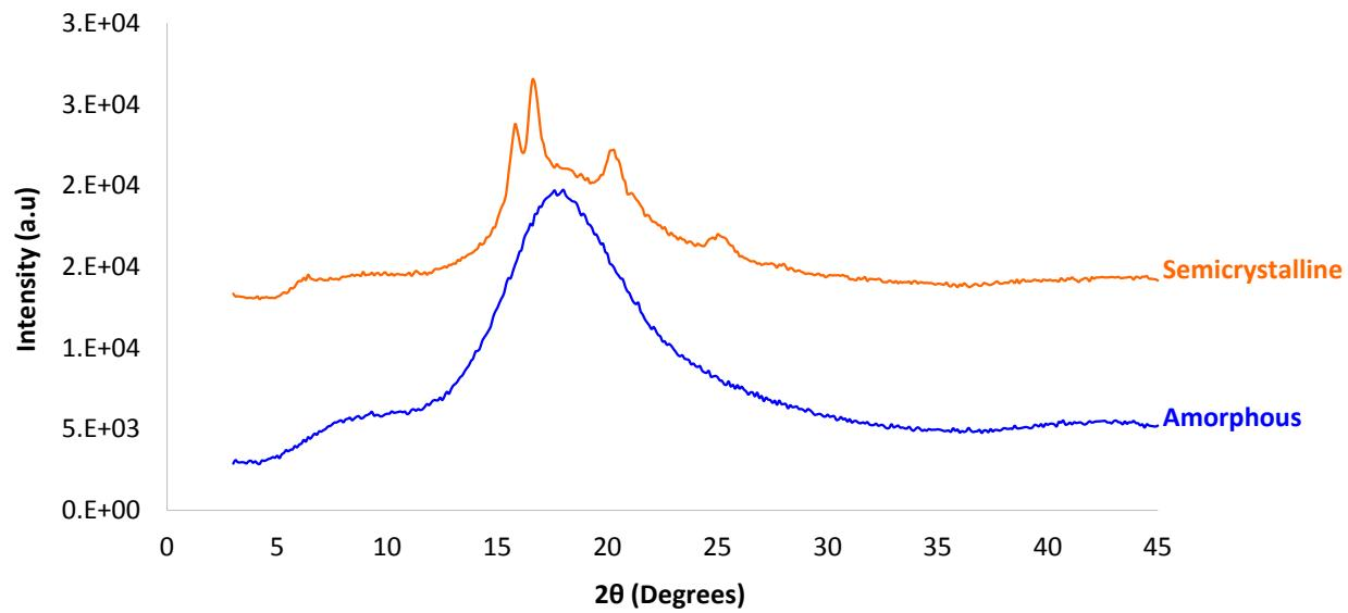
**Fig. S5** X-ray diffraction patterns of amorphous and semicrystalline 4,4'-BCD homopolymer.
