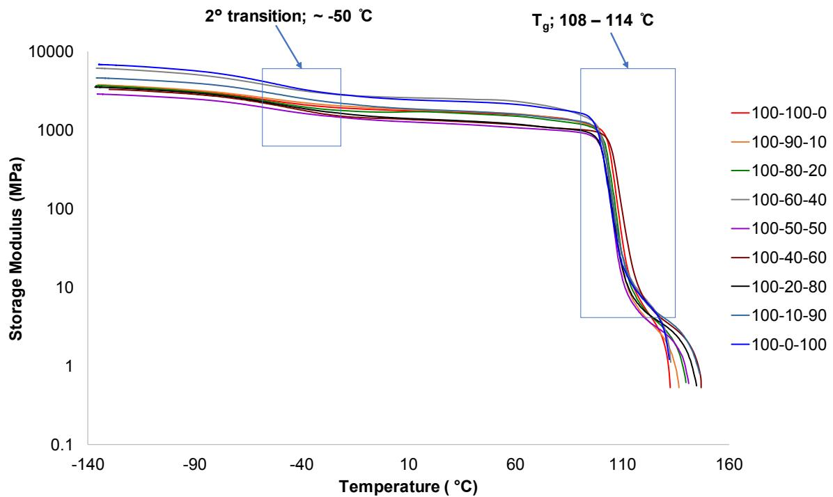
**Fig. S3** DMA storage modulus vs. temperature thermogram of poly(bicyclohexyldimethylene terephthalate) polyester series at a ramp rate of  $3\text{ }^{\circ}\text{C min}^{-1}$  from  $-140$  to  $150\text{ }^{\circ}\text{C}$  at an oscillation amplitude of  $15\text{ }\mu\text{m}$  and a frequency of  $1\text{Hz}$ .
