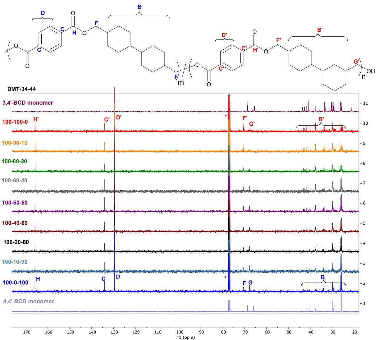
**Fig. S2**  $^{13}\text{C}$  NMR spectra of poly(bicyclohexyldimethylene terephthalate) polyester series. \* -  $\text{CDCl}_3$
