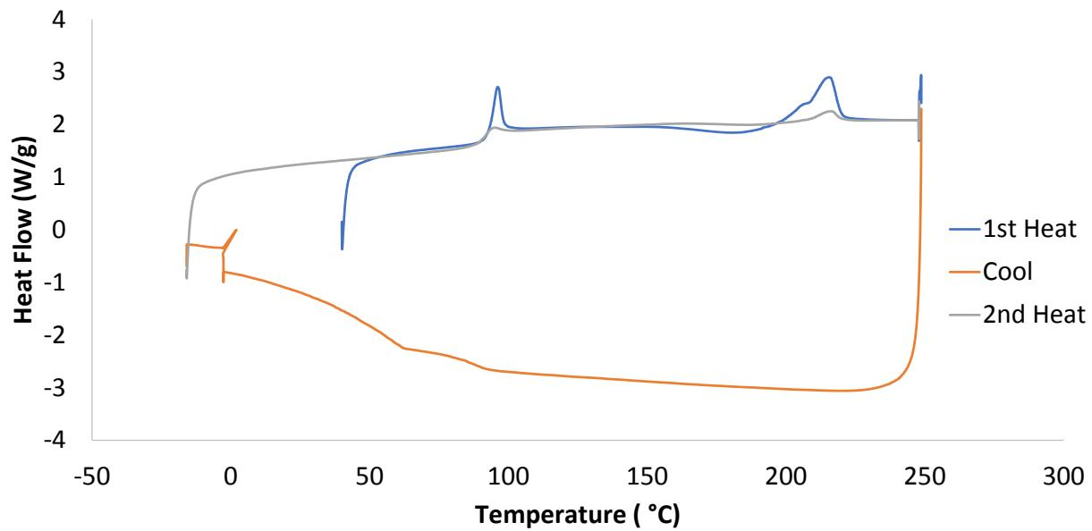
**Fig. S6** DSC thermogram of heat-cool-heat cycle of 4,4'-BCD homopolymer after synthesis. Samples in ground state. Heating and cooling cycles conducted at a ramp rate of  $10\text{ }^{\circ}\text{C min}^{-1}$ .
