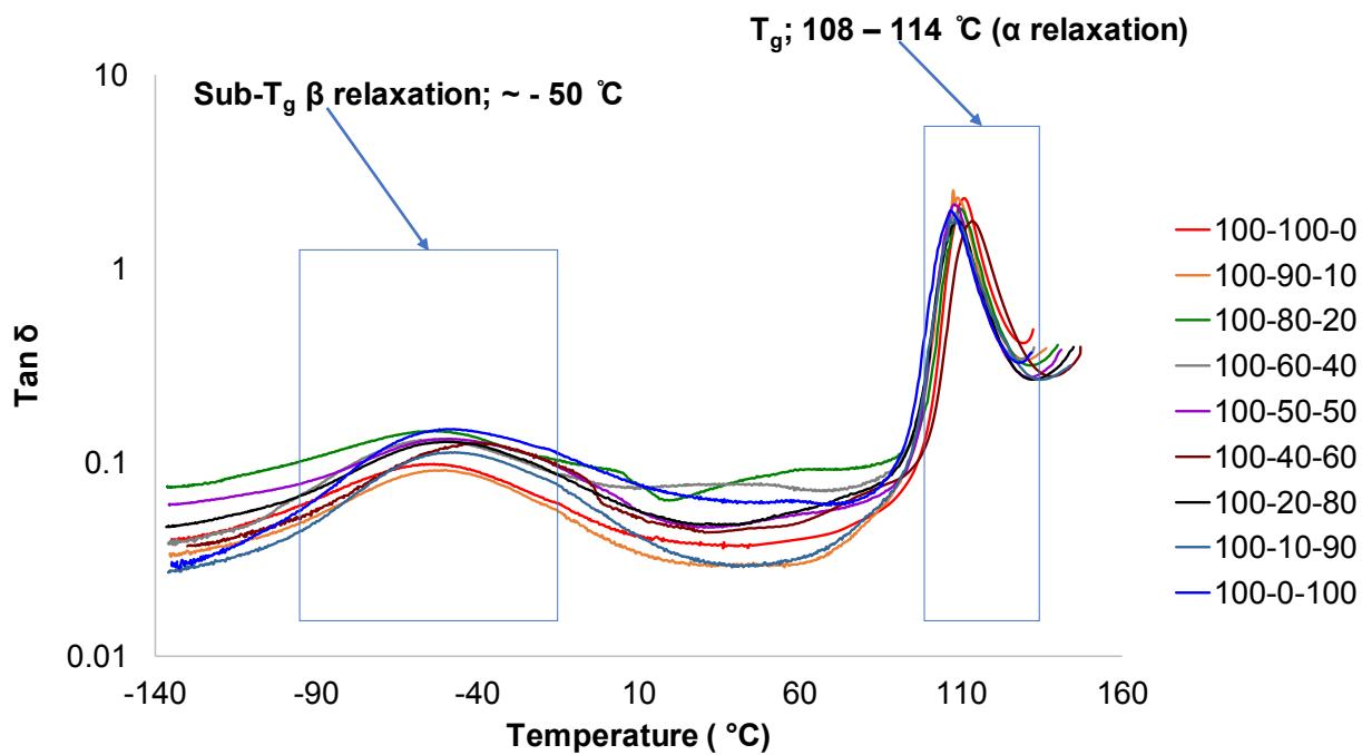
**Fig. S4** DMA  $\tan \delta$  vs. temperature thermogram of poly(bicyclohexyldimethylene terephthalate) polyester series at a ramp rate of 3  $^{\circ}\text{C}$  min $^{-1}$  from -140 to 150  $^{\circ}\text{C}$  at an oscillation amplitude of 15  $\mu\text{m}$  and a frequency of 1Hz.
