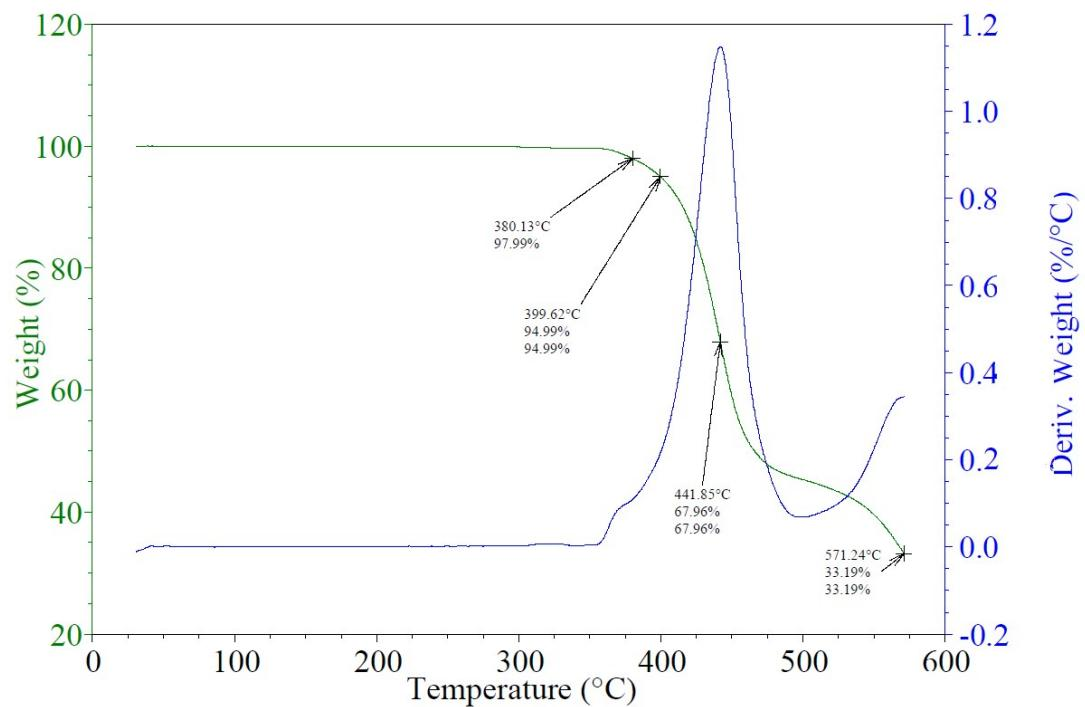
Fig. S4: Thermogravimetric analysis under air and heating at 10 °C/min for Entry 10, Table 1.
