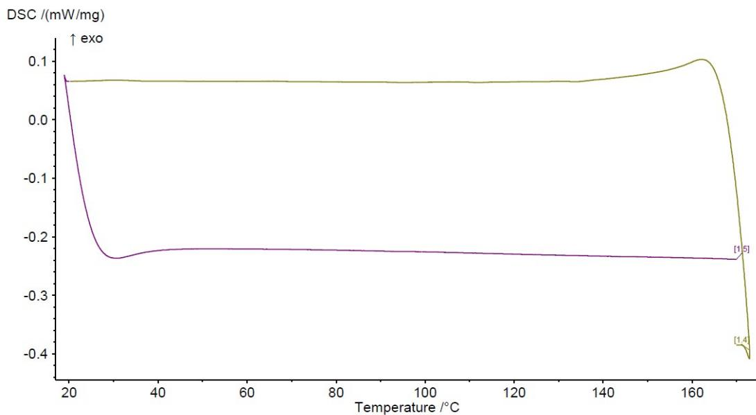
Fig S.6: Differential Scanning Calorimetry thermogram for Entry 5, Table 1. First cooling and second heating program.
