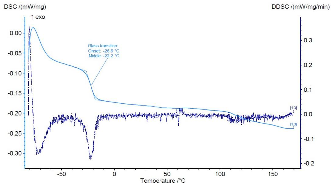
Fig. S8: Differential Scanning Calorimetry thermogram for Entry 6. First cooling and second heating program for  $T_g$  determination.
