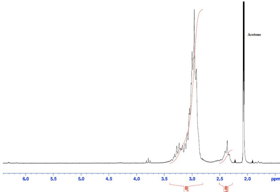
Fig. S1: <sup>1</sup>H NMR spectrum of poly(VDF-*co*-PMVE) copolymer (Entry 2, Table 1).
