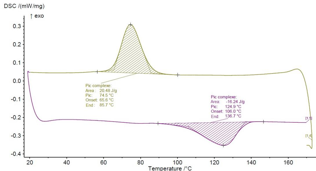
Fig S.5: Differential Scanning Calorimetry thermogram for Entry 2, Table 1. First cooling and second heating program.
