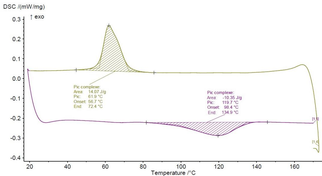
Fig S.7: Differential Scanning Calorimetry curve for Entry 9, Table 1. First cooling and second heating program for  $T_m$  and  $T_c$  and  $\Delta H_m$  and  $\Delta H_c$  determination.
