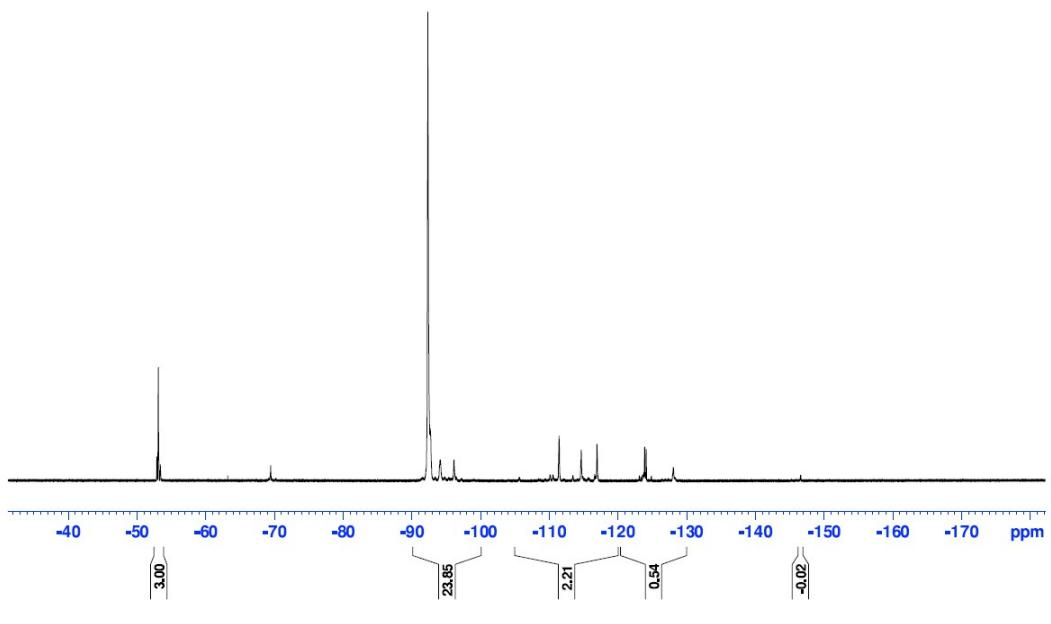
Fig. S2:  $^{19}\text{F}$  NMR spectrum of poly(VDF-*co*-PMVE) copolymer (Entry 2, Table 1)
