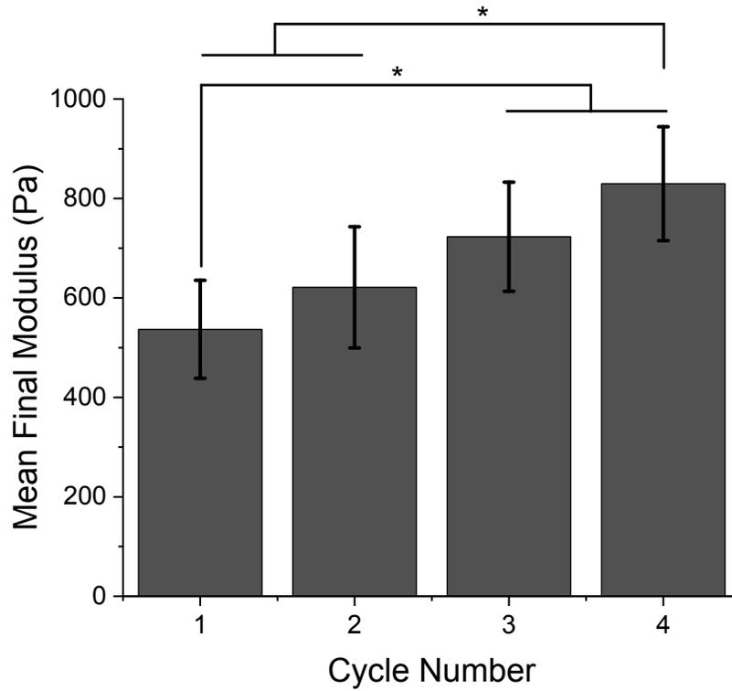
**Supporting Figure S3.** The mean final storage modulus of CNA/DNA gels after 3 heat/cool cycles shows a stiffening of the gel with each cycle number. Gels were made at 5% w/v 8PEG-T, 1:1 A:T ratio, and 20% H<sub>2</sub>O in DMSO. One cycle refers to a temperature ramp to 70°C followed by a cooling to 22°C and equilibration for 20 minutes. Statistical significance is denoted by \* (p<0.05).
