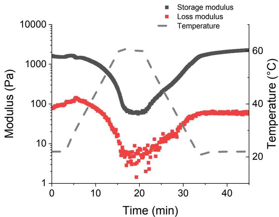
**Supporting Figure S4.** Temperature sweep data from 22°C to 60°C showing that at 60°C, the gel does not melt, indicating melting temperatures are higher than 60°C.
