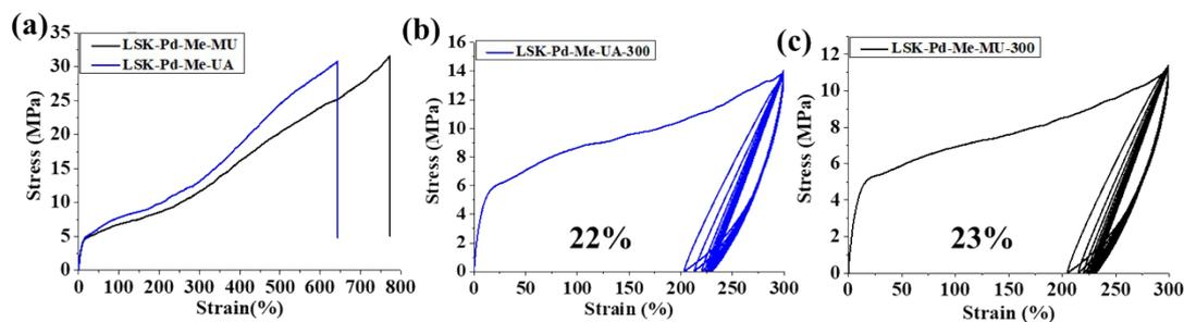
Figure S78. Stress-strain curves for E-UA and E-MU generated by Pd2 (Table 3, entries 2 and 6) (a); Plots of hysteresis experiments of ten cycles at a strain of 300% for samples generated by Pd2 (b-c) (Table 3, entries 2, 6)
