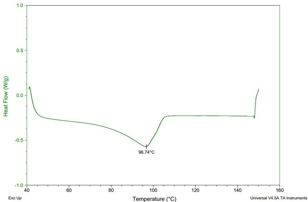
Figure S59. DSC of the polymer from table 2, entry 2.
