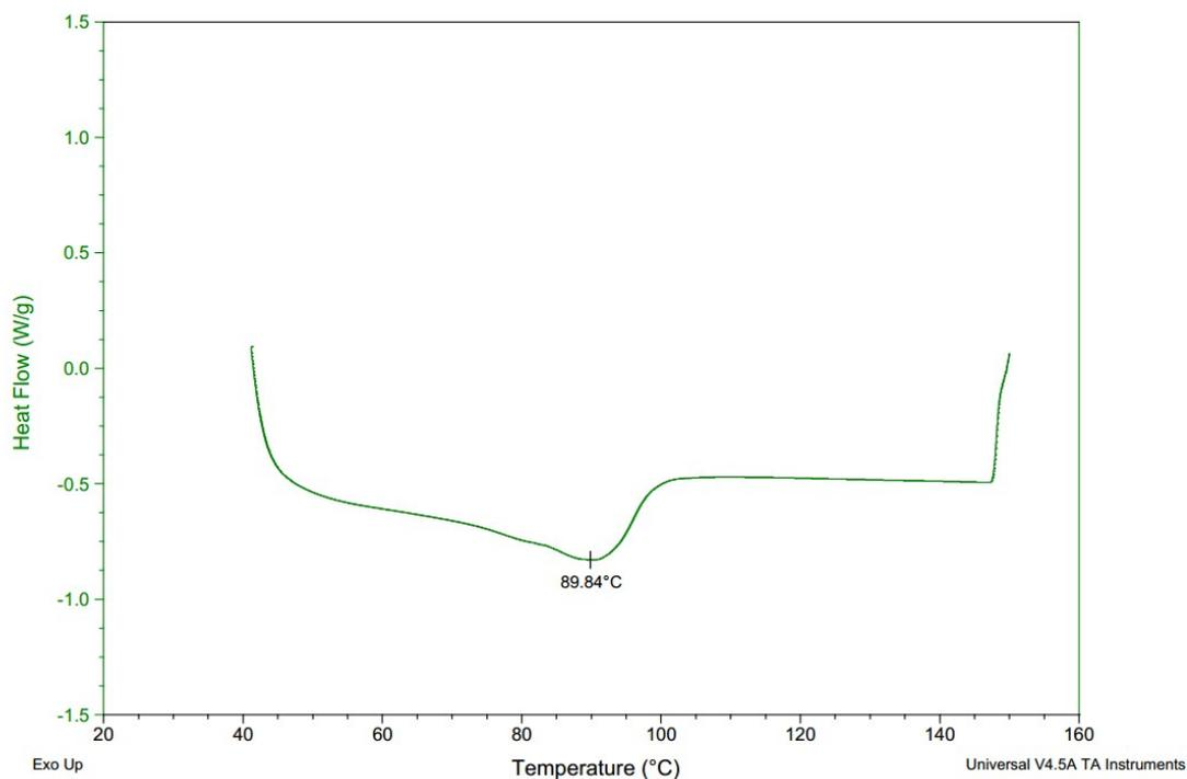
Figure S66. DSC of the polymer from table 3, entry 6.
