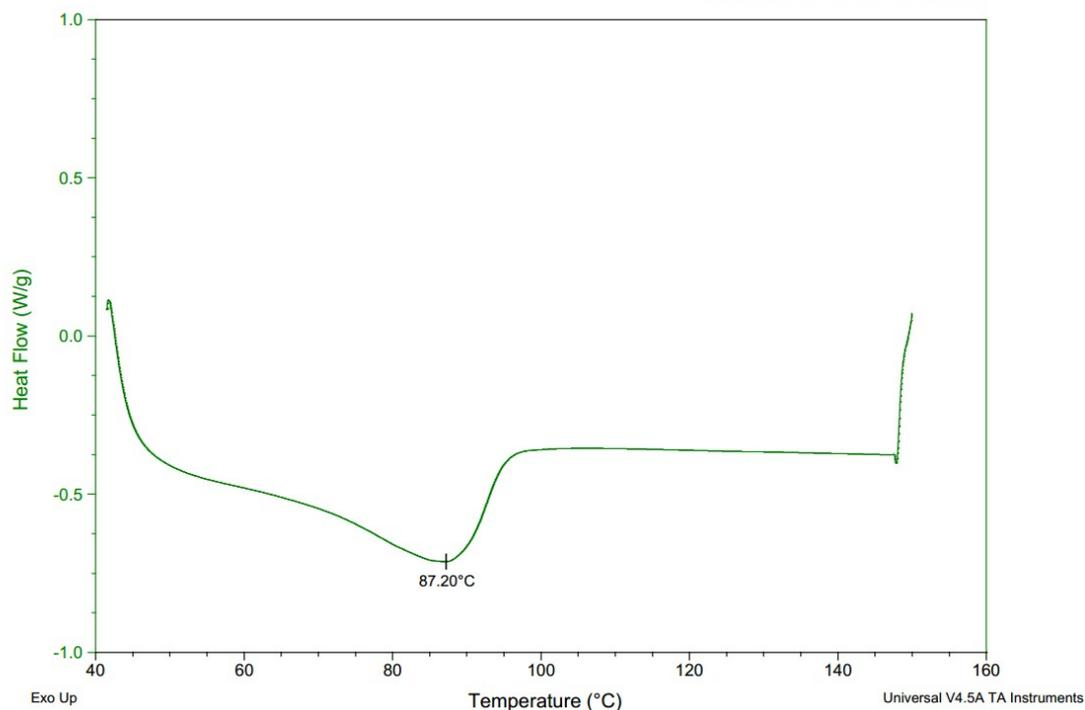
Figure S61. DSC of the polymer from table 1, entry 4.
