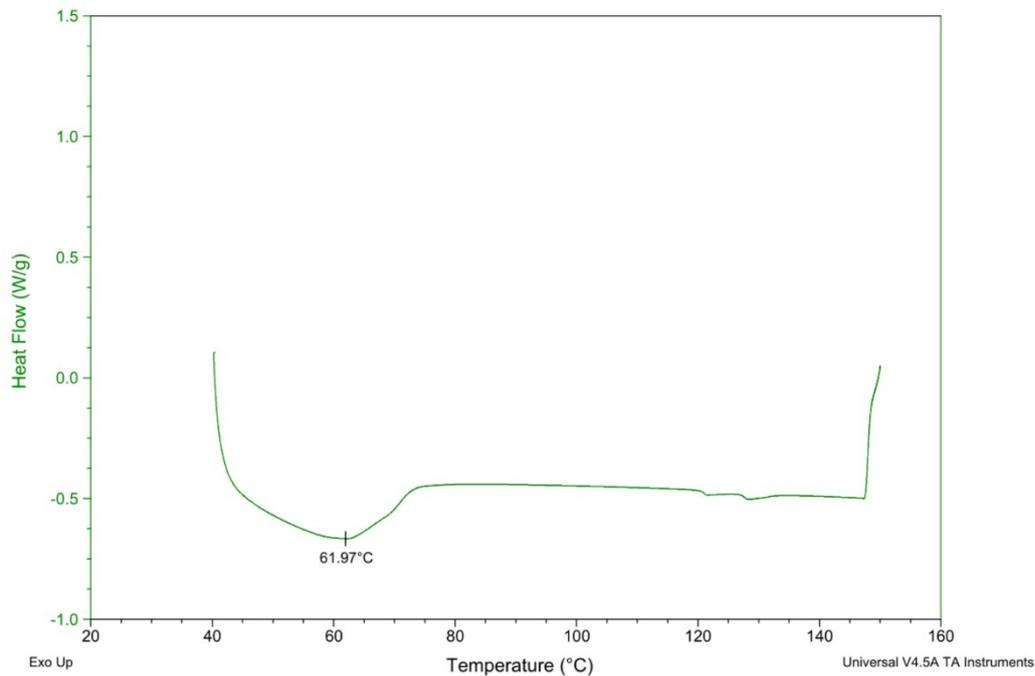
Figure S57. DSC of the polymer from table 1, entry 11.
