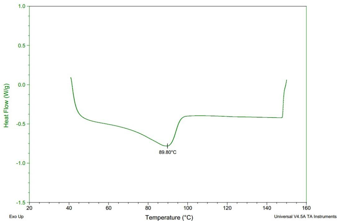
Figure S60. DSC of the polymer from table 1, entry 3.
