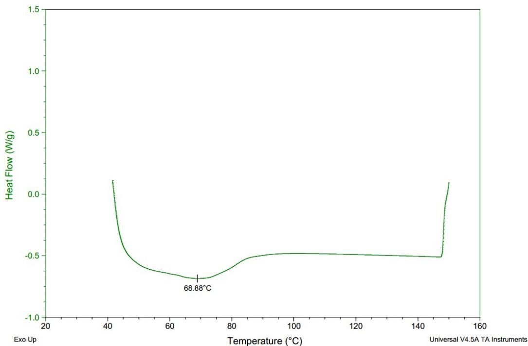
Figure S62. DSC of the polymer from table 3, entry 1.
