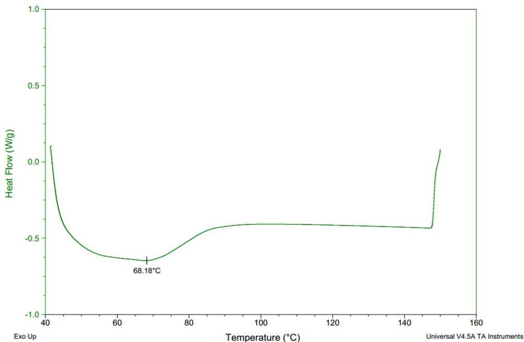
Figure S65. DSC of the polymer from table 3, entry 5.
