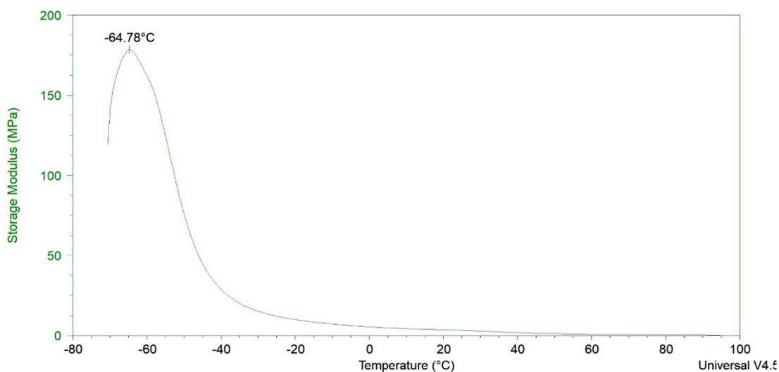
Figure S68. DMA of the polymer from table 1, entry 3.
