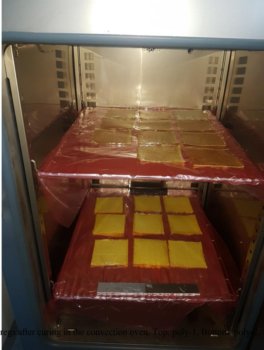
**Figure S9.** Prepregs after curing in the convection oven. Top: poly-1, Bottom: poly-2.
