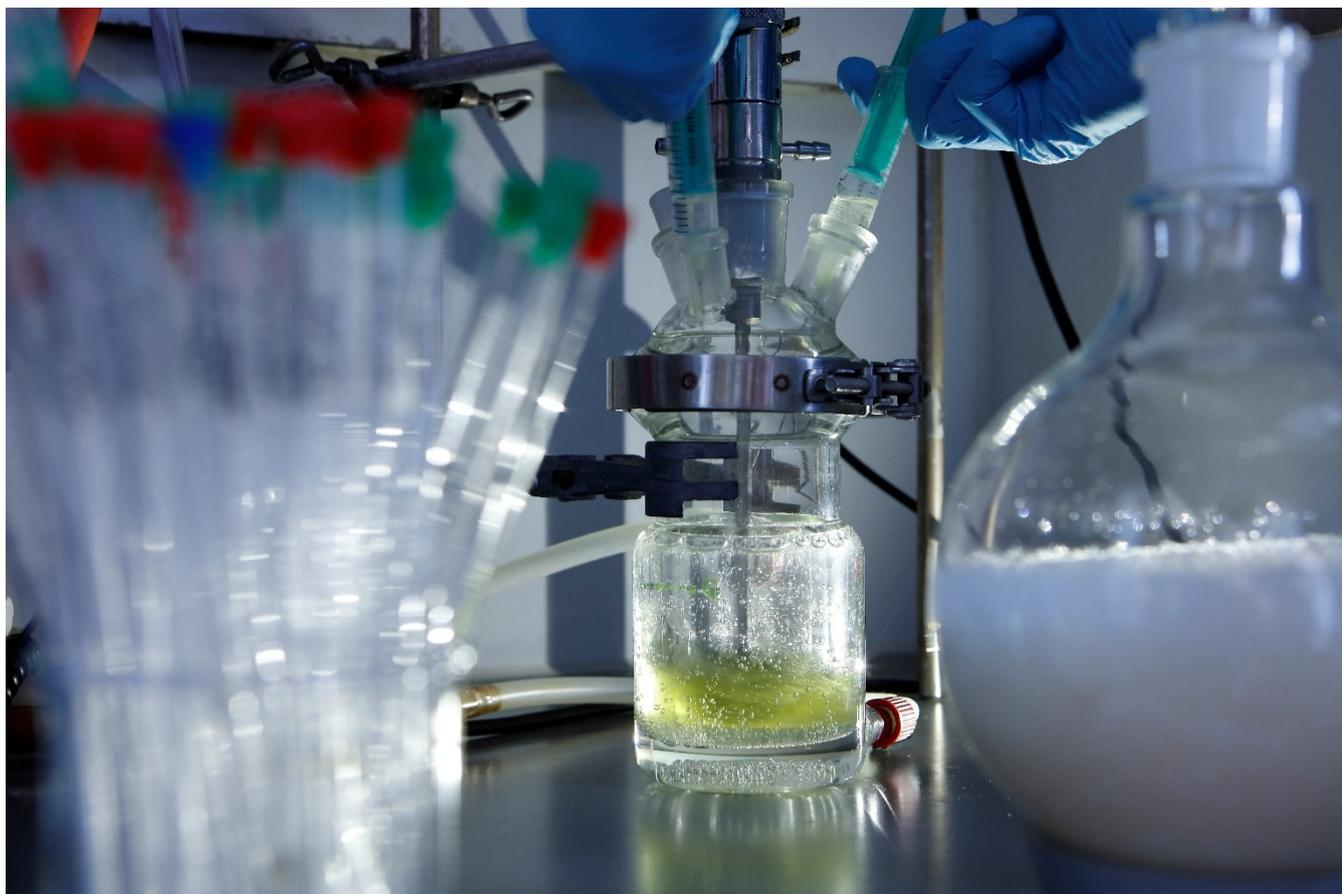
**Figure S10.** Preparation of a vitrimer in a heated glass-reactor.
