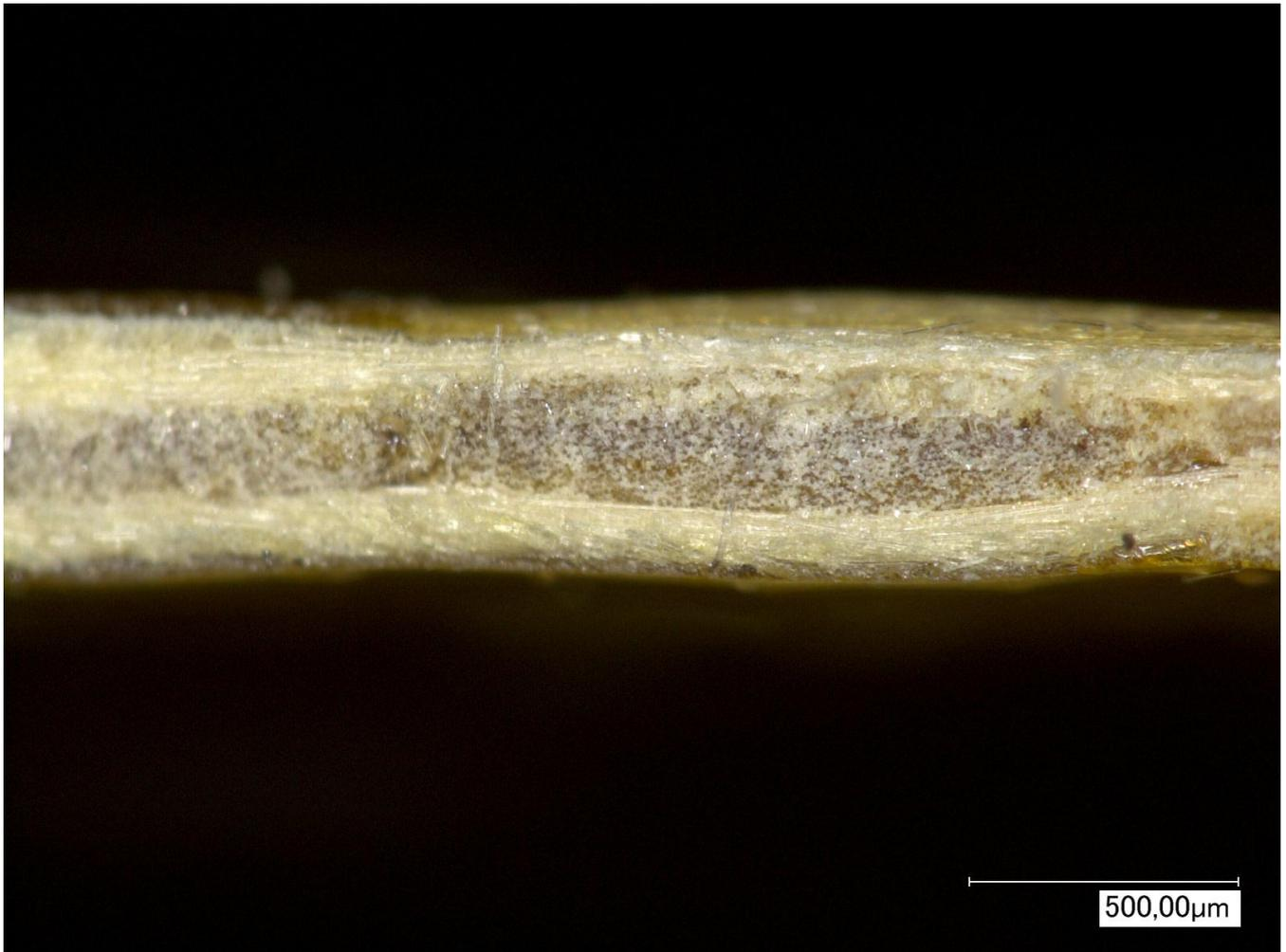
**Figure S16.** Microscope image after hot pressing two prepreg layers of poly-2 with a 0.3 mm gap at 150 °C and 10 kN for 1 h.
