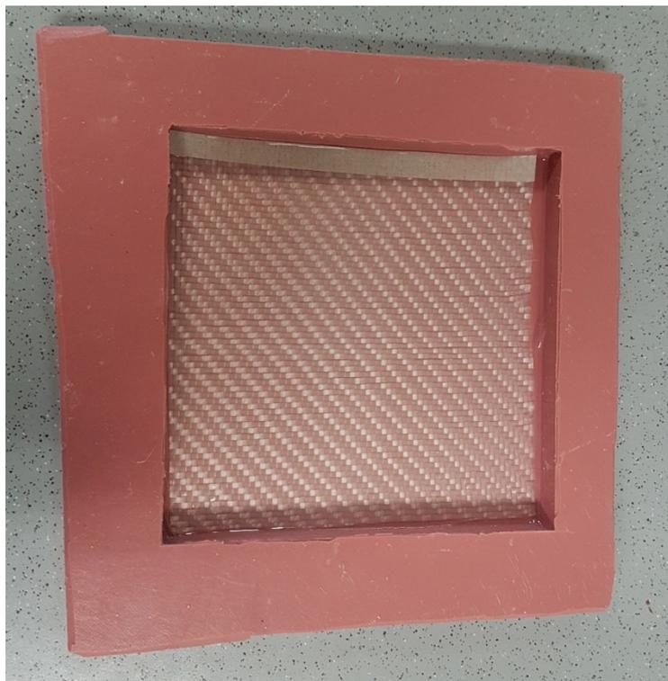
**Figure S8.** Silicone mold used for the preparation of the composites.
