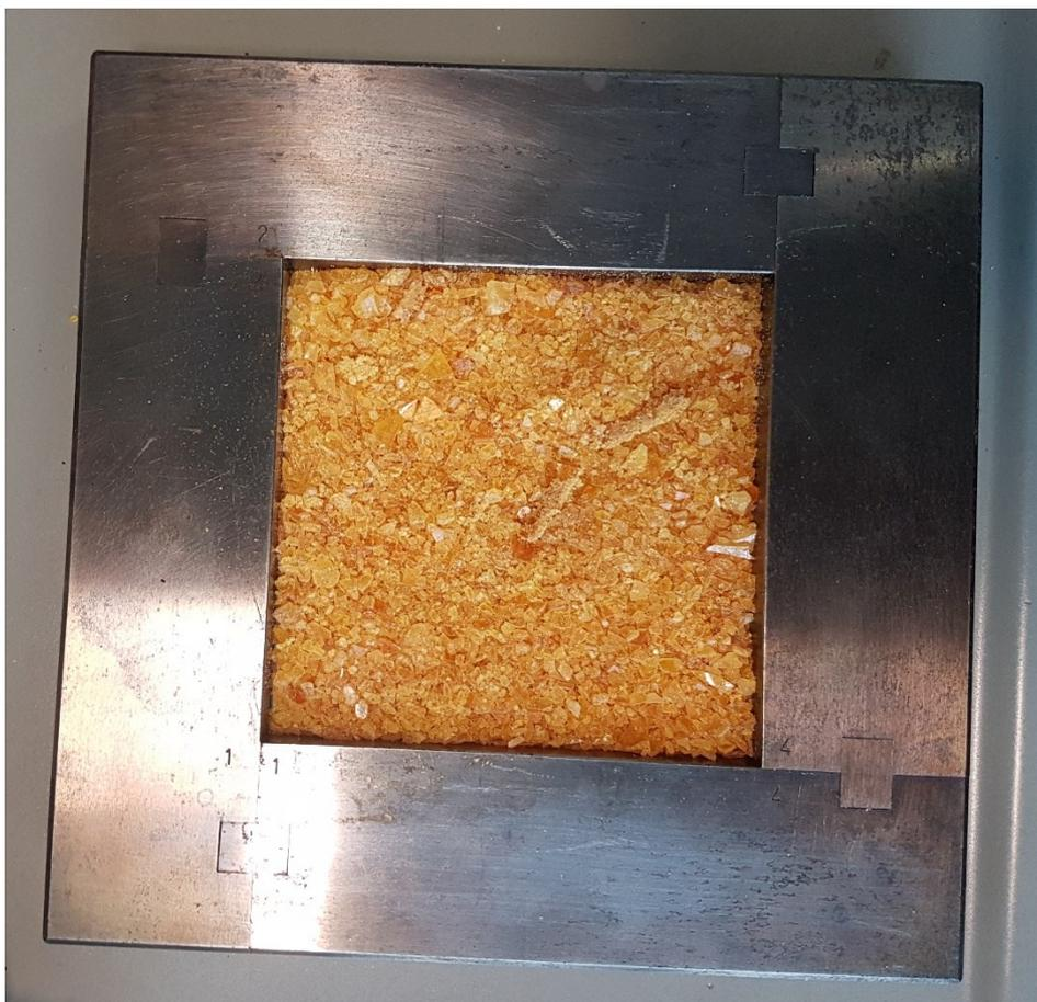
**Figure S14.** Preparation of 12 x 12 mm<sup>2</sup> cone plates: Poly-1 powder in a steel mold.
