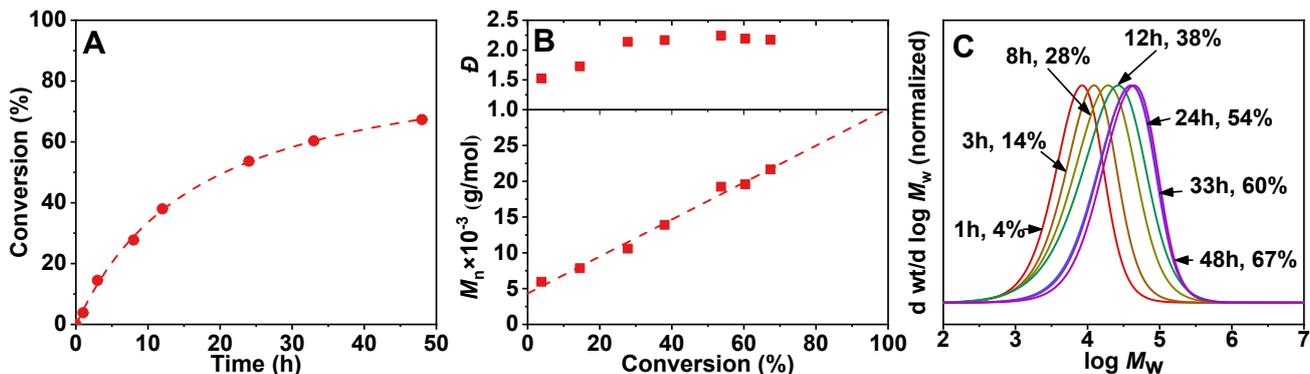
**Fig. S2.** Results of the polymerization of *t*BMA mediated by TfXT in toluene at 65 °C: plots of conversion of *t*BMA vs. time (A), plots of  $M_n$  &  $D$  vs. conversion of *t*BMA (B) and GPC-derived differential molecular weight distribution curves (C). Concentration of *t*BMA: 30 wt%; *t*BMA/ABVN/TfXT = 200/1/5.
