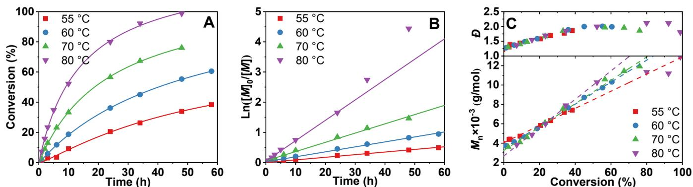
**Fig. S1.** Results of the polymerization of MMA mediated by TfXT with ABVN/TfXT = 1/2 in toluene at different temperatures: Plots of MMA conversion vs. time (A), polymerization kinetics (B), and plots of  $M_n$  &  $\bar{D}$  vs. conversion of MMA. Concentration of MMA: 30 wt%; MMA/ABVN = 100/1.
