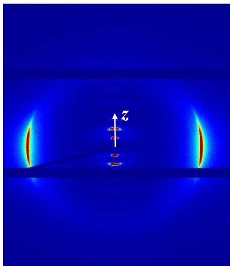
**Fig. S5** 2D XRD pattern of the stretched film sample of **P8-6-E**. The z-axis is stretching direction.
