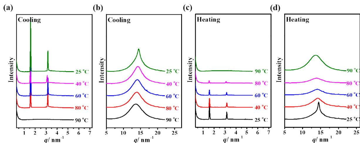
**Fig. S11** 1D XRD profiles of **P8-6-E** recorded at various temperatures upon (a, b) cooling and (c, d) subsequent heating. (a) and (c), low angle region; (b) and (d), high angle region.
