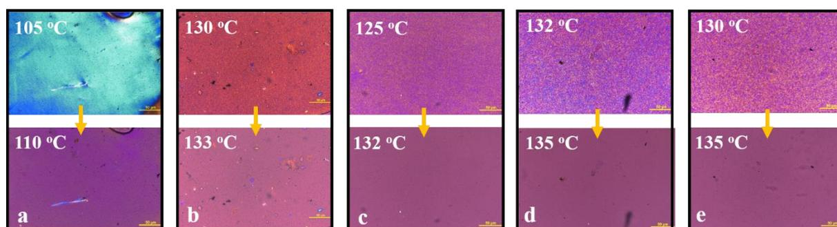
**Fig. S7** Isotropic transition of **P8-ns** observed under POM upon heating. (a) **P8-2**; (b) **P8-4**; (c) **P8-6**; (d) **P8-8**; (e) **P8-10**.
