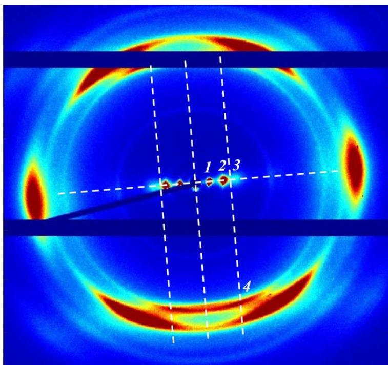
**Fig. S3** 2D XRD pattern of stretched film sample of **P8-10**. The dotted white lines are parallel or perpendicular to the stretching direction for indexation.
