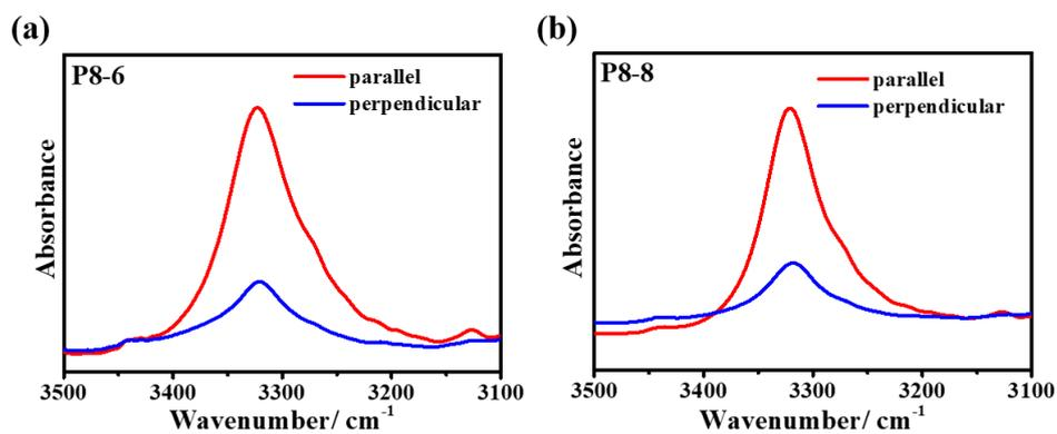
**Fig. S13** Polarized FT-IR spectra of the oriented films of (a) **P8-6**; (b) **P8-8**. The red and blue curves represent the data measured with polarizer parallel and perpendicular to the stretching direction, respectively.
