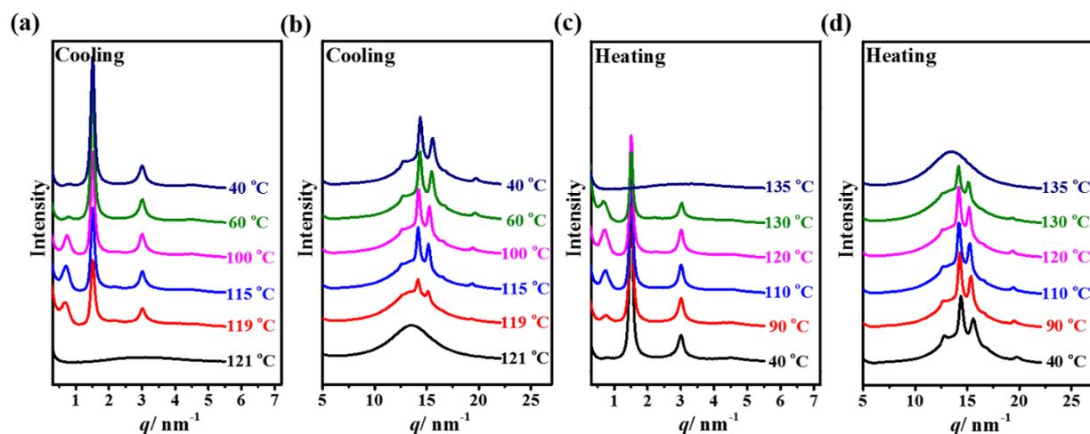
**Fig. S9** 1D XRD profiles of **P8-8** recorded at various temperatures upon (a, b) cooling and (c, d) subsequent heating. (a) and (c), low angle region; (b) and (d), high angle region. It is noted that upon relatively fast cooling some residual diffraction at  $0.5q^*$  could be seen at low temperatures. However, it would disappear after thermal annealing.
