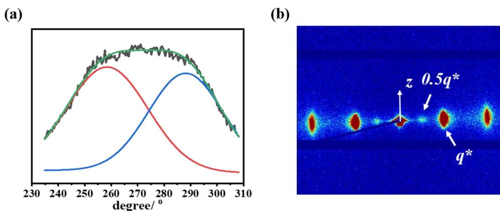
**Fig. S4** (a) Azimuthal integration (black line) of spot 4 of P8-6 and peak separation of this peak (red and blue line); (b) 2D XRD pattern of the low angle region of the stretched film sample of **P8-6**. The  $z$ -axis is stretching direction.
