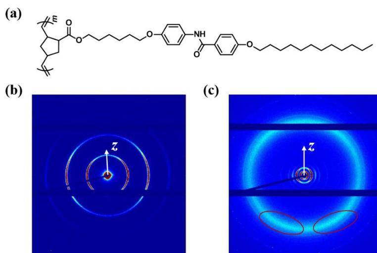
**Fig. S12** (a) Chemical structure of **P12-6**; (b) and (c), 2D XRD patterns of the stretched film sample of **P12-6** recorded at room temperature. (b) shows the low angle diffractions. The oriented film was obtained by melt drawing. z direction is the stretching direction.
