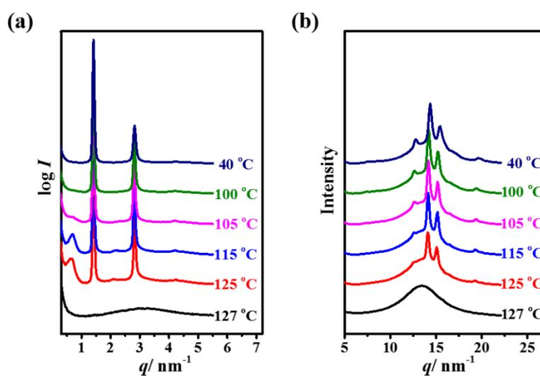
**Fig. S8** 1D XRD profiles of **P8-10** recorded at various temperatures during cooling. (a) and (b), low angle and high angle region, respectively.
