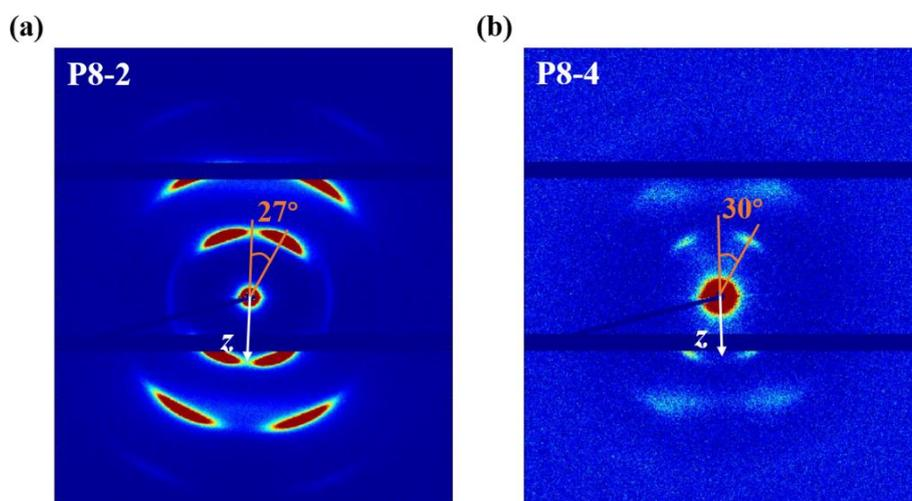
Fig. S2 2D XRD patterns of the low angle region of stretched film samples of (a) **P8-2** and (b) **P8-4** recorded at room temperature. The z-axis is stretching direction.
