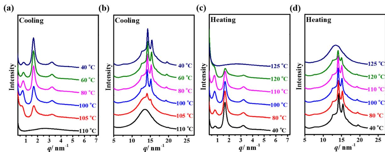
**Fig. S10** 1D XRD profiles of **P8-6** recorded at various temperatures upon (a, b) cooling and (c, d) subsequent heating. (a) and (c), low angle region; (b) and (d), high angle region.
