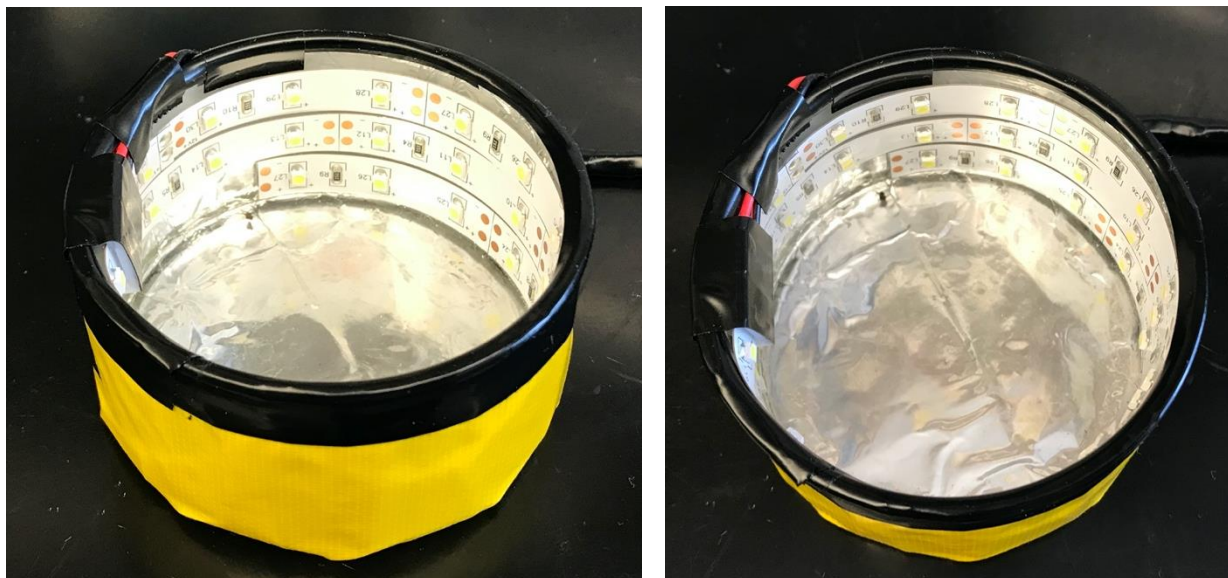
Figure S5. Photographs of the LED wells constructed with more light strips. These reactors were built by wrapping an 80 mm x 40 mm recrystallization dish with aluminum foil and wrapping uncoated white LED strips (15 LED segments) around the inside of the dish. The photographs provide a side view (left) and top view (right).
