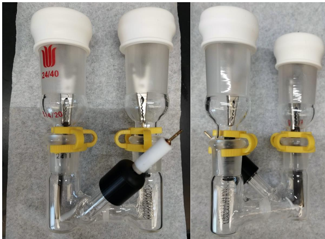
Figure S1. Photographs of the U-cell used in this work. (Left) Front side of the cell, showing the working electrode compartment on the left side, with a glassy carbon working electrode and reference electrode inserted in the side-arm. In the center, an extra-fine glass frit acts as a separator
