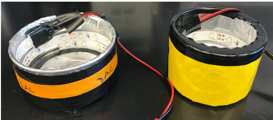
Figure S7. Photograph comparing the original light well used in this work (left, dimensions: 80 x 40 with 9 LED segments) and that constructed to move the LEDs closer to the reaction vessel (right, dimensions: 70 x 50 with 9 LED segments).
