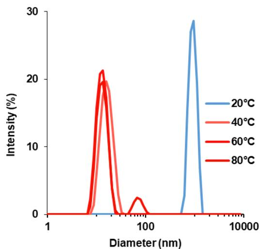
**Figure S11.** Overlay of DLS profiles of sample 11 (Table 1) at 1 wt% in water upon heating from 20 to 80 °C.
