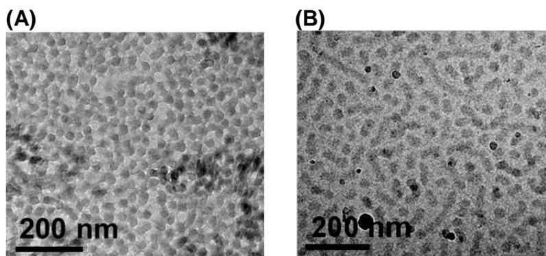
**Figure S15.** Representative cryo-TEM images of sample 16: (A) heated at ~10 wt% to 70 °C, then diluted at 1 wt% at 70 °C and analyzed after deposition at 70 °C; (B) heated at ~10 wt% to 70 °C, then cooled to room temperature and diluted at 1 wt%.
