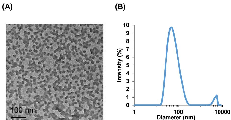
**Figure S10.** (A) Representative TEM image prepared at 0.03 wt% stained with phosphotungstic acid at 25 °C and (B) final size distribution determined by DLS prepared at 0.03 wt% at 25 °C of the aqueous solution PDMAc-*b*-P(AAm-*co*-AN) (Entry 10, Table 1).
