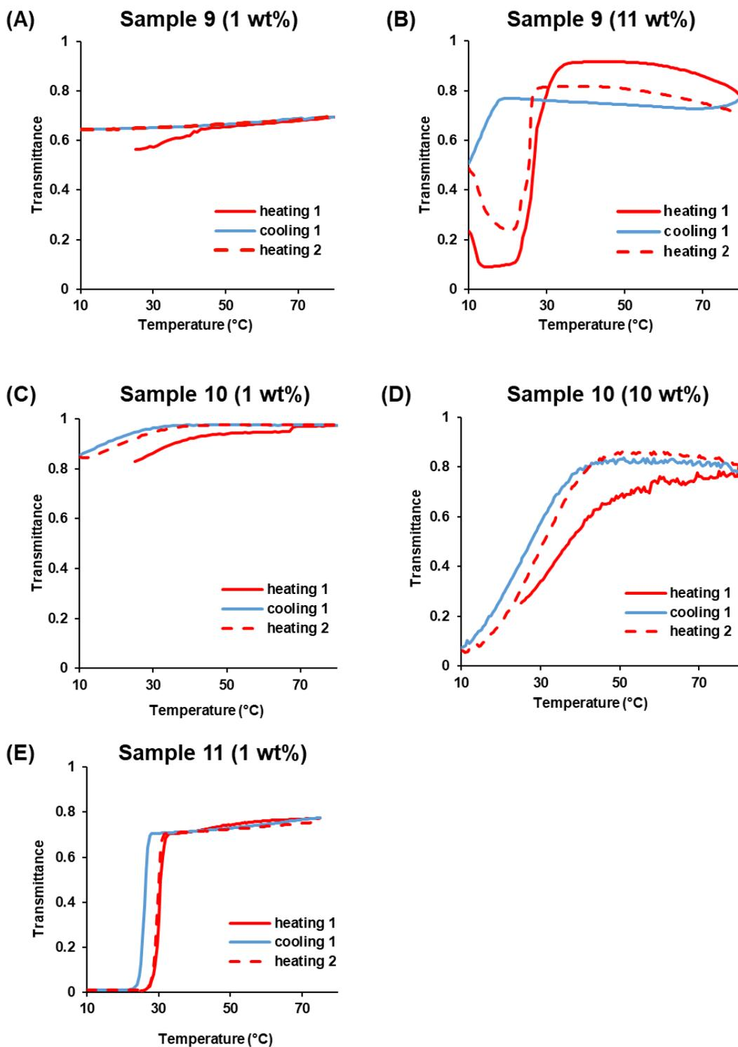
**Figure S9.** Turbidimetry measurements (first heating, first cooling and second heating) of PDMAc-*b*-P(AAm-co-AN) dispersions (Samples 9, 10 and 11 in Table 1).
