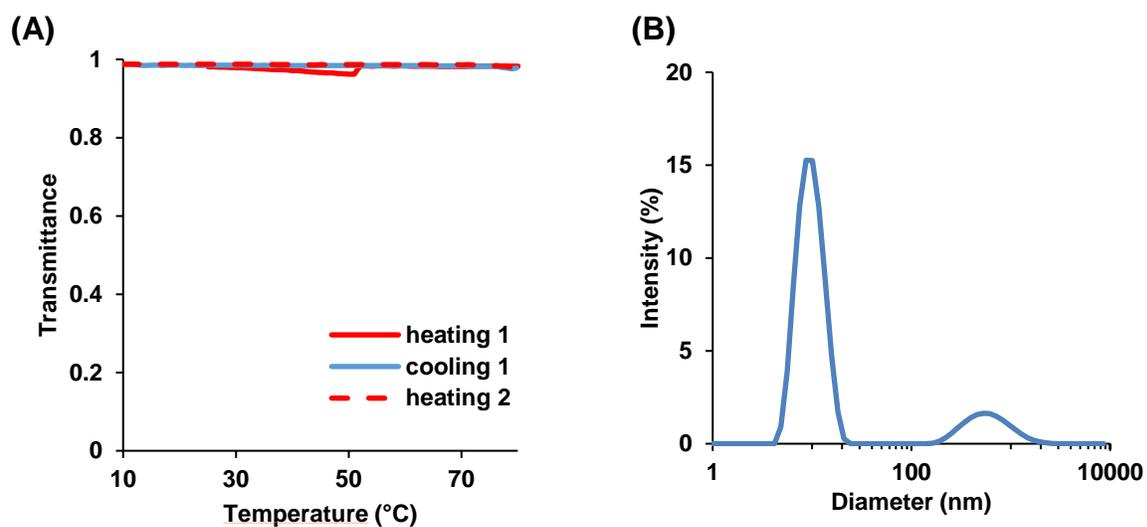
**Figure S8.** (A) Turbidimetry measurements (first heating, first cooling and second heating) of PDMAc-*b*-P(AAm-*co*-AN) dispersion prepared at 1 wt% (Entry 8, Table 1) and (B) size distribution determined by DLS at 25 °C.
