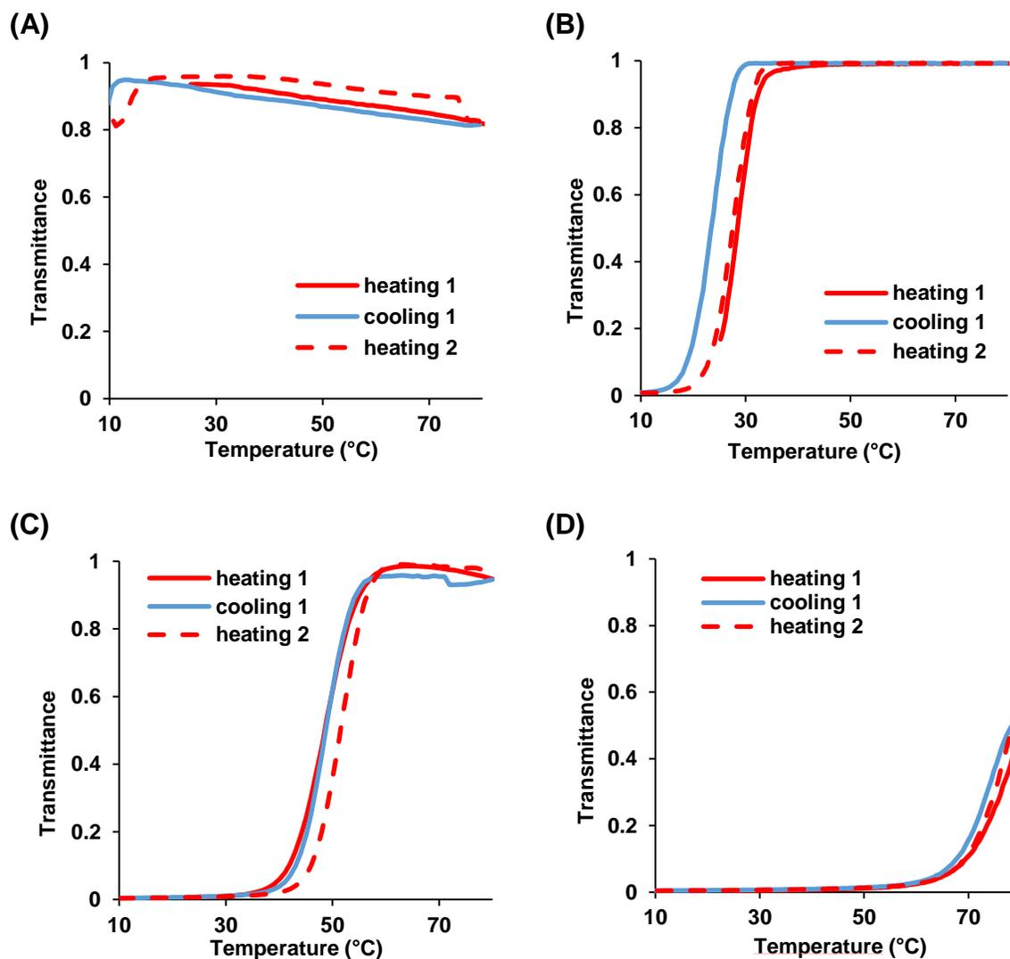
**Figure S3.** Turbidity curves (first heating, first cooling and second heating) of P(AAm-co-AN) dispersions at 0.2 wt% with different copolymer compositions : (A)  $F_{AN} = 0.32$  (Table S1, entry 2), (B)  $F_{AN} = 0.40$  (Table S1, entry 3), (C)  $F_{AN} = 0.43$  (Table S1, entry 4) and (D)  $F_{AN} = 0.52$  (Table S1, entry 5).
