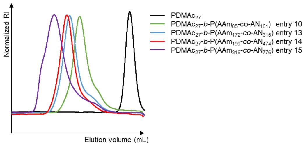
**Figure S12.** Normalized size exclusion chromatograms of PDMAc macroRAFT agent and the resulting PDMAc-*b*-P(AAm-*co*-AN) block copolymers prepared by copolymerization of AAm and AN in water at 45 °C with a constant initial  $f_{AN}$  of 0.65 targeting various DP.
