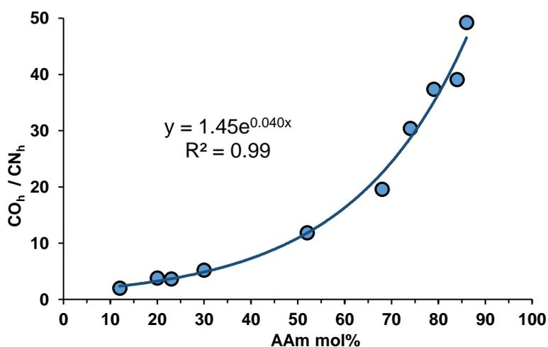
**Figure S1.** Calibration curve used for the determination of the copolymer compositions of P(AAm-*co*-AN) obtained by attenuated total reflection Fourier-transform infrared spectroscopy.
