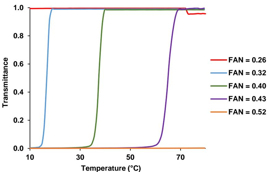
**Figure S4.** Turbidity curves (first cooling) of P(AAm-co-AN) copolymers with various AN fractions ( $F_{AN}$ ) at 1 wt% in water.
