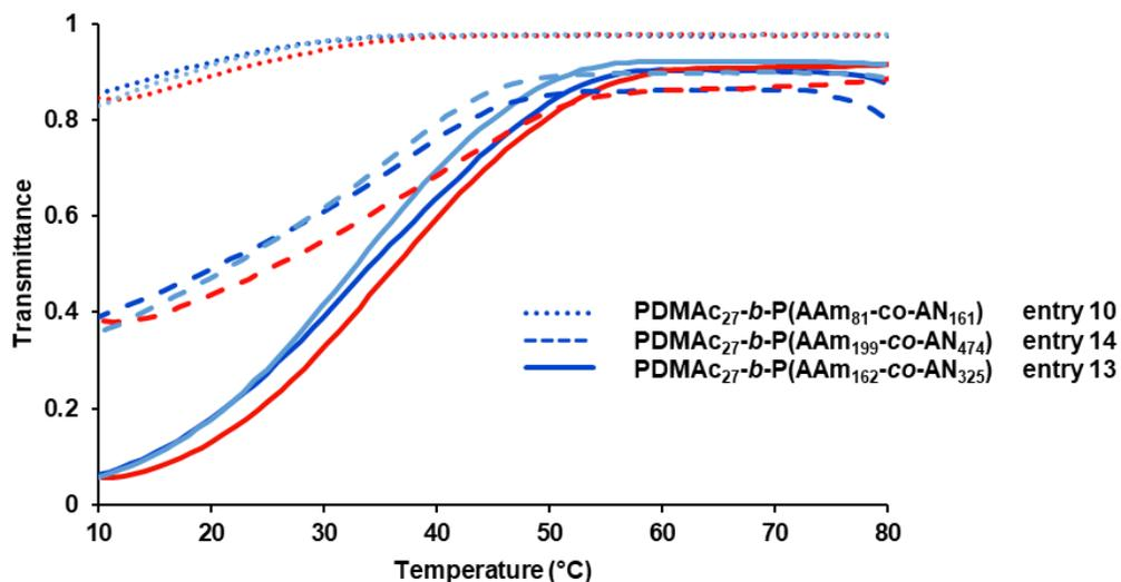
**Figure S14.** Turbidity curves of PDMAc-*b*-P(AAm-*co*-AN) dispersions at 1 wt% (entries 10, 13 and 14 in Table 3). First and second cooling in dark and light blue, second heating in red.
