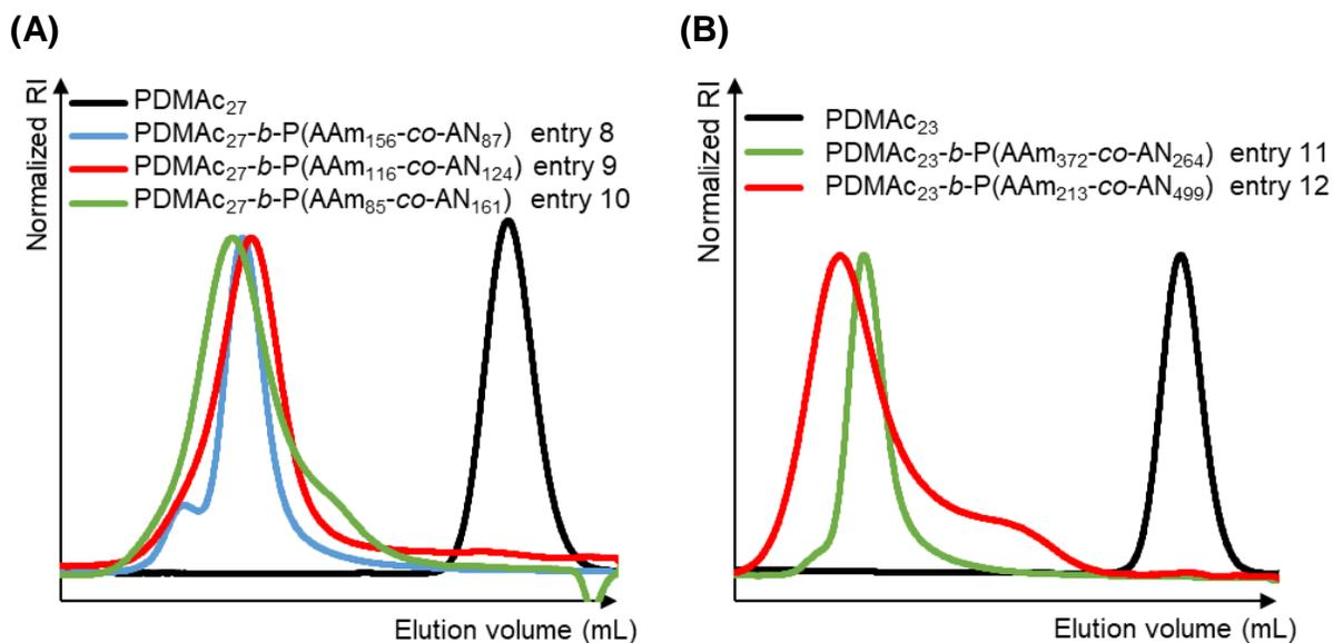
**Figure S7.** Normalized size exclusion chromatograms of PDMAc macroRAFT agents and the resulting PDMAc-*b*-P(AAm-*co*-AN) block copolymers prepared by copolymerization of AAm and AN in water at  $45\text{ }^\circ\text{C}$  targeting (A) a DP = 250 and (B) a DP = 800, and various AN contents (Table 1).
