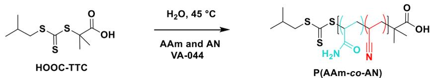
**Scheme S1.** Synthesis routes for the statistical P(AAm-co-AN) copolymers *via* aqueous RAFT polymerization.
