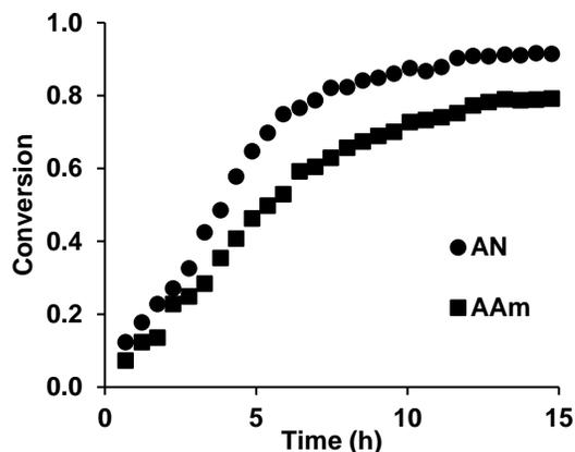
**Figure S6.** Monomer conversions monitored by  $^1\text{H}$  NMR in  $\text{D}_2\text{O}$ . Polymerization performed with  $f_{\text{AN},0} = 0.44$  using an initial molar ratio of monomers/macroRAFT/initiator of 800/1/0.3 and VA-044 as initiator at  $45\text{ }^\circ\text{C}$ .
