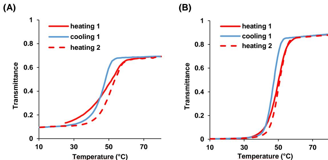
**Figure S5.** Turbidity curves (first heating, first cooling and second heating) of a P(AAm-co-AN) dispersion at (A) 0.2 wt% and (B) 1 wt% for copolymer obtained by FRP containing 32 mol% of AN (Table S1, Entry 7).
