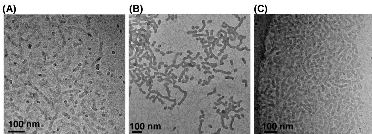
**Figure S13.** (A) Representative cryo-TEM image of sample 13, PDMAc-*b*-P(AAm-*co*-AN) with a  $DP_n$  (P(AAm-*co*-AN)) = 510 prepared at 1 wt% (the dark spots are surface contaminations stemming from water crystals on the sample surface); (B) TEM and (C) cryo-TEM images of sample 14 with  $DP_n$  (P(AAm-*co*-AN)) = 760 prepared at 0.03 wt% (TEM) and at 0.3 wt% (cryo-TEM), respectively.
