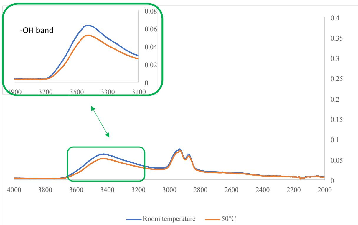
Figure S 20 : FTIR analysis of PIMA in function of temperature.
