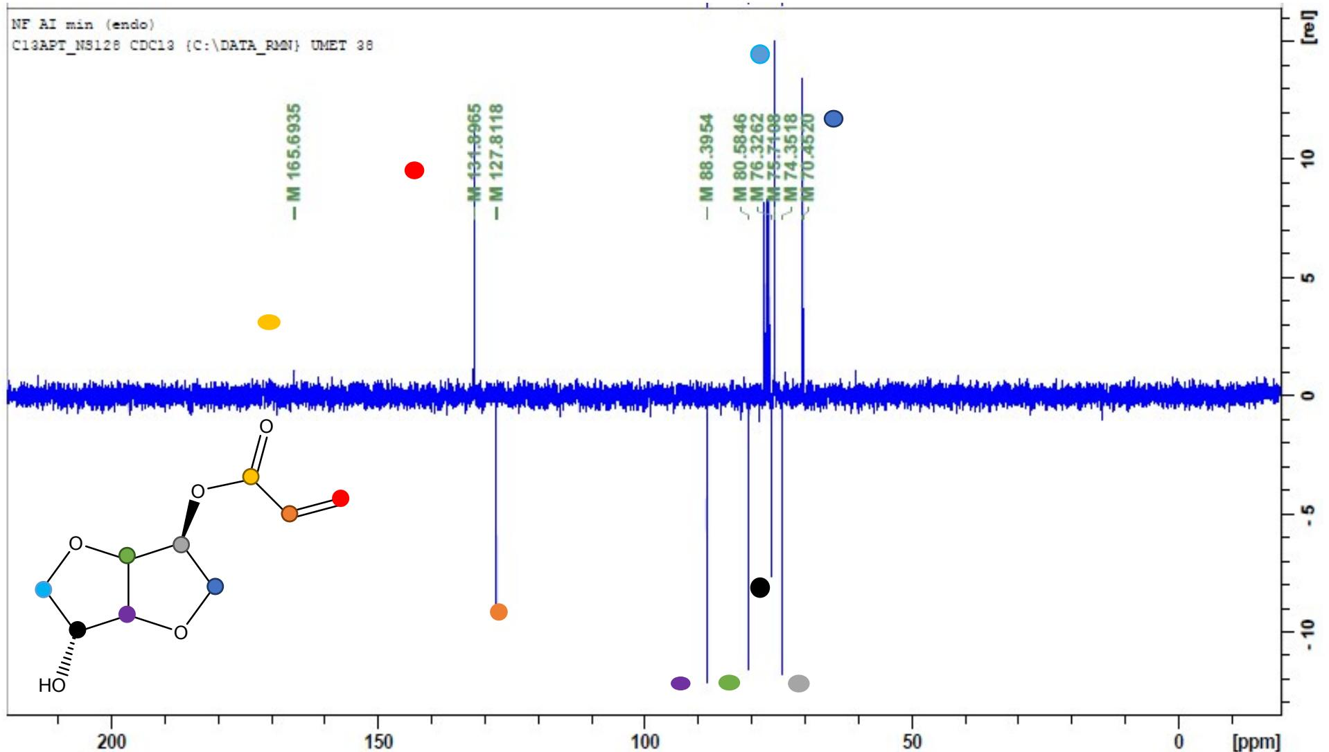
Figure S 2 : NMR <sup>13</sup>C Jmod, CDCl<sub>3</sub> of IMA endo
