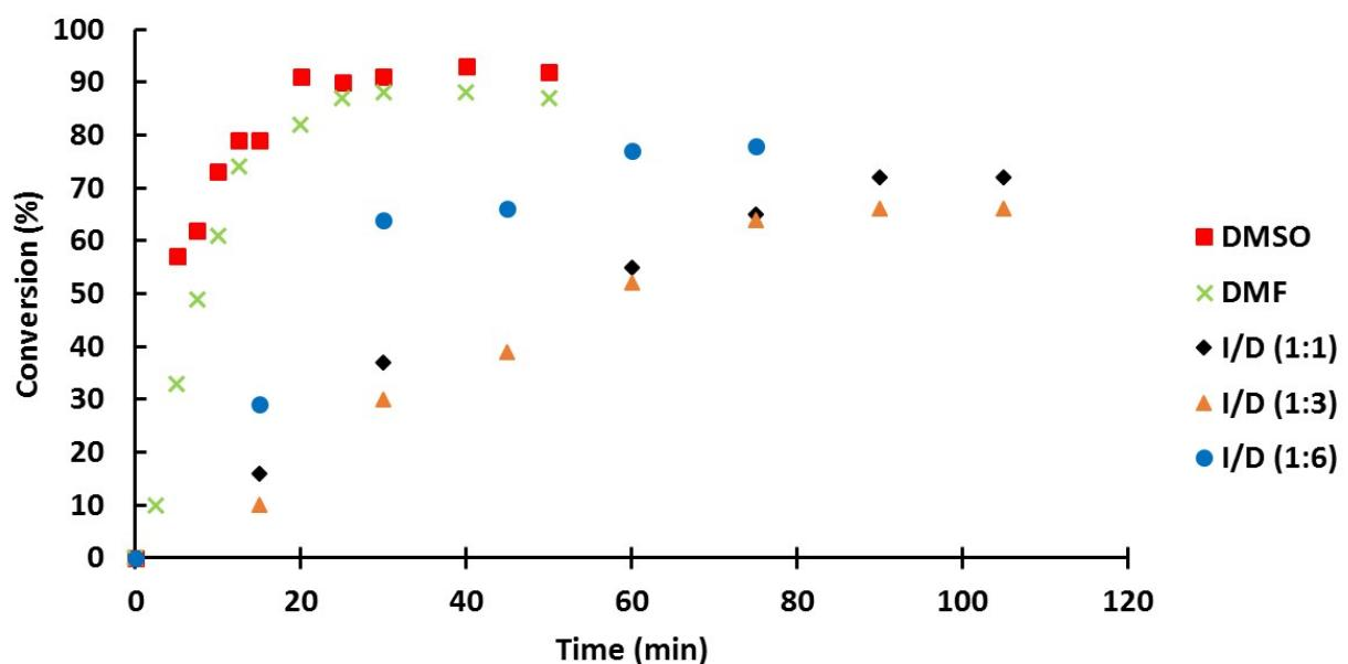
Figure S 5: Evolution of IMA conversion in different solvents ( $[IMA]/[AIBN] = 100$ ) at  $90\text{ }^{\circ}\text{C}$
