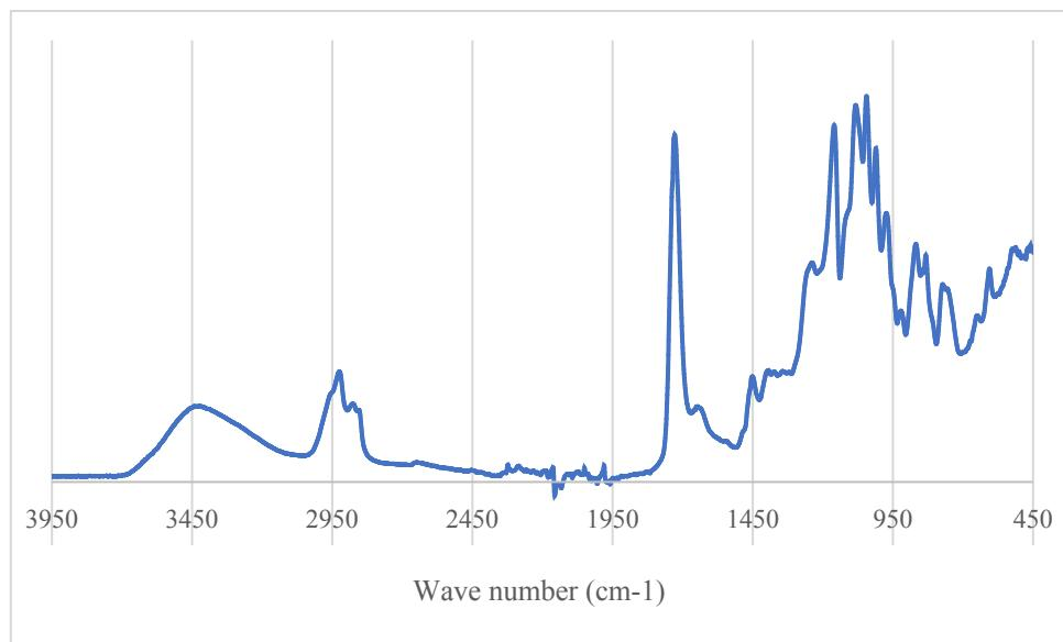
Figure S 23 : FTIR analysis of PIMA thermoset (10% crosslinker)
