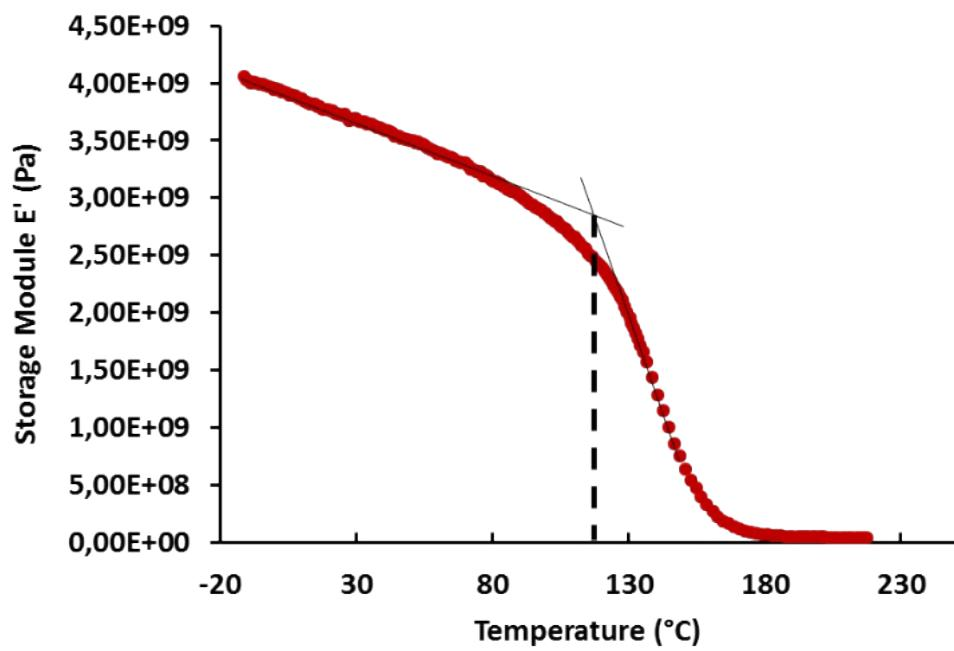
Figure S 22 : DMA analysis of PIMA thermoset (10% crosslinker)
