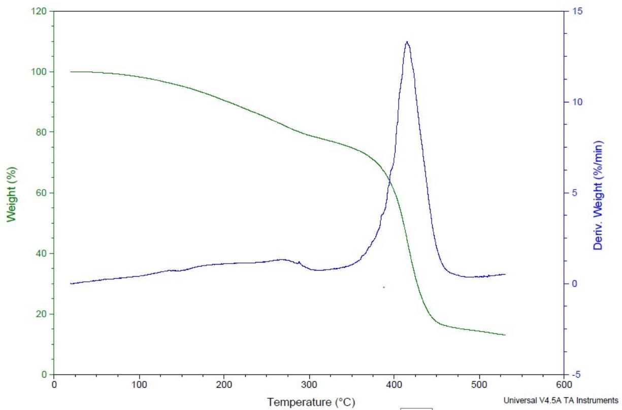
Figure S 24 : TGA thermogram of PIMA thermoset (10% crosslinker)
