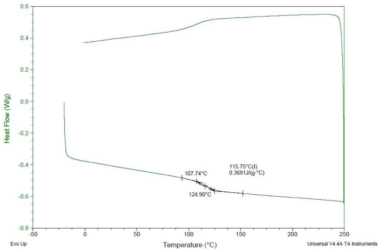
Figure S 21 : DSC thermogram of PIMA thermoset (10% crosslinker)
