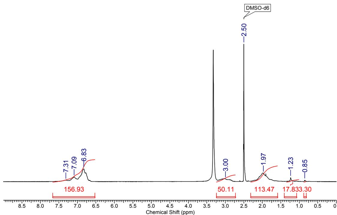
**Figure S29.**  $^1\text{H}$  NMR (400 MHz,  $\text{DMSO-}d_6$ ) spectrum of poly(1VIM) and PNVP after purification by precipitation in diethyl ether and following dialysis. *The PNVP block is not visible in the spectrum, which indicates the PNVP was not successfully coupled with poly(1VIM).*
