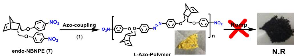
Scheme 6. The other synthetic route for Porous polynorbornene with azobenzene subunit.
