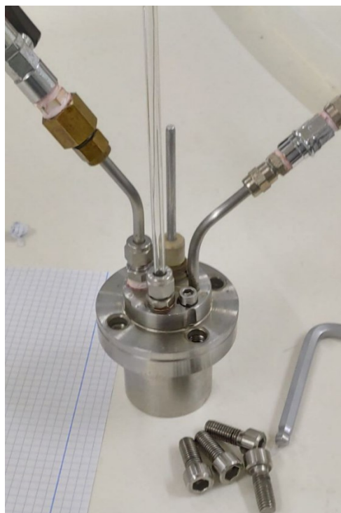
Fig. S19. The SS304 reactor used for e ATRP of vinyl chloride at the Department of Chemical Engineering of University of Coimbra.
