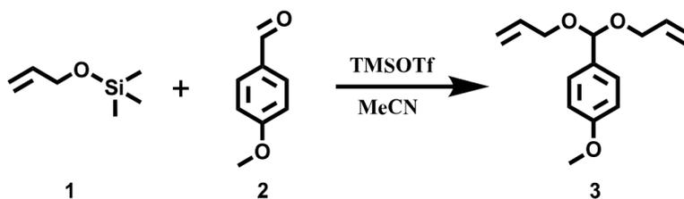
**Scheme S1.** Synthesis of bis-allyl 4-methoxybenzylidene acetal (BAMA, **3**)
