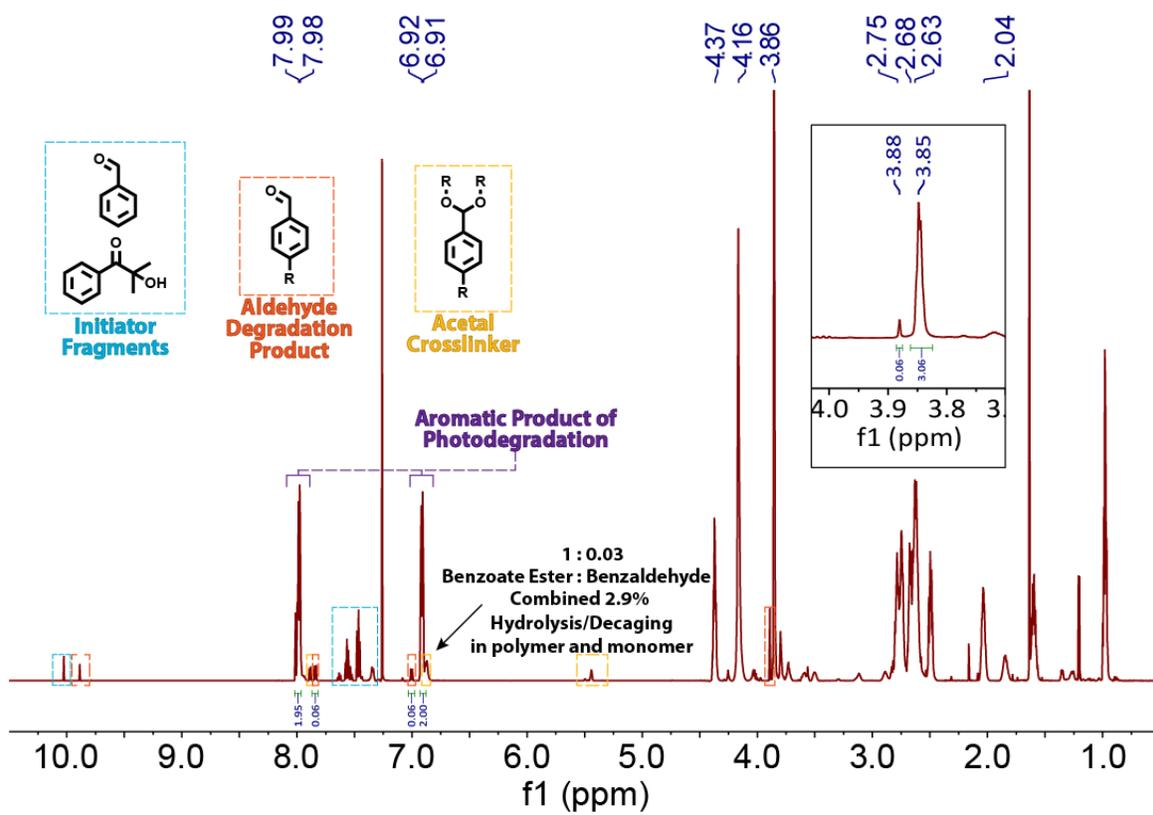
**Fig. S1.** NMR of crude photodegradation products to show lack of competing hydrolysis/decaging reactions. The areas integrated represent only 4-methoxybenzoate ester and 4-methoxybenzaldehyde aromatic and methoxy shifts. Complete assignments and integrations listed in NMR data section.
