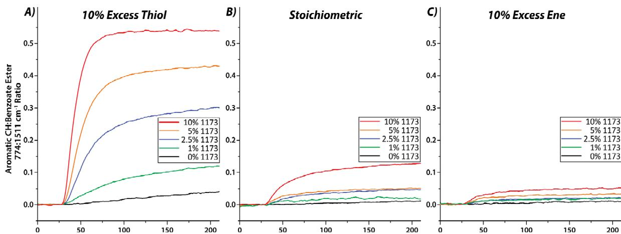
**Fig. S2.** Initiator concentration dependence of BAMA:PETMP network degradation at 200 mW cm<sup>-2</sup> irradiation.
