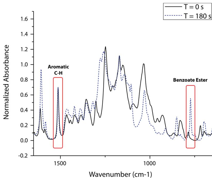
**Fig. S6.** Spectra of PETMP-acetal resin prior to irradiation (solid black) and after 180 s irradiation at 200 mW cm<sup>-2</sup> (dashed blue) cropped to the region of interest. As in figure S.2, the highlighted regions indicate the peaks tracked to obtain kinetic information.
