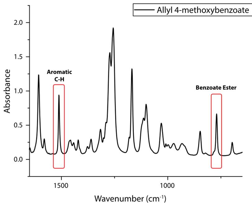
**Fig. S4.** FT-IR of allyl-methoxybenzoate control compound **6**. Benzoate ester peak at  $774\text{ cm}^{-1}$  corresponds to the same peak observed in the degradation process. The ratio of the highlighted benzoate ester peak to the highlight aromatic peak is used to quantify acetal  $\beta$ -scission to form benzoate esters.
