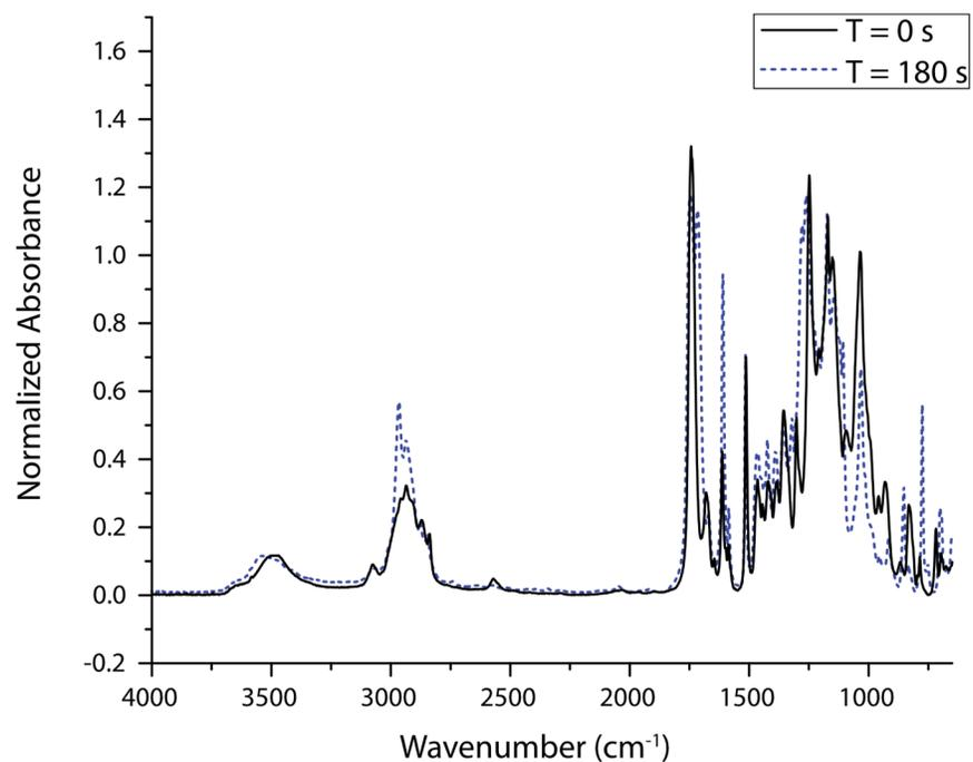
**Fig. S5.** PETMP-acetal resin prior to irradiation (solid black) and after 180 s irradiation at 200 mW cm<sup>-2</sup> (dashed blue).
